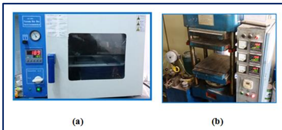
Figure (3-6) Equipment required for pressing specimens (a) Electric thermal oven and (b) Hydraulic thermal press.
