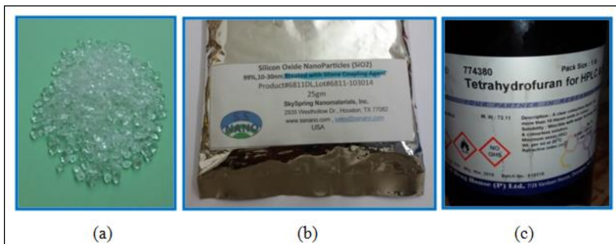
Figure (3-2) (a) PMMA granules, (b) Silicon oxide nanoparticles ( \text{SiO}_2 ) and (c) Tetrahydrofuran solvent.
