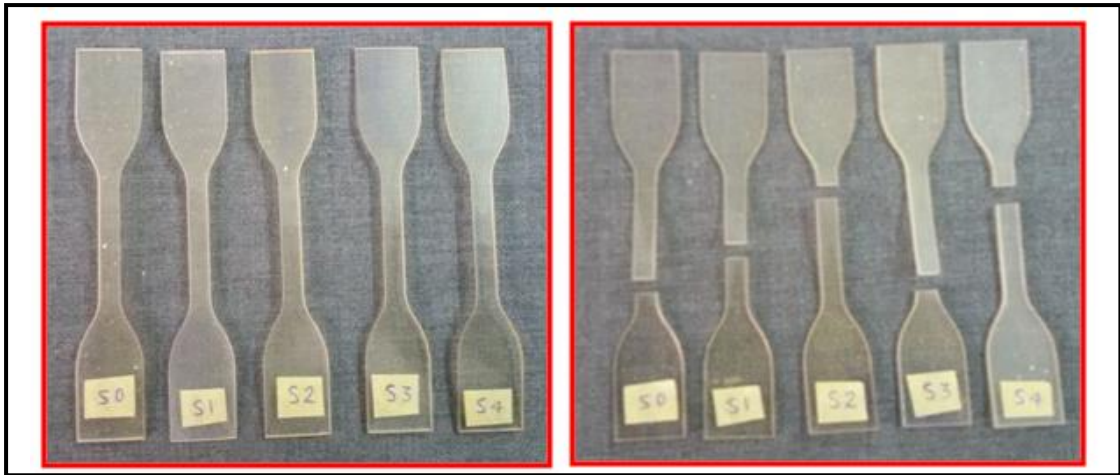
Figure (3.9) Specimens of tensile test before and after conducting the tensile tests.
