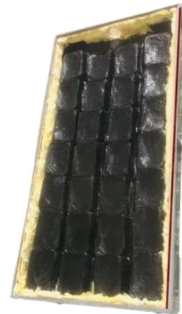
Facing downwards the Configuration is made of disposable aluminum bowls
