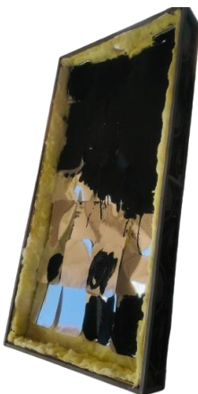
Figure (3-13) Painting the cover of insulation
