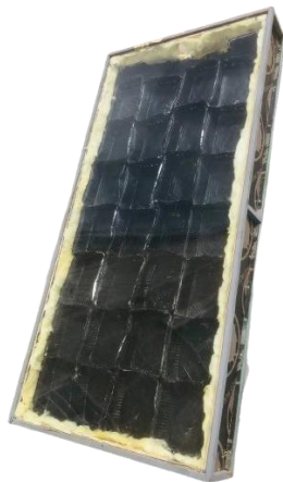
Facing upwards the Configuration is made of disposable aluminum bowls
