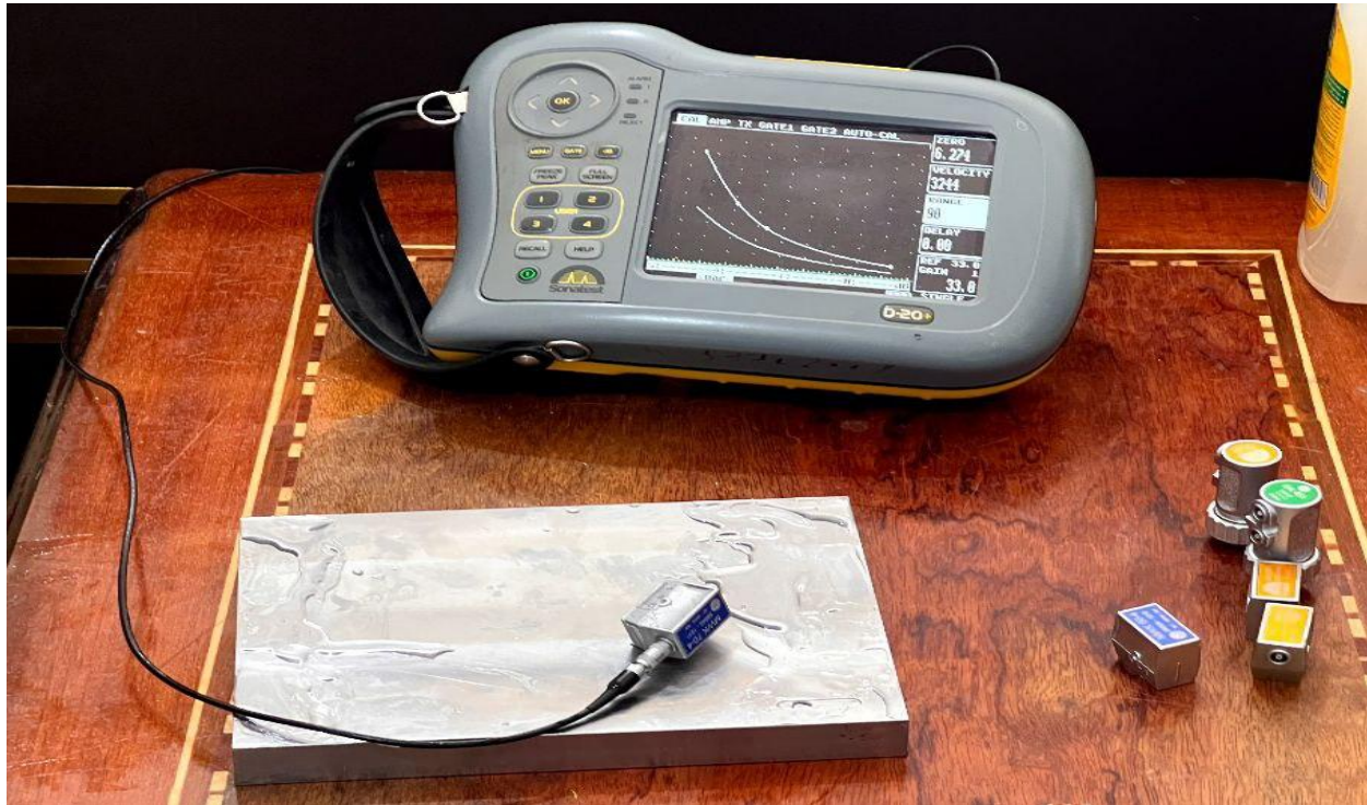
Fig.1 Sonatest Ultrasonic Flow detector D20+
