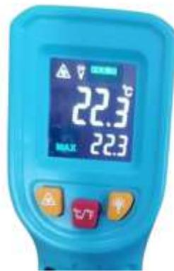
Figure (4.9): Infrared Thermometer Device
