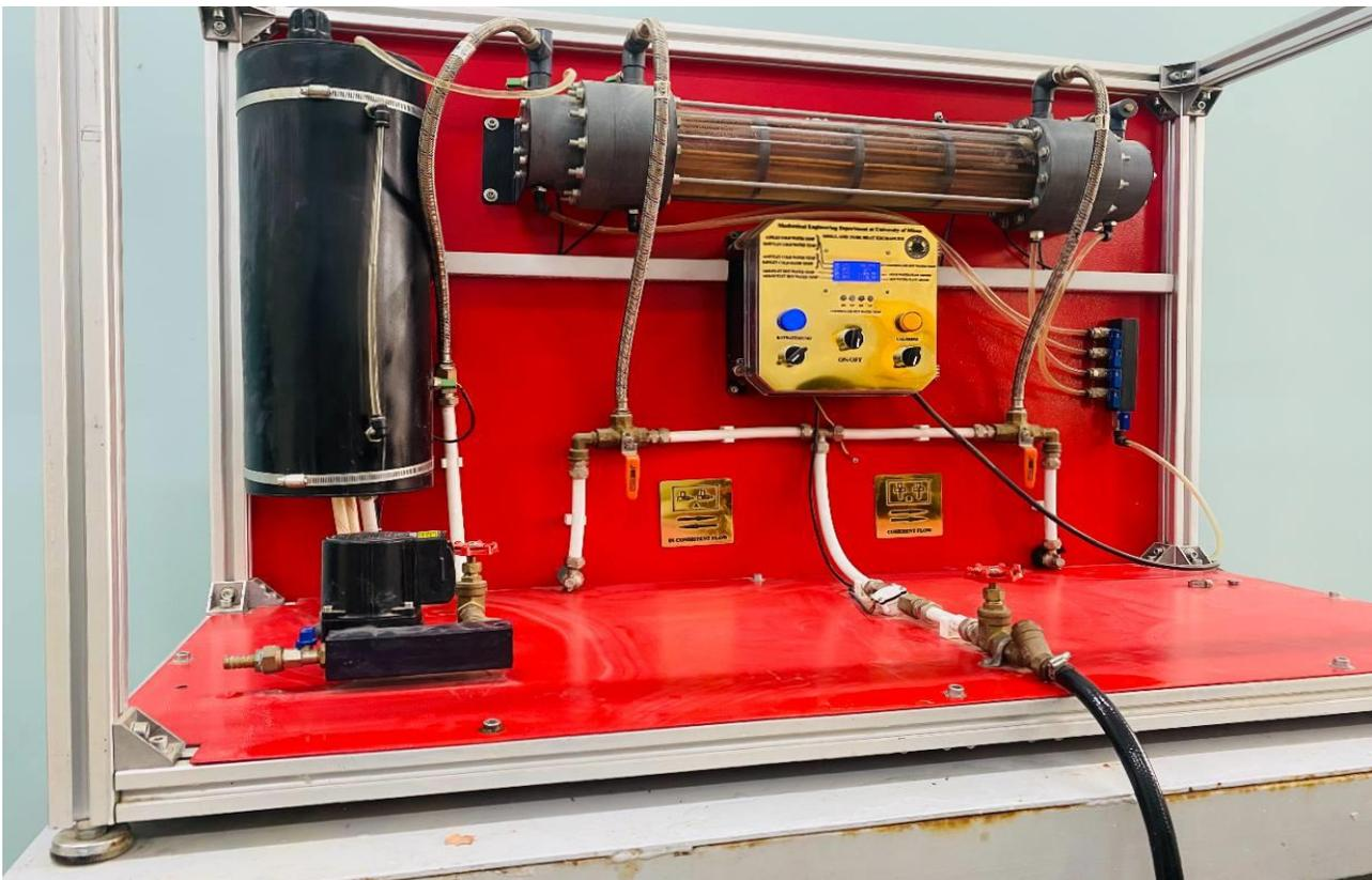
**Figure (3.1): Shell and tube heat exchanger.**
