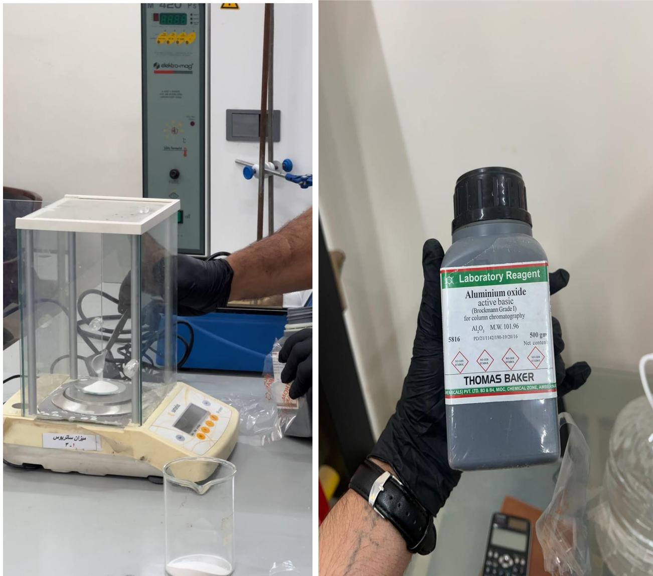
**Figure (4.3):** Weighting the Aluminum Oxide.
