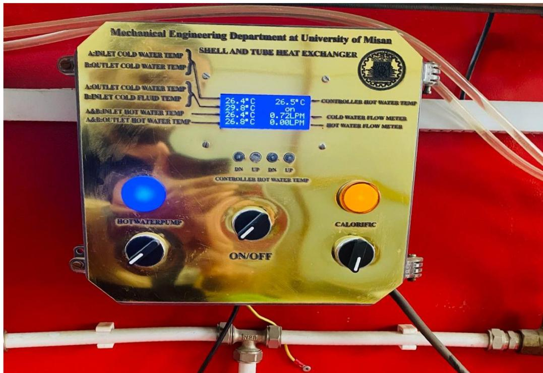
**Figure (3.5): Data logging device.**
