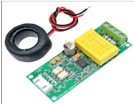
Figure (2.10): PZEM-004T sensor
