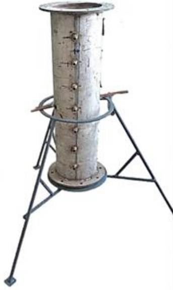
Figure 1: The schematic of the cylindrical storage packed bed used in the present study.
