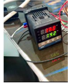
Figure 2 The electric heater (on the left) used to provide the desired inlet temperature. The temperature controller (on the right) used to control the outlet temperature from the heater.
