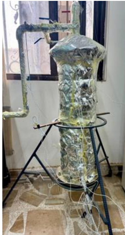
Figure 4: The storage vessel showing the external insulation used to reduce heat losses to the ambient.
