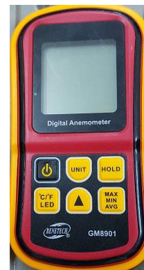
Figure 3: Air blower used to provide cold air to the storage system on the left. Digital Anemometer (on the right) used to measure the outlet velocity from the system
