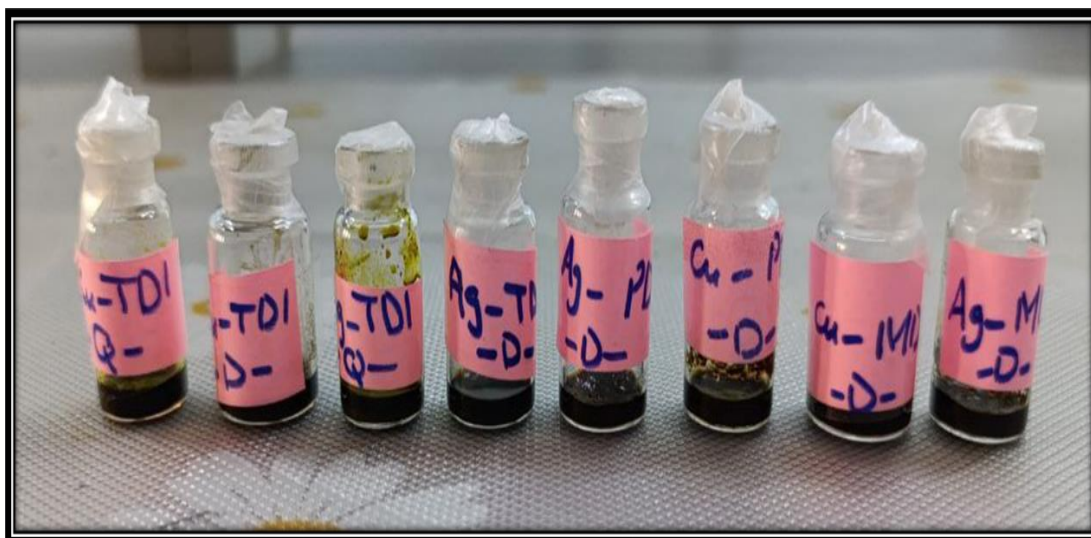
Figure (2-6): Laboratory photograph of conductive ink prepared by doping of polyurea polymers.
