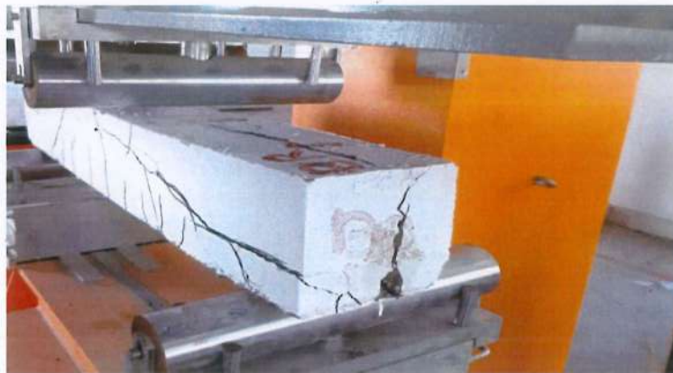
Figure 4.3 Slip Concrete Lower Layer in BR3 Beam.
