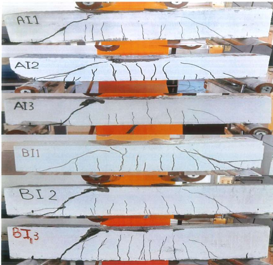
Figure 4.6 Crack Pattern of Beams with I-Shear Connector.
