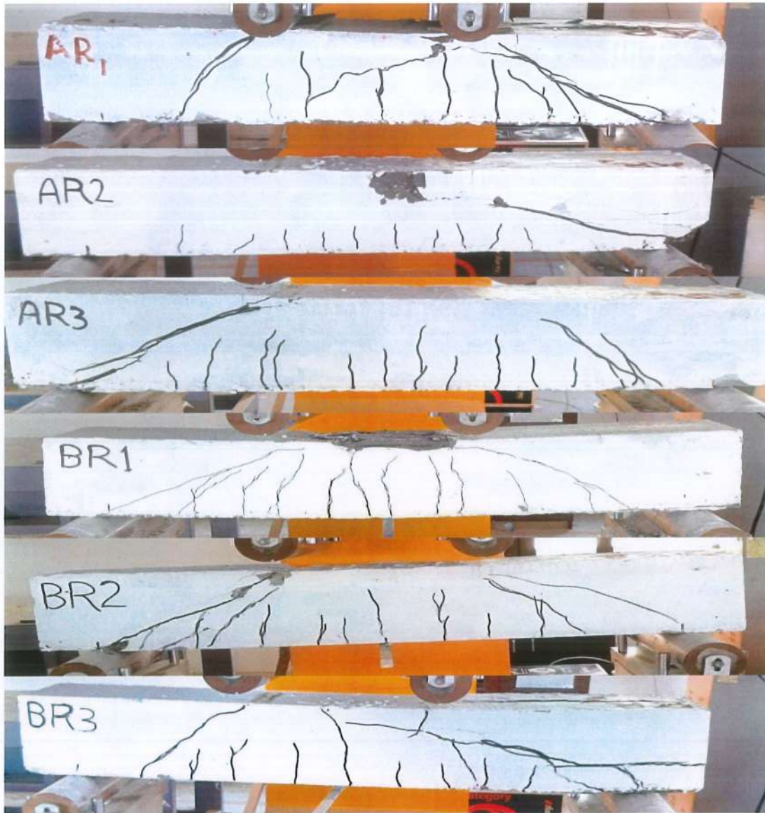
Figure 4.4 Crack Pattern of Beams with Rectangle Shear Connector.
