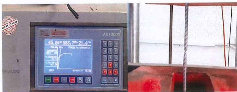
Figure 3.3 Reinforcement Test Bars' Tensile Strength.
