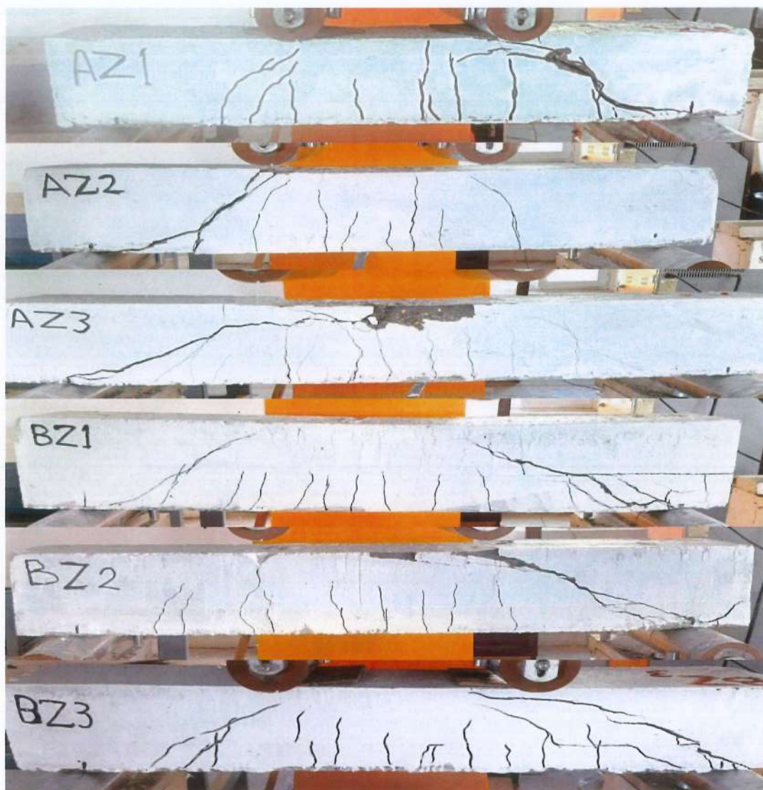
Figure 4.9 Crack Pattern of Beams with Z-Shear Connector.
