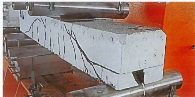
Figure 4.7 Slip Concrete Layer in BI1 Beam.
