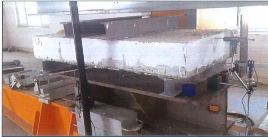
Figure 3.37 Loading and Support System for Panels Test.
