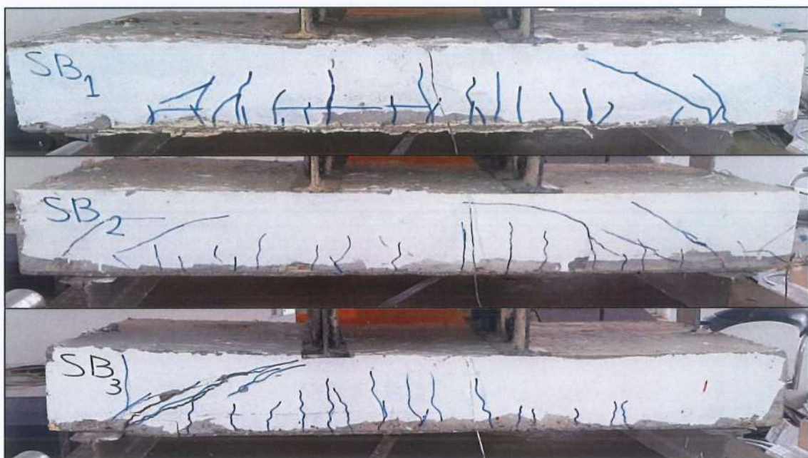
(b) Crack Pattern of SB Series
