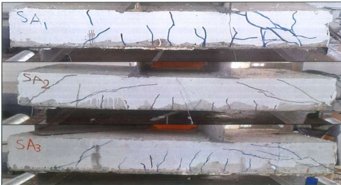
(a) Crack Pattern of SA Series.
