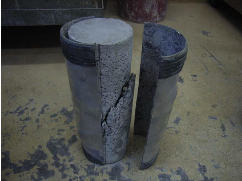
Figure 2.3 Failure Mode of Column Specimen [6].
