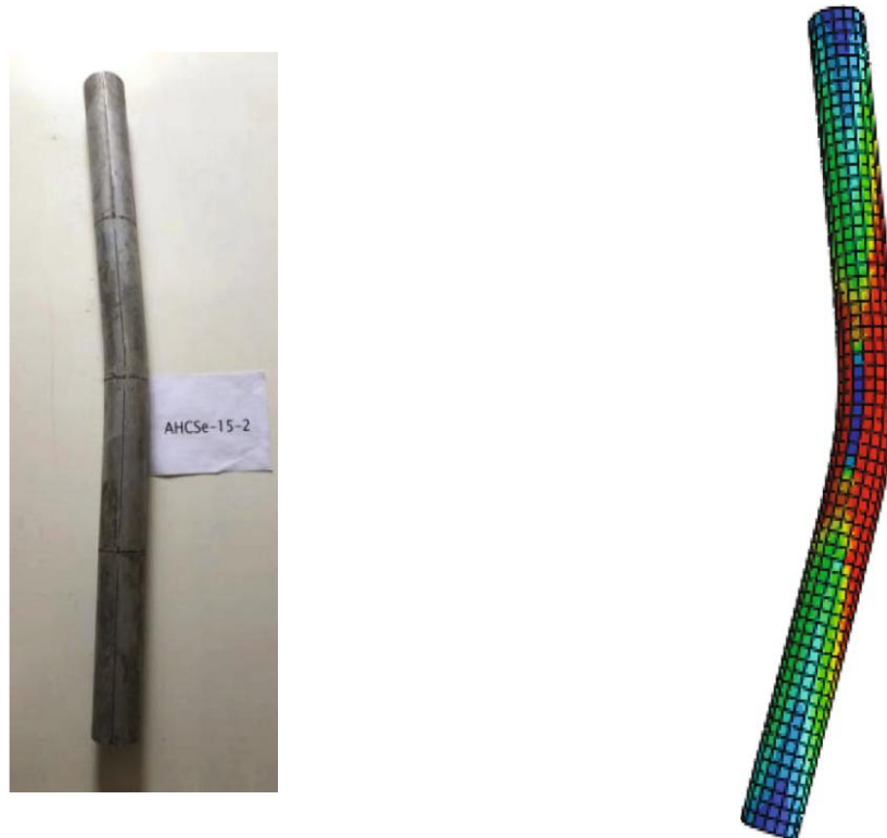
Figure 2.15 Numerical and Experimental Failure Mode [38].
