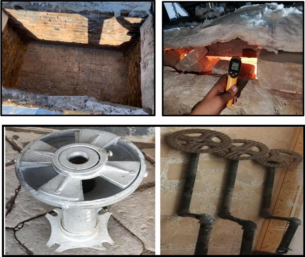
Figure 3.16: Firebricks for the oven, laser thermometer, and gas supply for the burners inside the oven.
