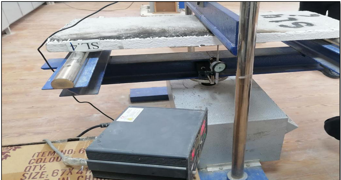
Figure 3.23: A Clip Illustrating the Loading and Mechanical LVDT Device.
