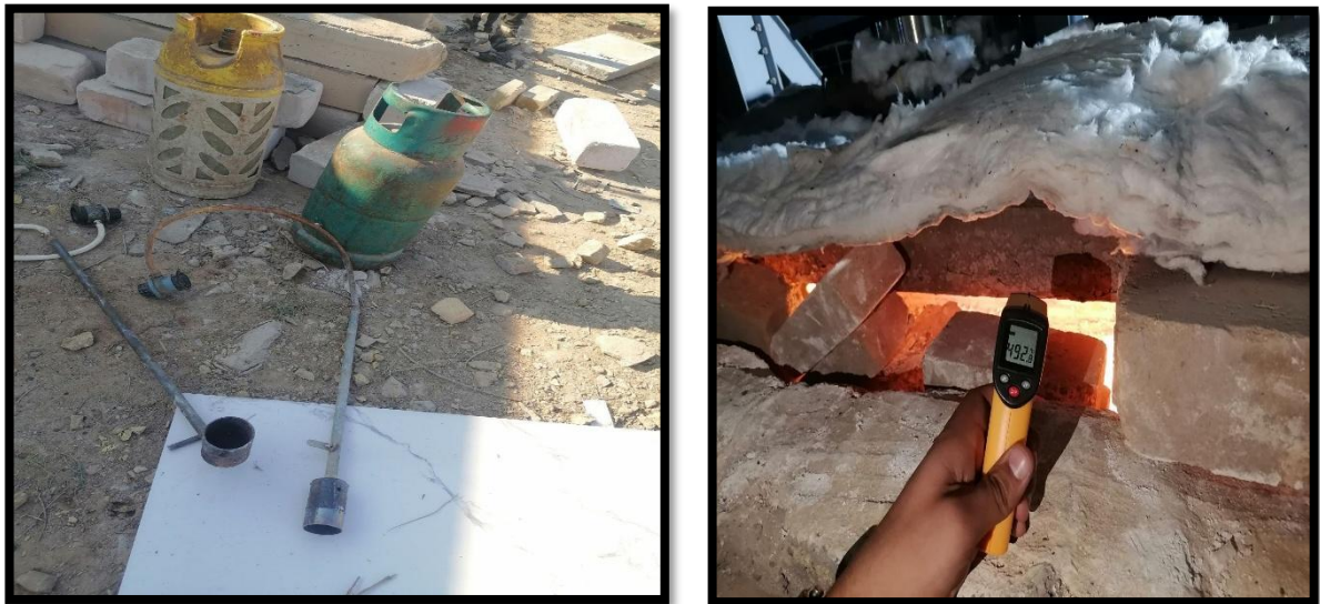
Figure 3. 21:a-Gaseous Heat Source b-Laser Thermometer
