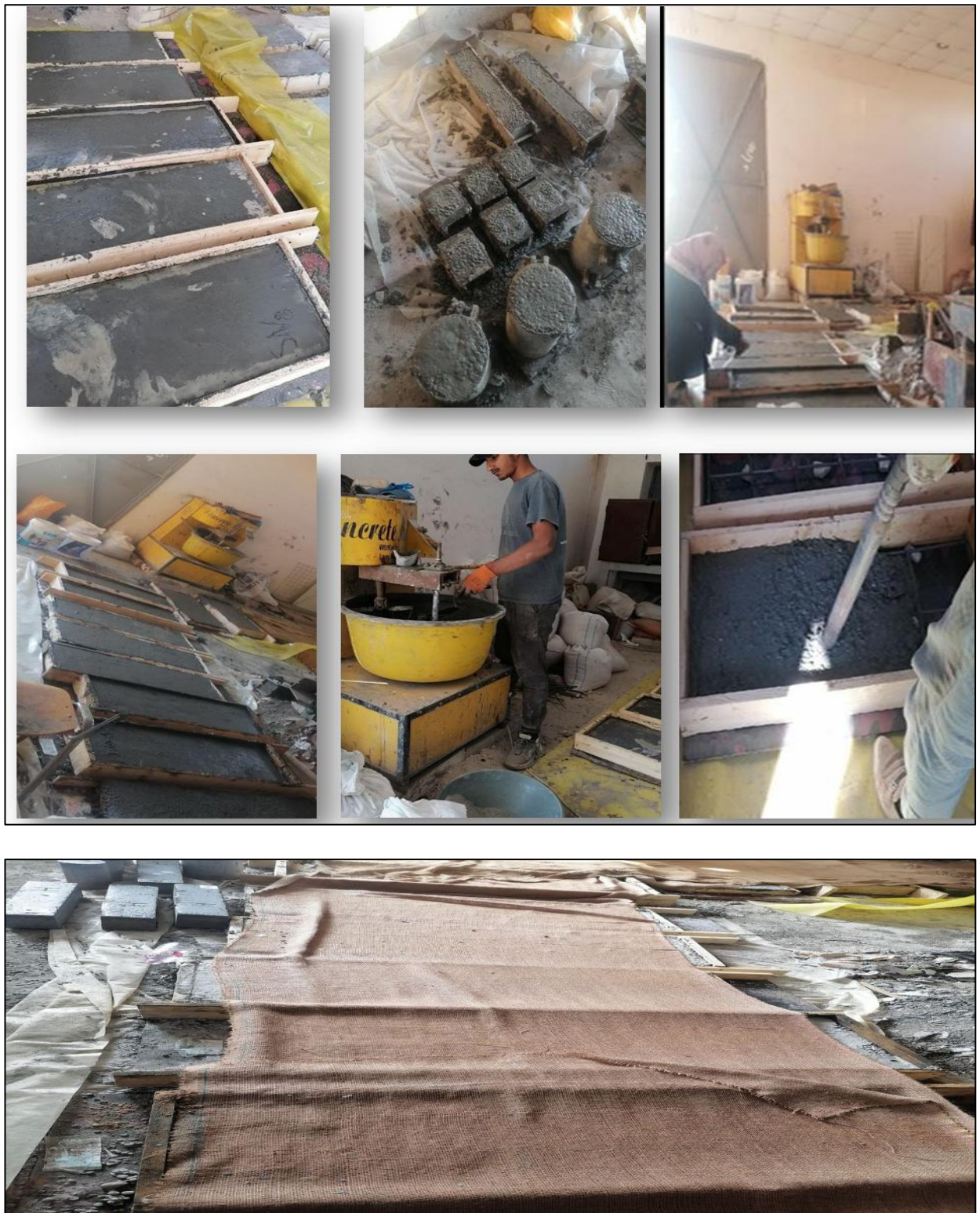
Figure 3.14 : Fabrication, Moulds, and Casting of the Specimens for Group 2.
