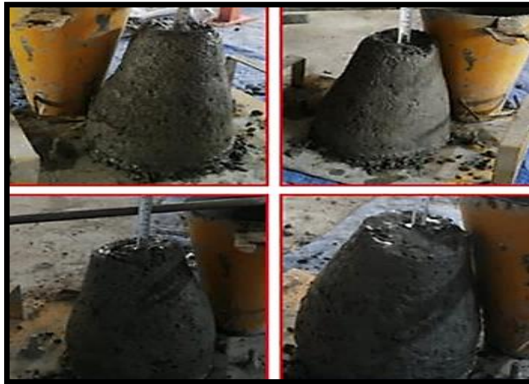
Figure 3.7 Slump Test of Fresh Concrete.
