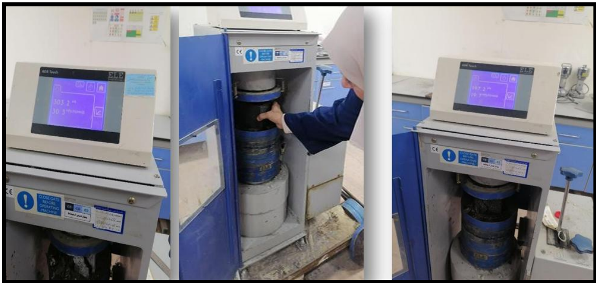
Figure 3.8 Compressive Test of Concrete.
