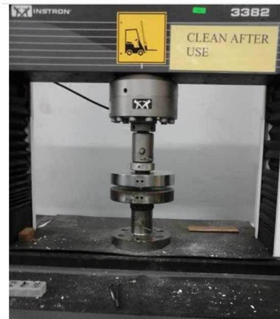
Figure 2.5: 2.5 T Universal Testing machine by INSTRON.
