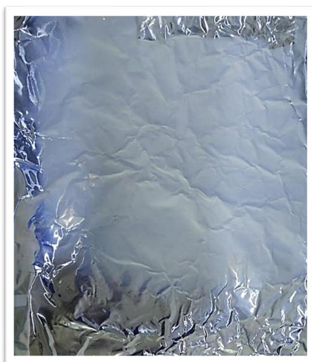
Figure (2-5) : Image for Deposition of Nylon 6,6 Electrospun Nanofibers on aluminum foil
