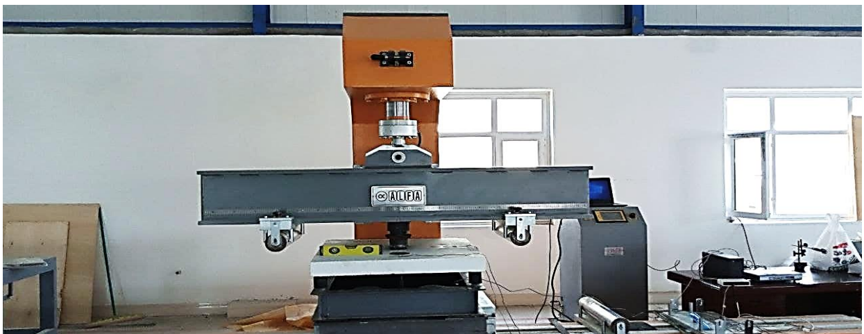
Figure 4.98 Concrete slabs containing D.S with fibers under concentrated load.
