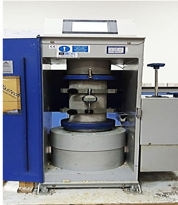
Figure 3.38 Modulus of elasticity test for cylindrical specimens.
