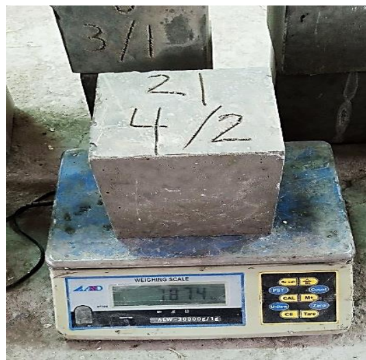
Figure 4.44 The dry density test for the concrete specimens (cubes).
