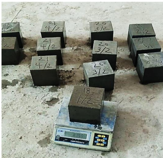
Figure 4.44 The dry density test for the concrete specimens (cubes).
