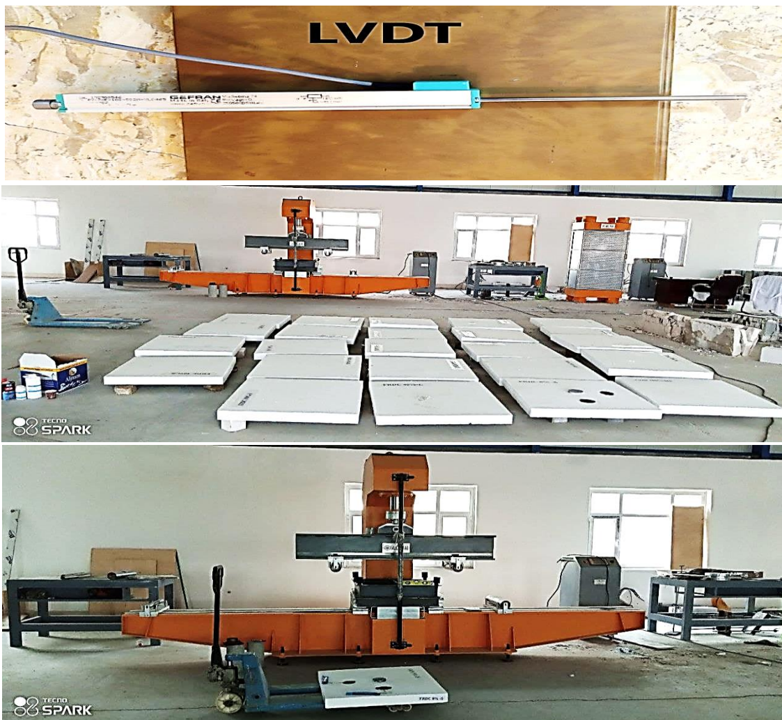
Figure 3.41 LVDT device with the electronic testing machine for concrete slabs.
