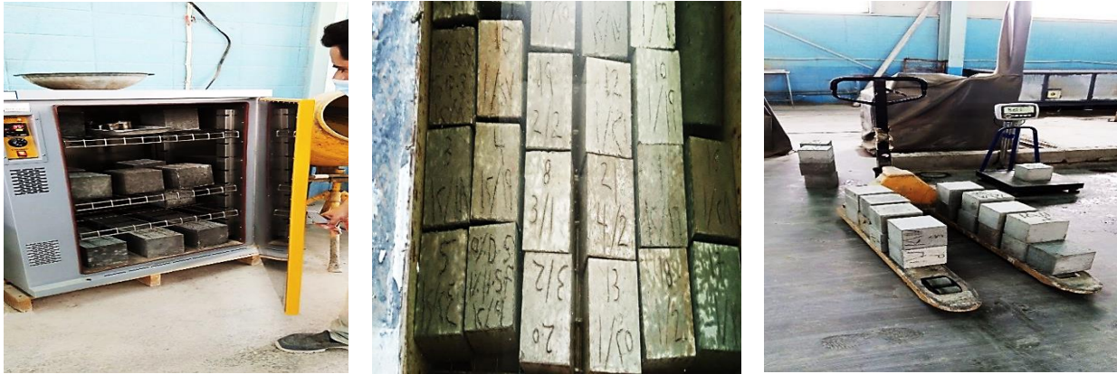
Figure 4.66 The water absorption test of the concrete specimens.
