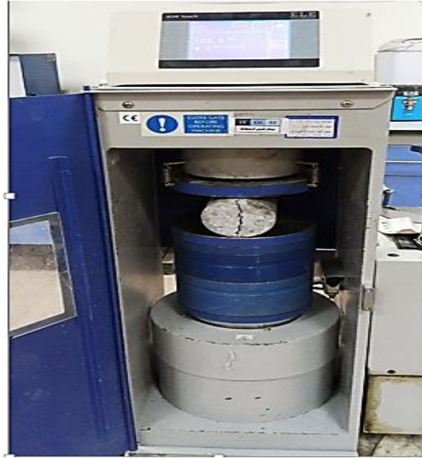
Figure 3.33 Splitting tensile test for concrete cylinders.
