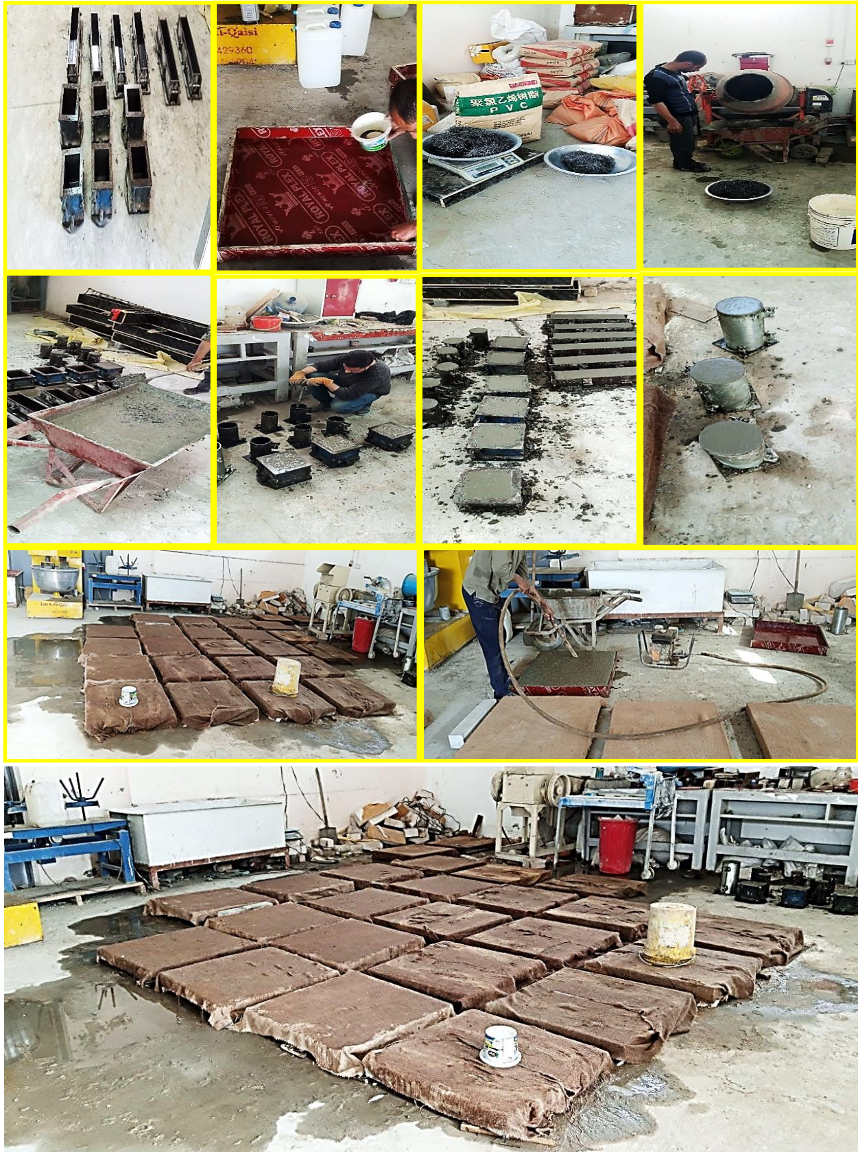
Figure 3.27 Lubrication of molds, casting concrete, and curing the slabs with water.
