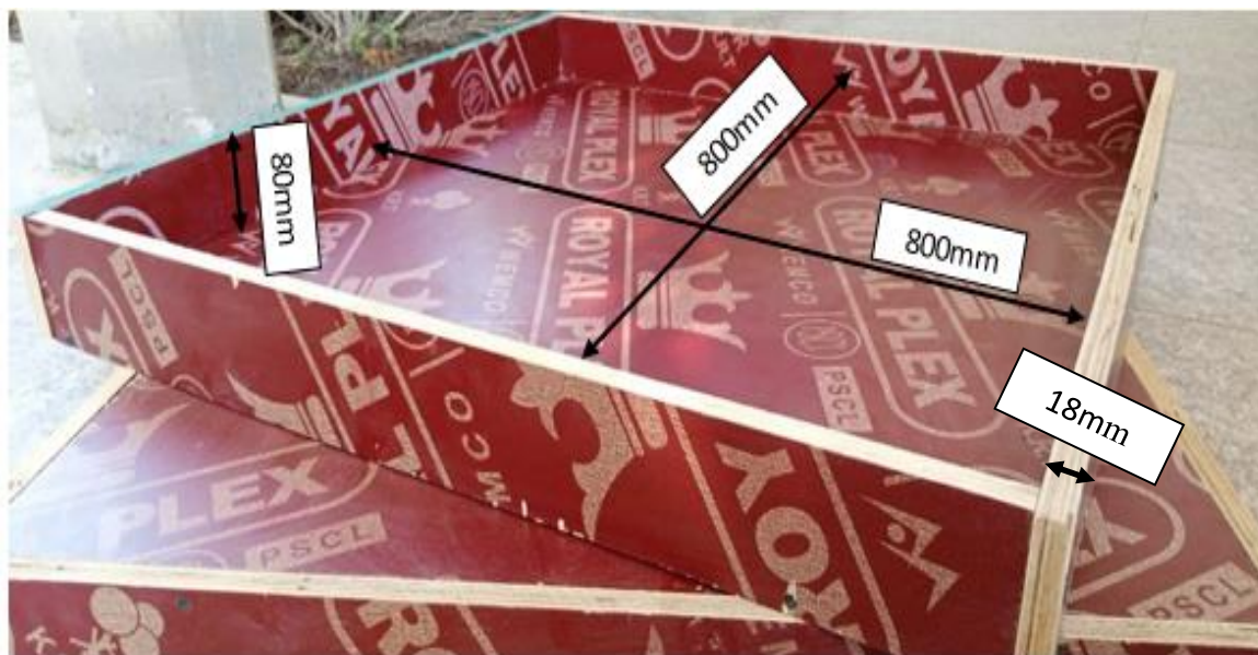
Figure 3.24 The internal dimensions of the wooden mold.
