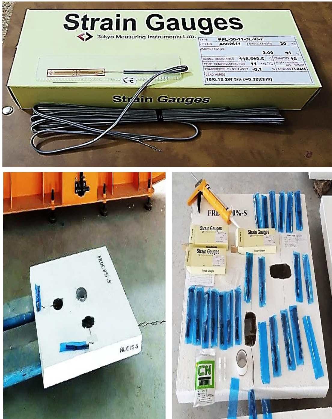
Figure 3.40 Paste strain gauges on the concrete slabs.
