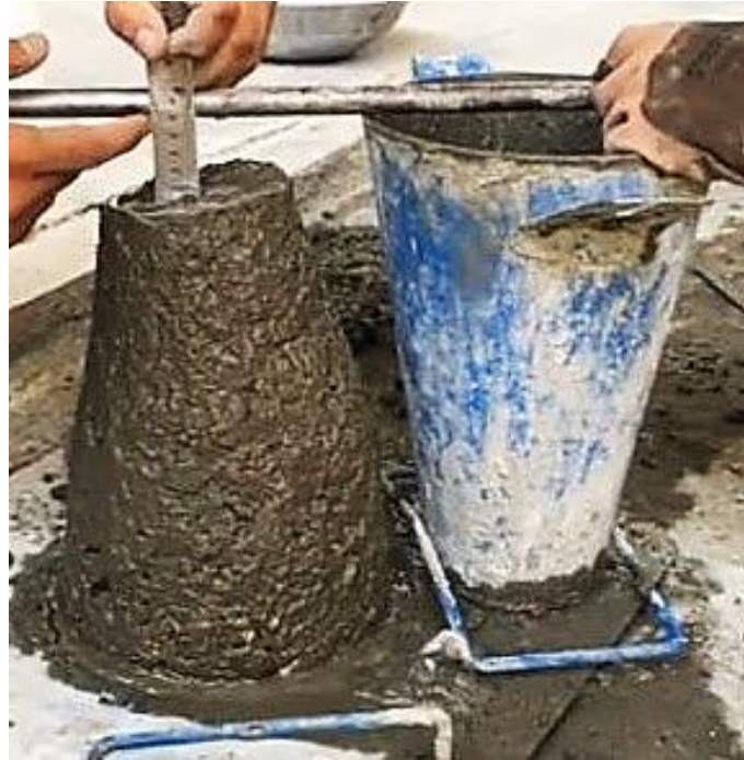
Figure 3.29 Slump test for concrete.
