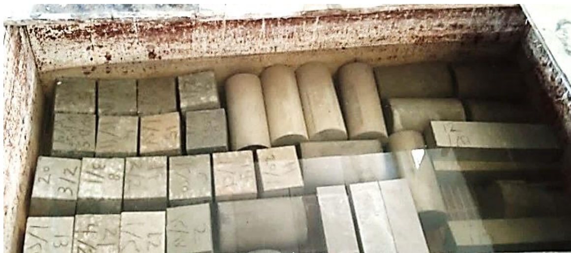
Figure 3.8 Curing concrete models with pure water.
