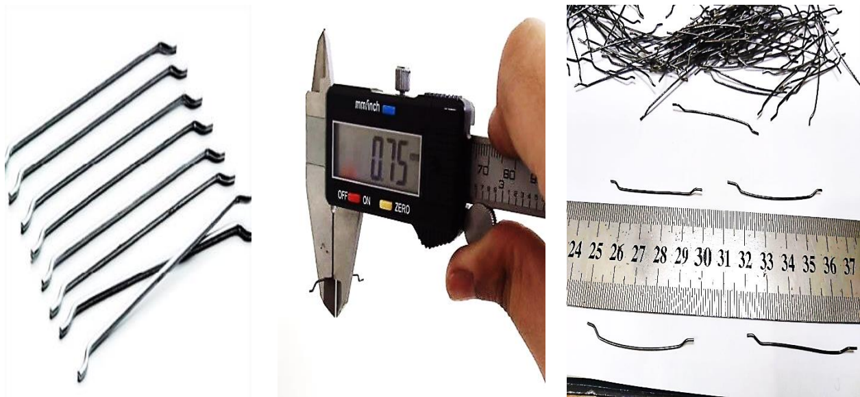
Figure 3.7 The shape of the macro steel fiber (hooked-end).
