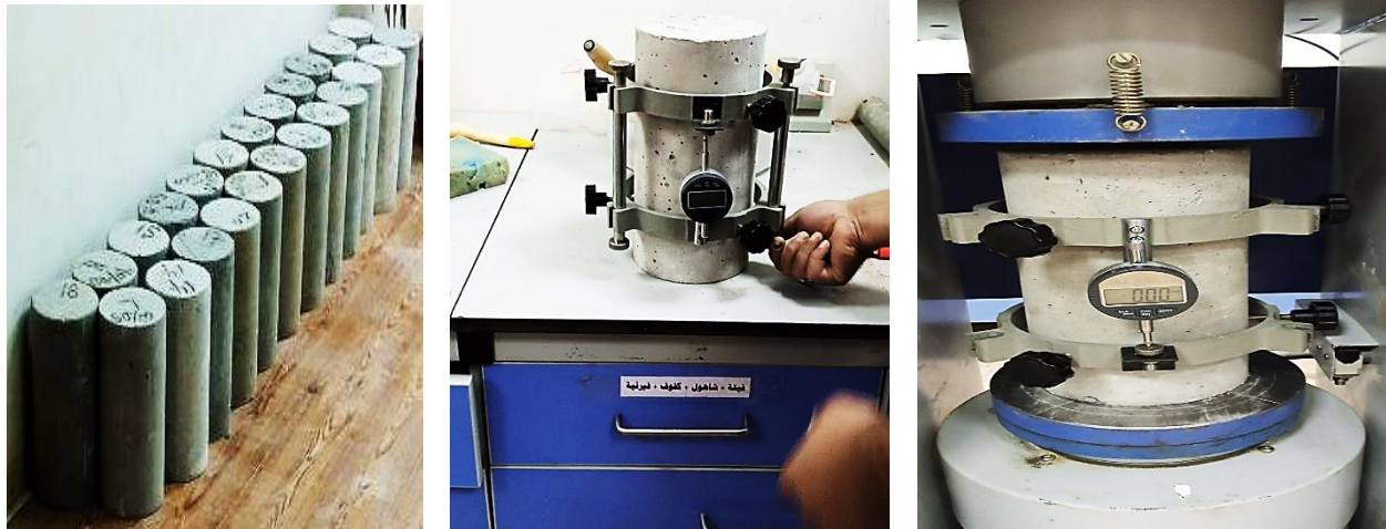
Figure 4.77 The static elastic modulus test of the concrete specimens (cylinders).
