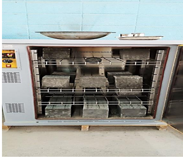
Figure 3.36 Water absorption test of concrete cubes specimens.
