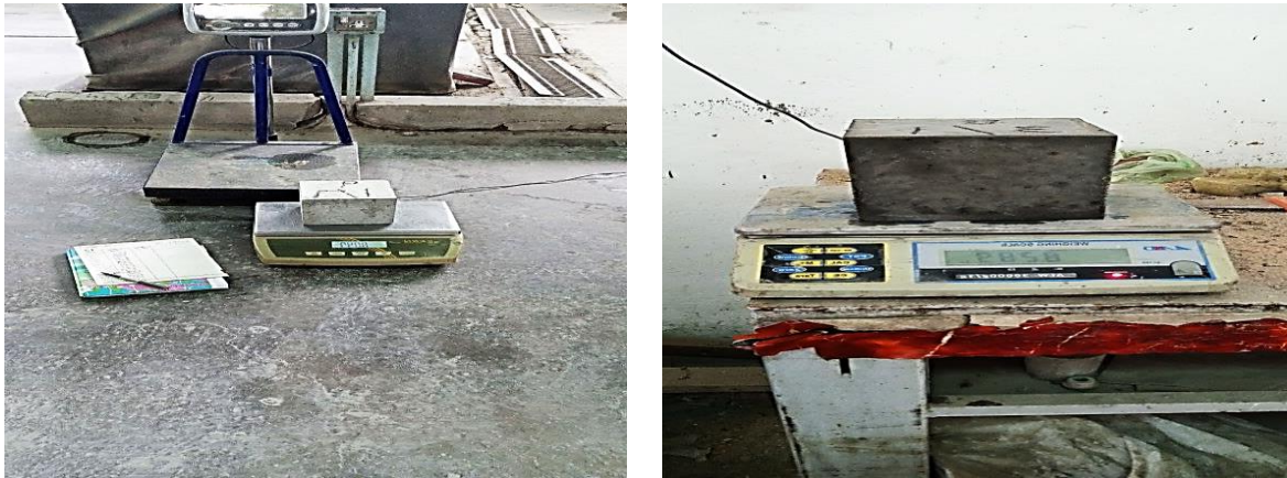
Figure 3.35 Dry density test of the concrete cubes.
