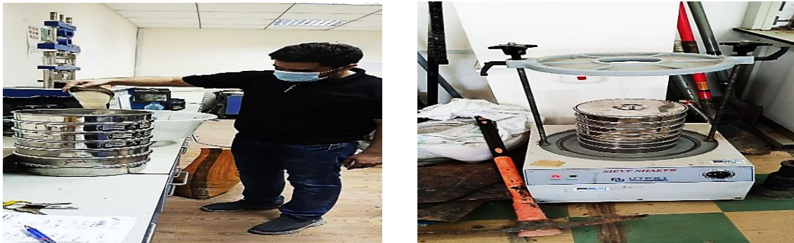
Figure 3.11 Gradation test for sand dunes in a laboratory.
