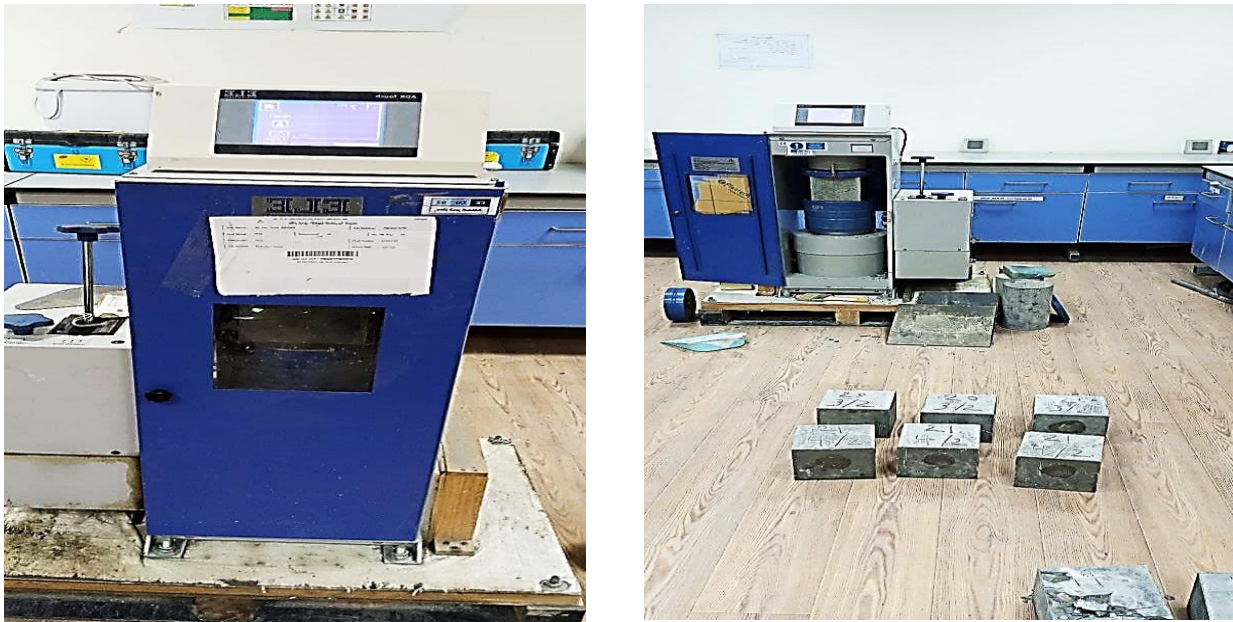
Figure 3.30 Compression testing machine for concrete cubes.
