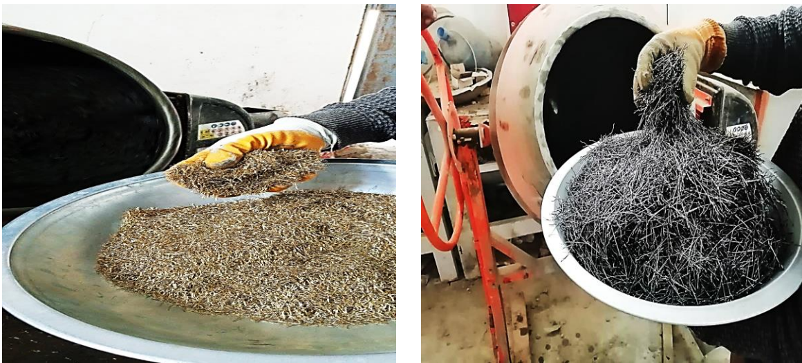
Figure 3.26 Manually adding fibers to the mixer.
