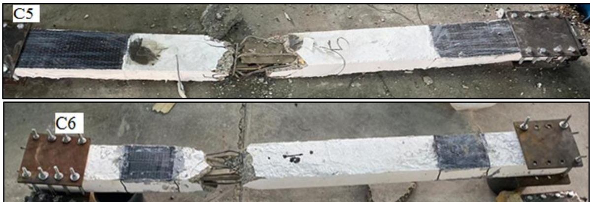
Fig. 4.11 Failure mode of second group (after testing).
