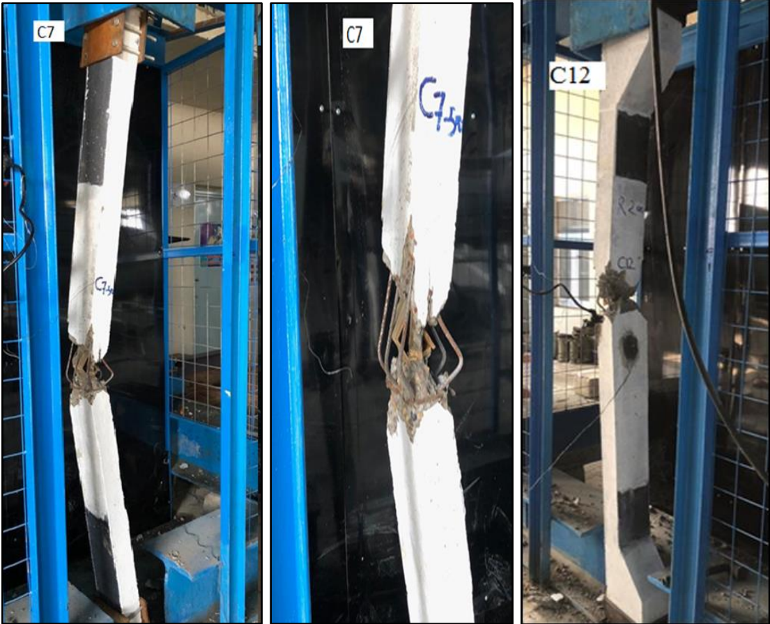
Fig. 4.28 Mode failure of sixth group (during the test).
