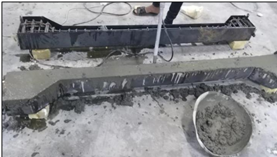
Fig. 3.21 using the vibrator during casting of column specimens.
