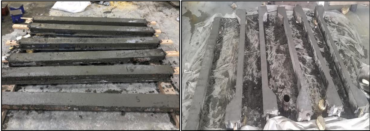
Fig. 3.22 Finishing casting of column specimens.
