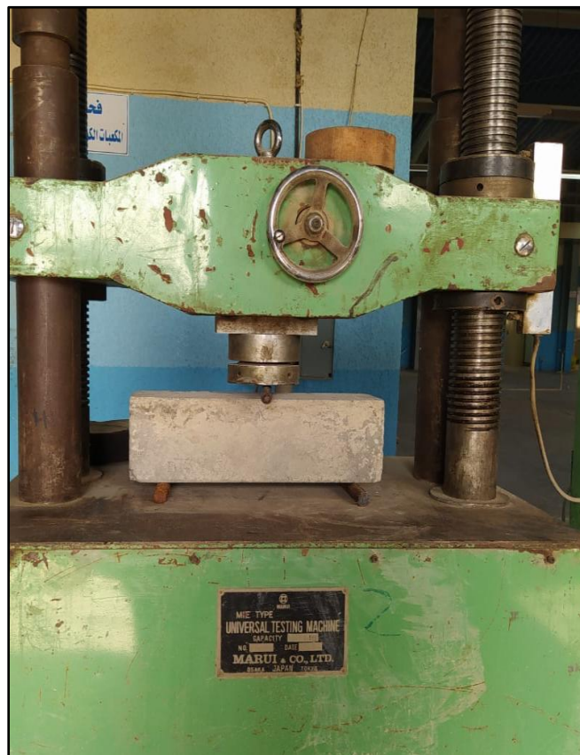
Fig. 3.27 Flexural strength test.
