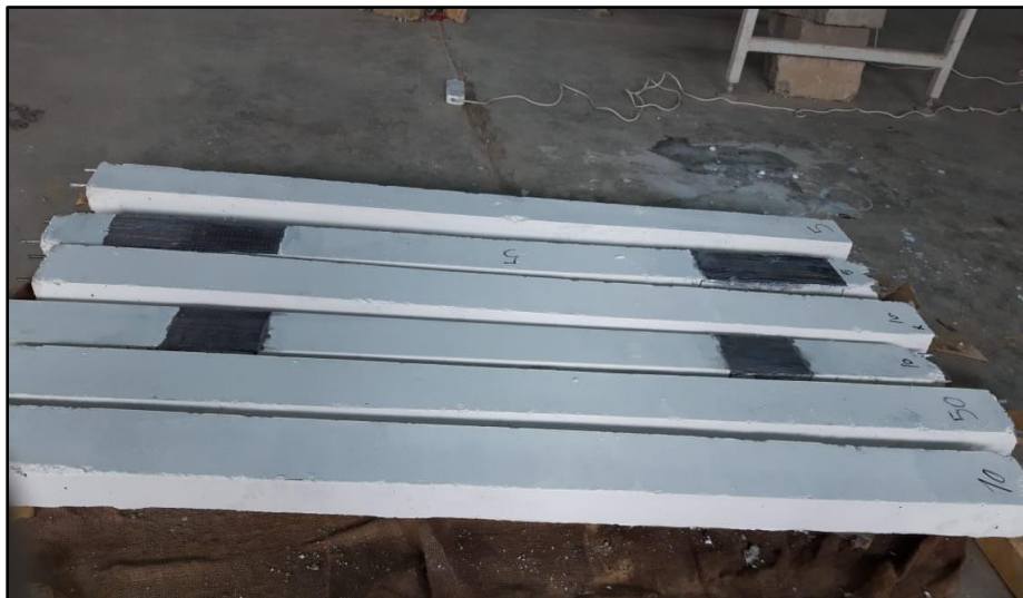
Fig. 3.24 Painting of the column specimens by white emulsion.
