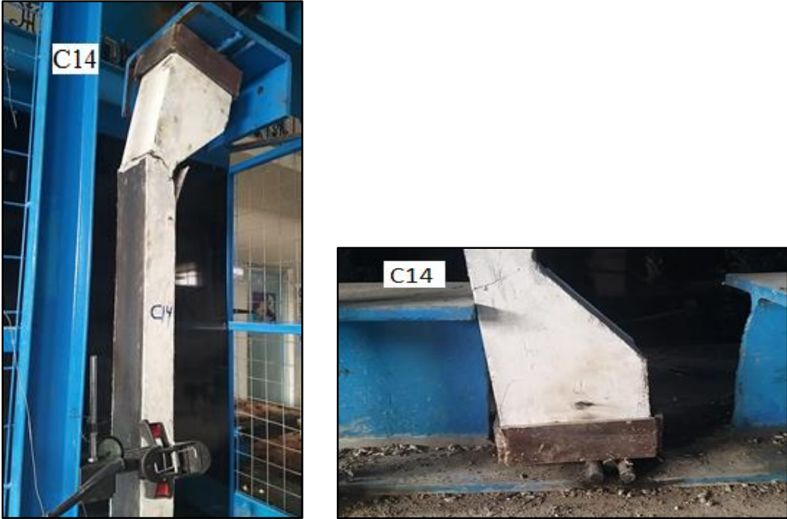
Fig. 4.35 Mode failure of column C14.
