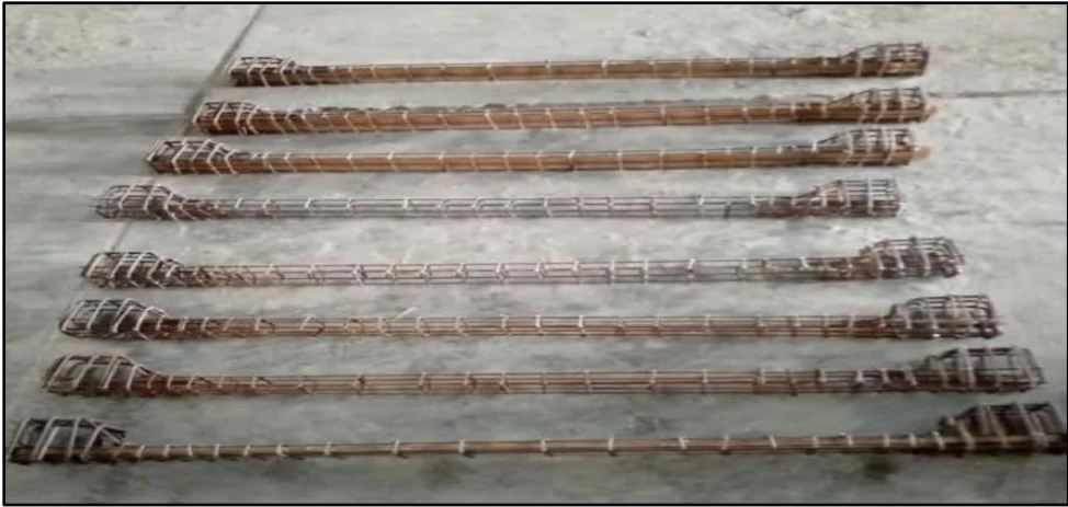
Fig. 3.15b Cage of steel reinforcement with corbels for columns (C8-C15).
