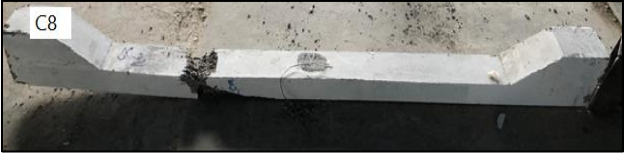
Fig. 4.15 Mode failure of columns during the test for third group.
