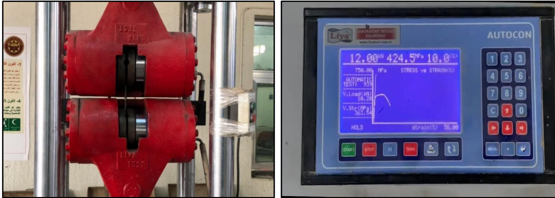
Fig. 3.3 Stress-Strain relationship for steel.
