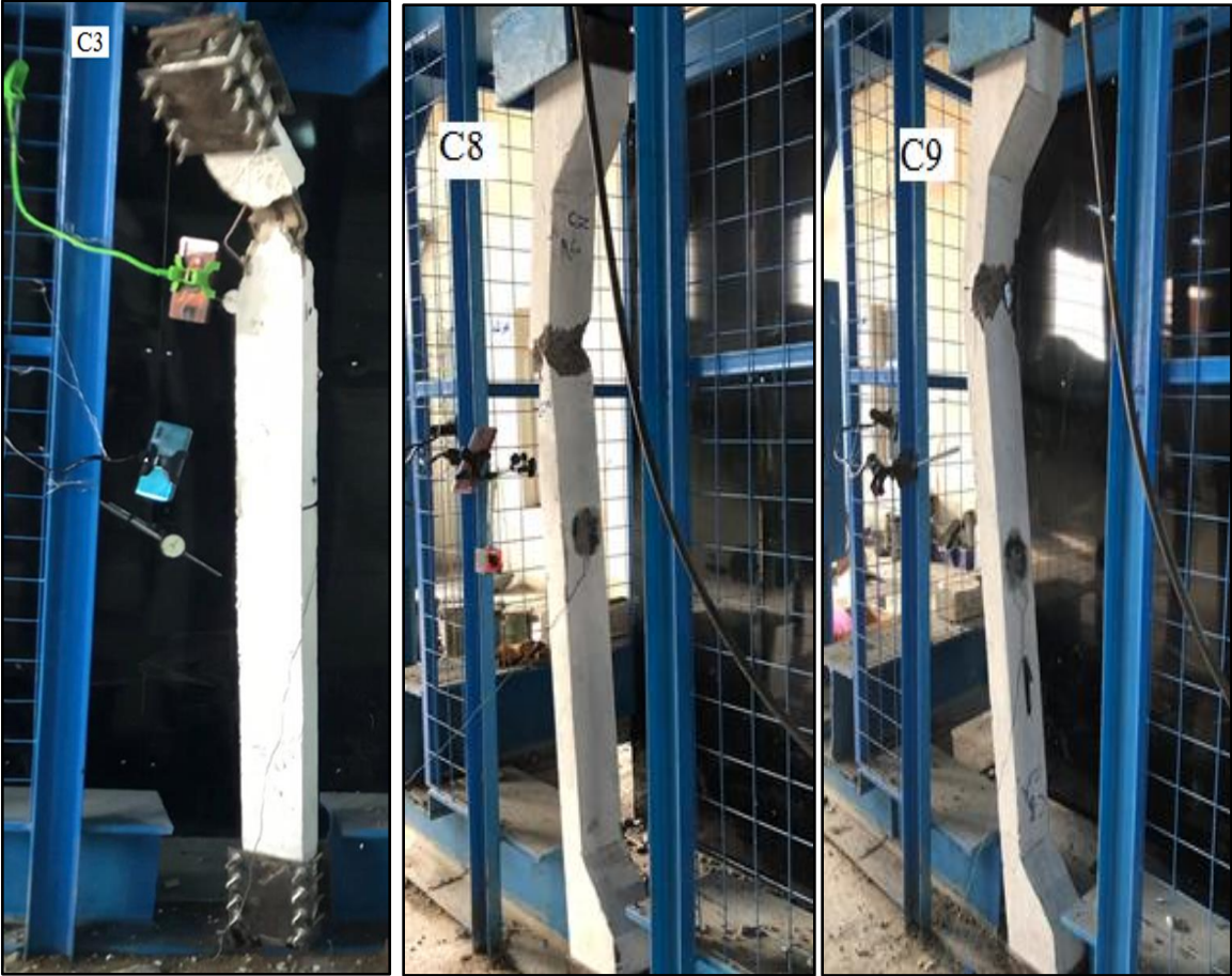
Fig. 4.15 Mode failure of columns during the test for third group.
