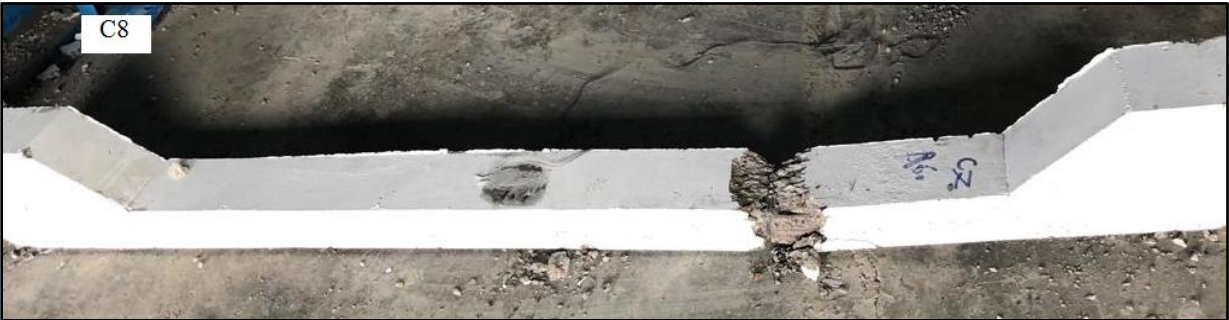
Fig. 4.16 Mode failure of columns after the test for third group.
