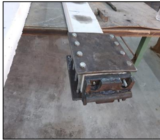
Fig. 3.29b end column cap (top view).
