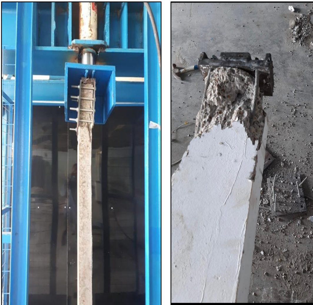
Fig. 3.31 The failure of experimental work of an experimental column.
