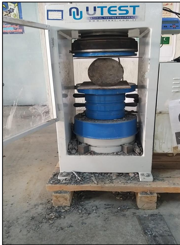
Fig. 3.26 Splitting tensile strength test.
