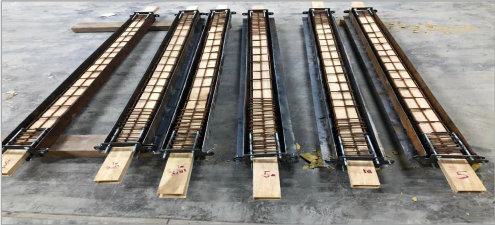
Fig. 3.16 Steel Reinforcement cage and molds without corbel.
