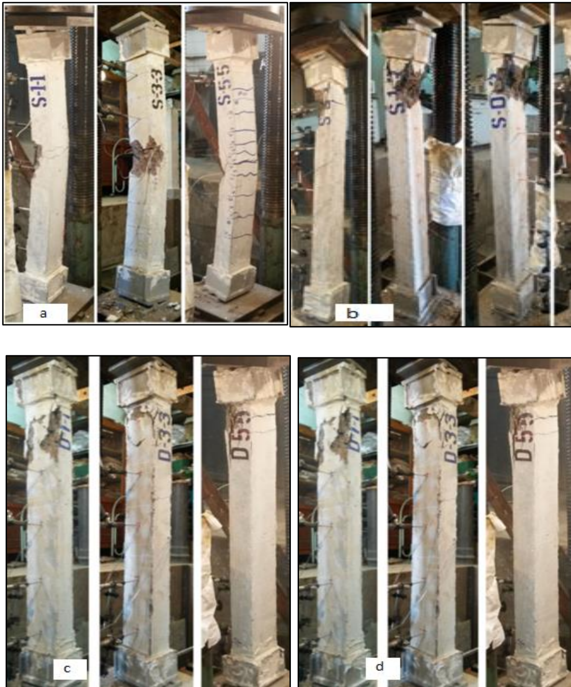
Fig. 2.1 Final failure modes for all columns a- group No. (1)
