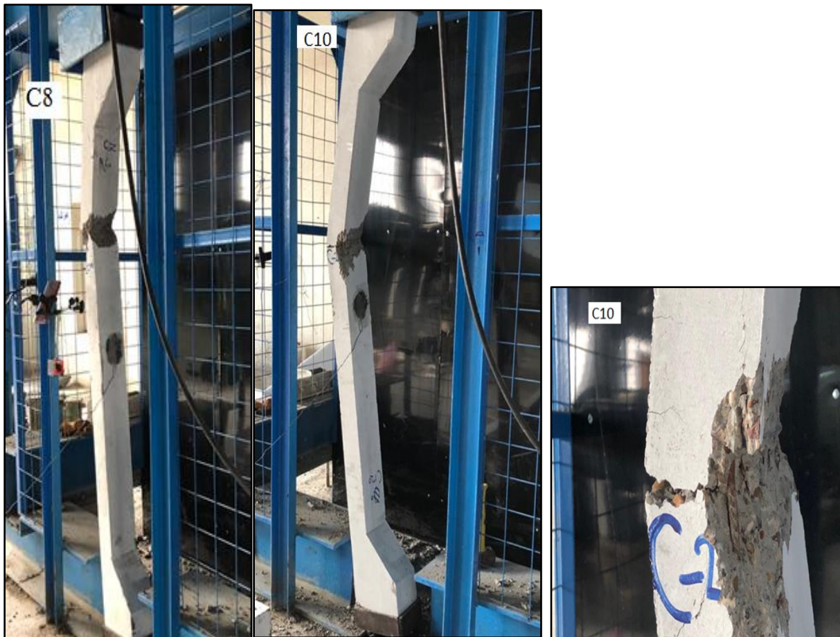
Fig. 4.20 Mode failure of fourth group.
