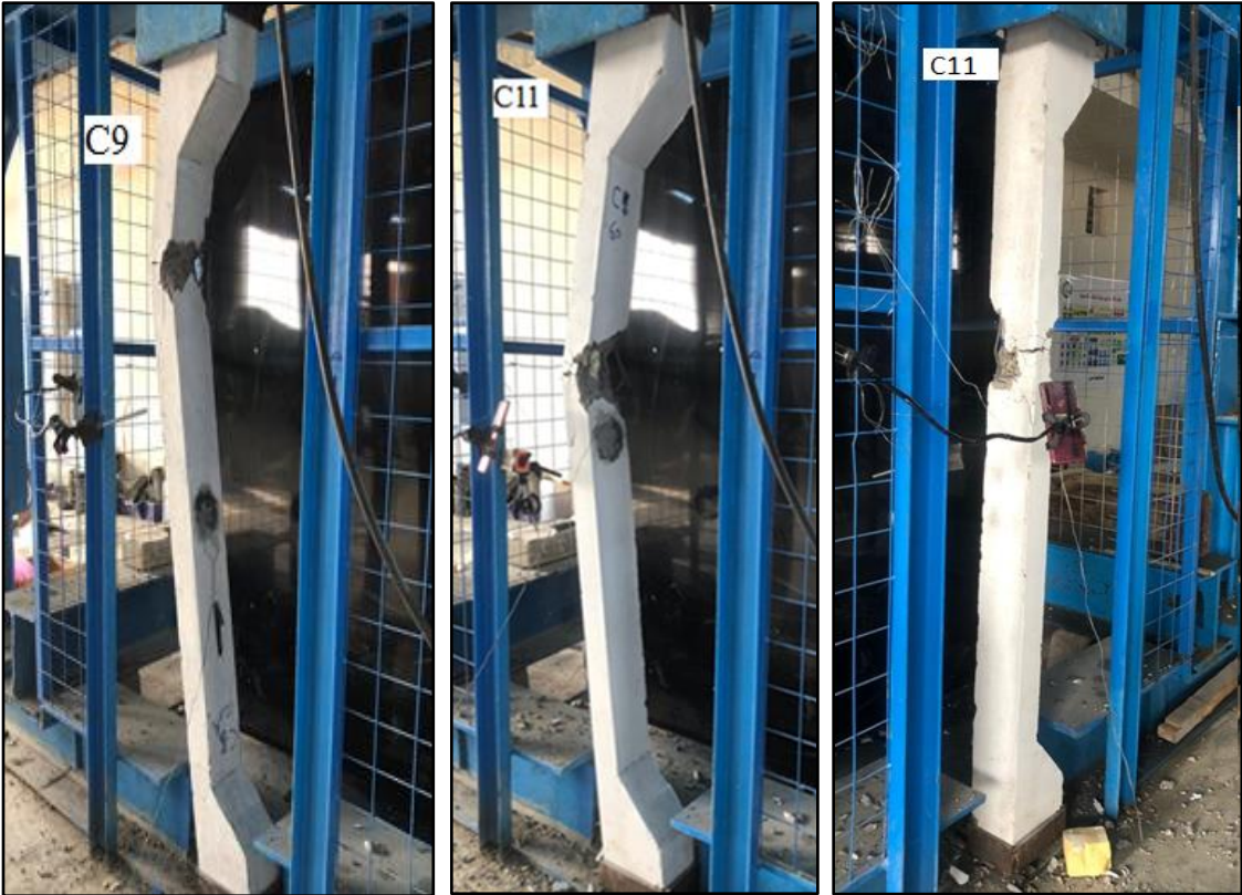
Fig. 4.24 Mode failure for fifth group .
