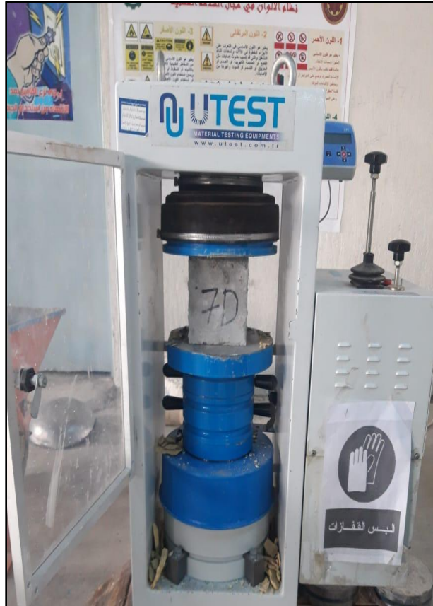
Fig. 3.25 Concrete compressive strength test.
