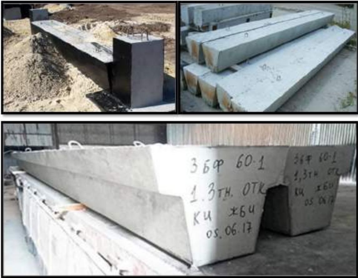
Plate (1.1) Trapezoidal reinforced concrete section
