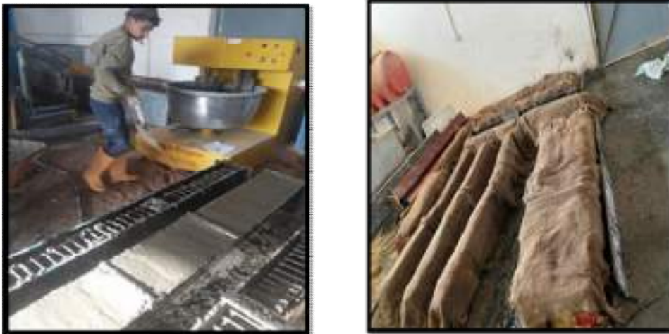
Plate (3.7) Casting and curing procedure of the specimens
