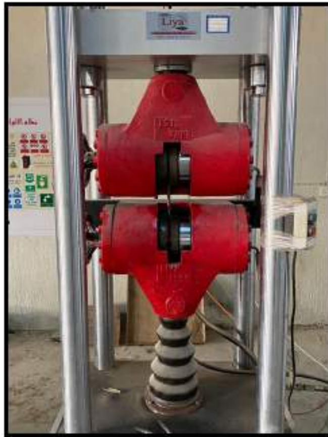
Plate (3.1) Tensile strength of reinforcement test bars
