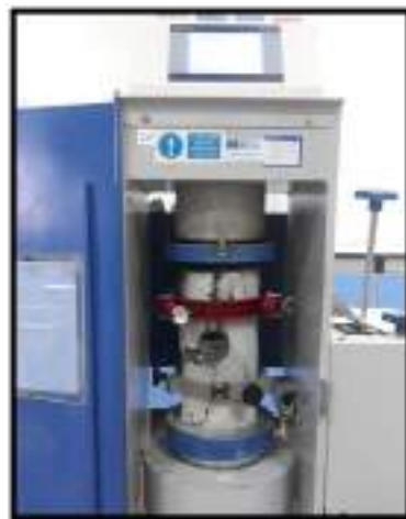
Plate (3.5) Modulus of elasticity test setting
