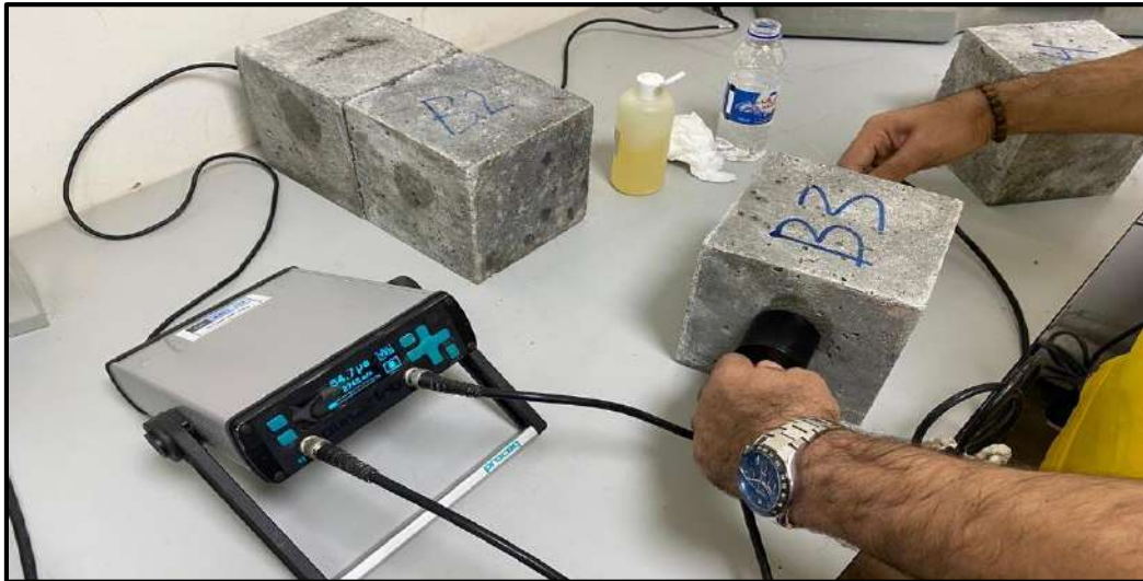
Figure 3.13 The Ultrasonic Pulse Velocity Test.
