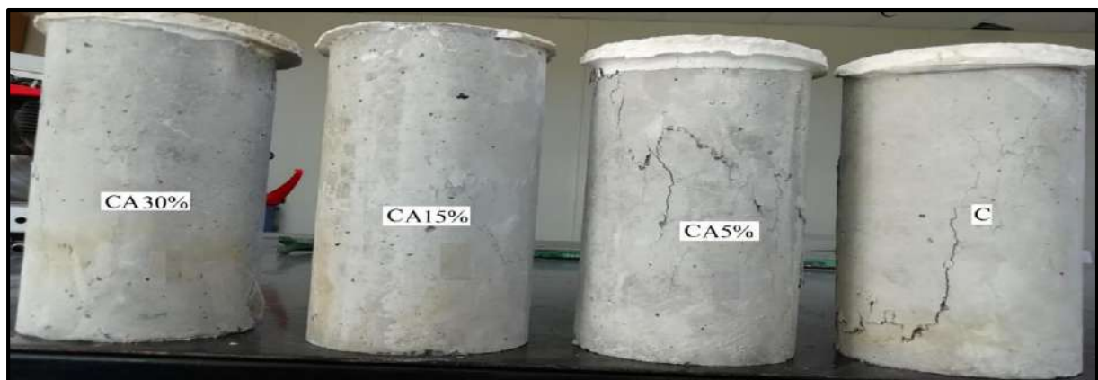
Figure 2.24 cylinder failure mode under tensile load [40].
