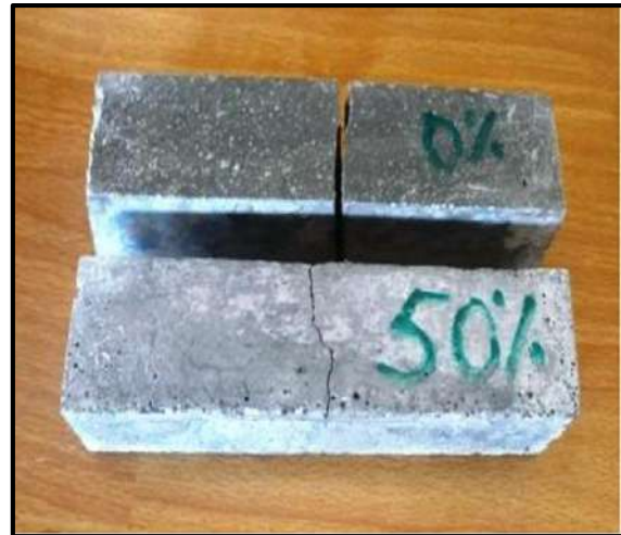
Figure 2.22 Comparison between reference and 50% PVC under flexural test [39].
