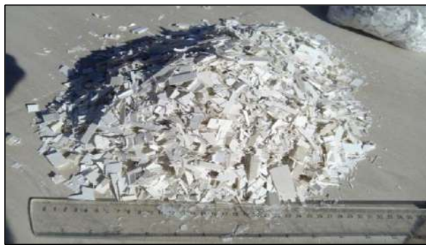
PVC from primary crushing
