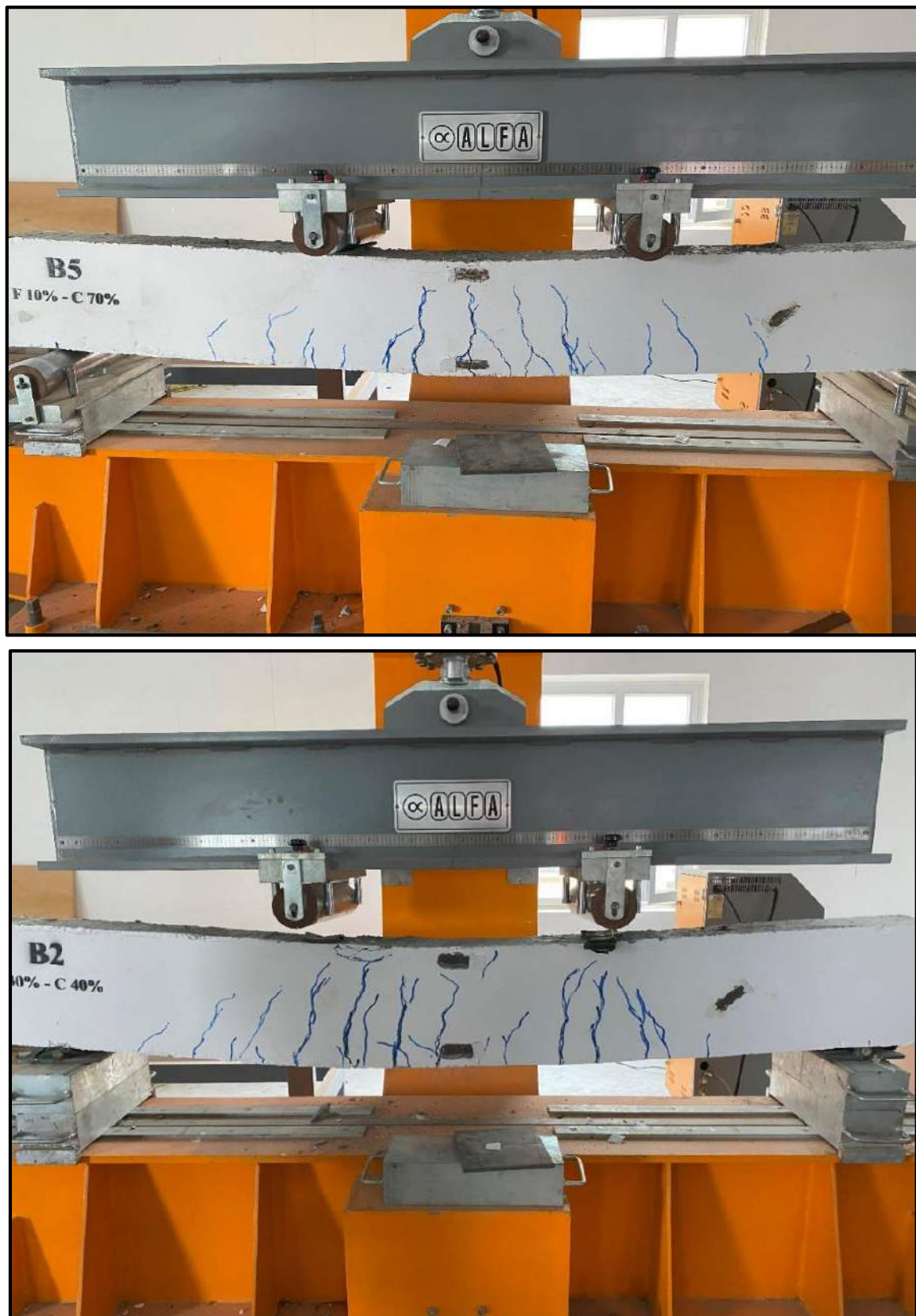
Figure 4.9 The Lightweight Concrete Beams under the load.
