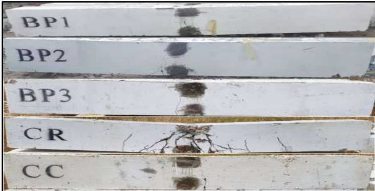
Figure 2.13 cracks modes in concrete beams [31]
