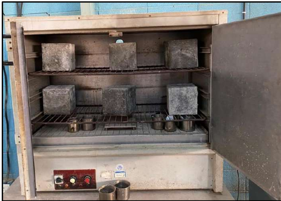
Figure 3.12 Drying the Specimens in the Oven.
