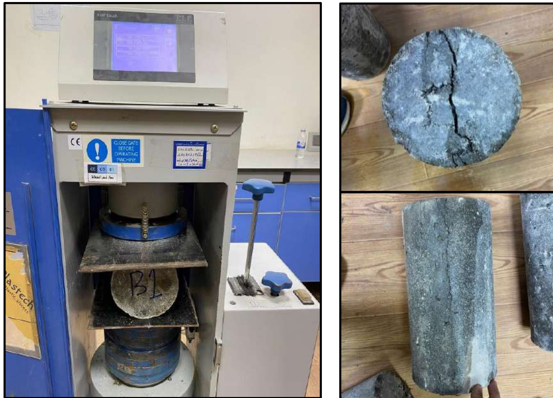
Figure 3.10 The Splitting Tensile Test.
