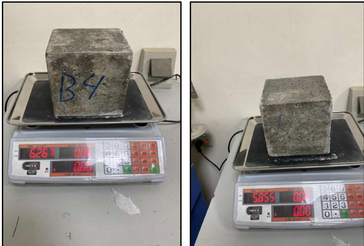
Figure 3.8 The Density Test.
