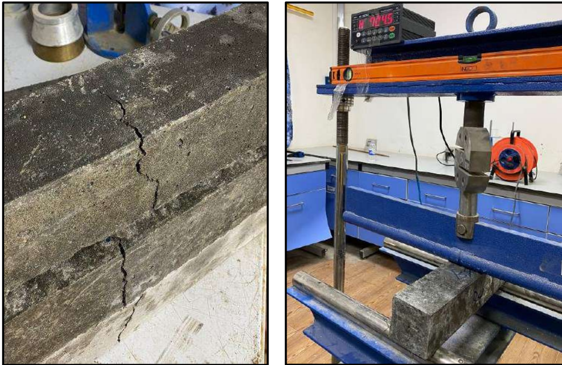
Figure 3.11 The Flexural Strength Test.
