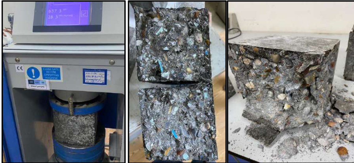
Figure 3.9 The Compressive Test.
