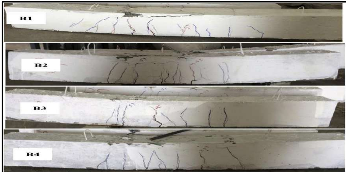
Figure 2.11 failure modes of reinforced concrete beams [30].
