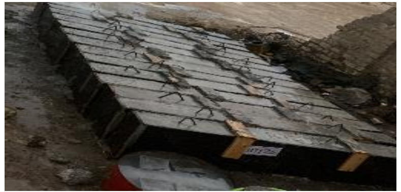
Figure 3.8: Fabrication, moulds, and casting of the specimens.
