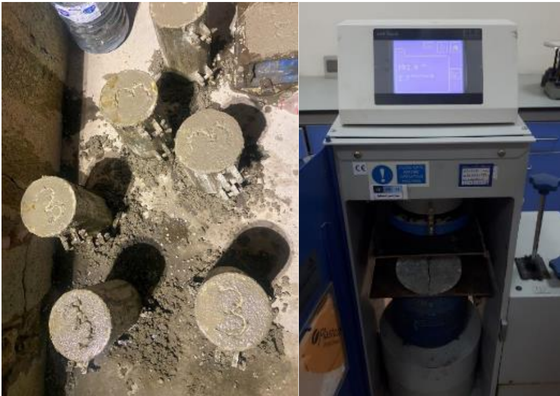
Figure 3.4: Test of splitting tensile strength.
