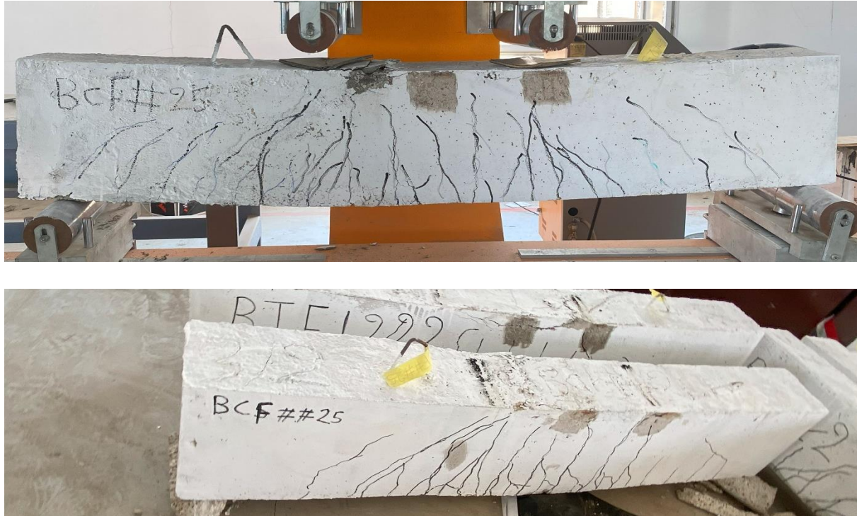
Figure 4.22: Cracks pattern for beams/ Mode I
