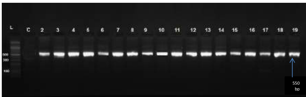
Figure (3-6): Agarose gel electrophoresis of PCR chromosome encoded bla CTX-M gene, amplicon (550bp), where L: ladder (100bp) , Lane(2-19) positive results, C: Control (only primer+ Master Mix), the gel stained by ethidium bromide (0.5 µg/ml) and (65) volts for one hour.
