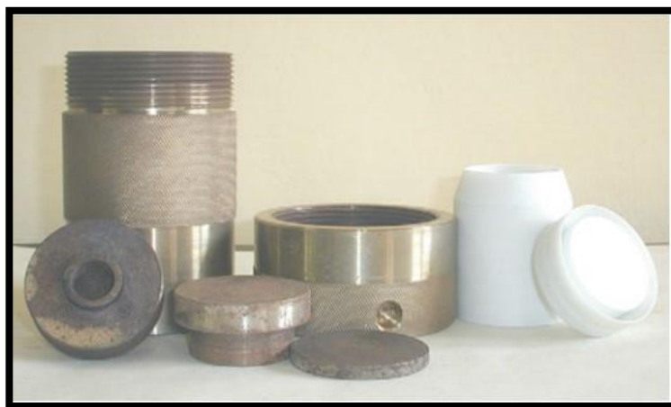
Fig. (1-9) A general-purpose Hydrothermal autoclave. The Hydrothermal reactions occur inside the Teflon container[42]
