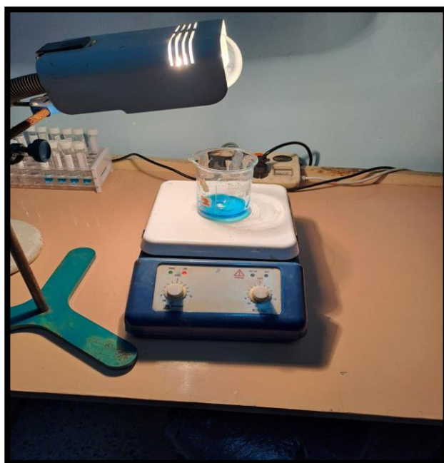
Fig. (2-3) Hotplate with magnetic stirrer under Tungsten lamp- 300 watt
