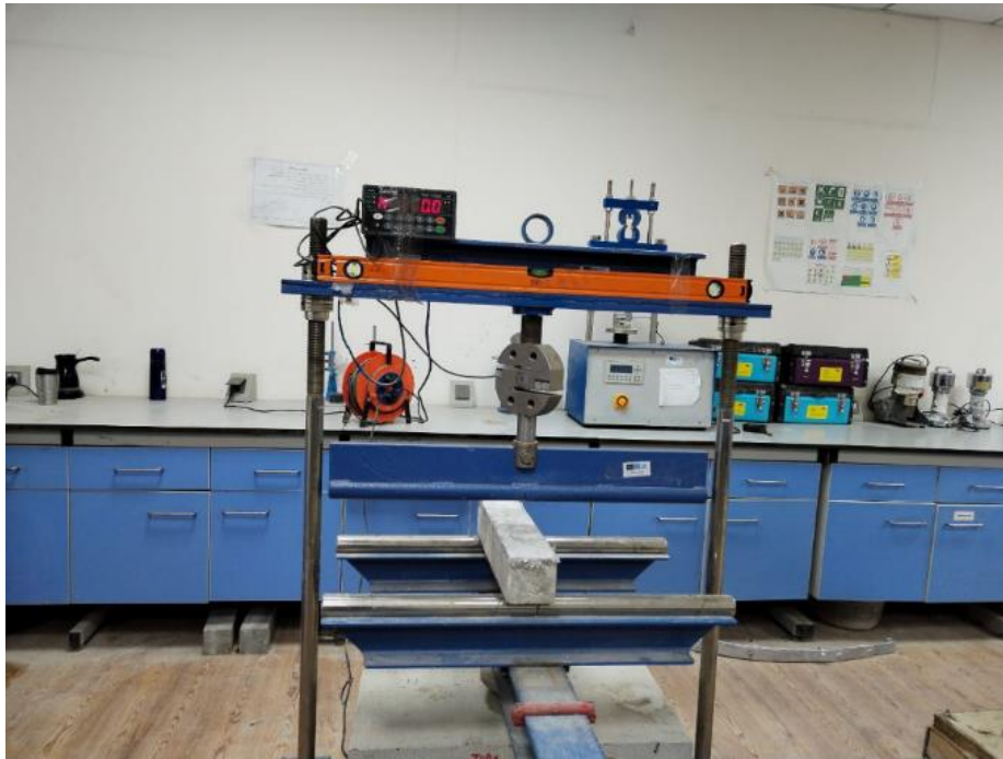
Figure 3.11 Flexural Strength Testing Machine For Concrete Prisms.
