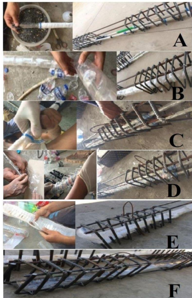
Figure 2.15 Type of PET Waste Bars as a Tension Reinforcement [25].
