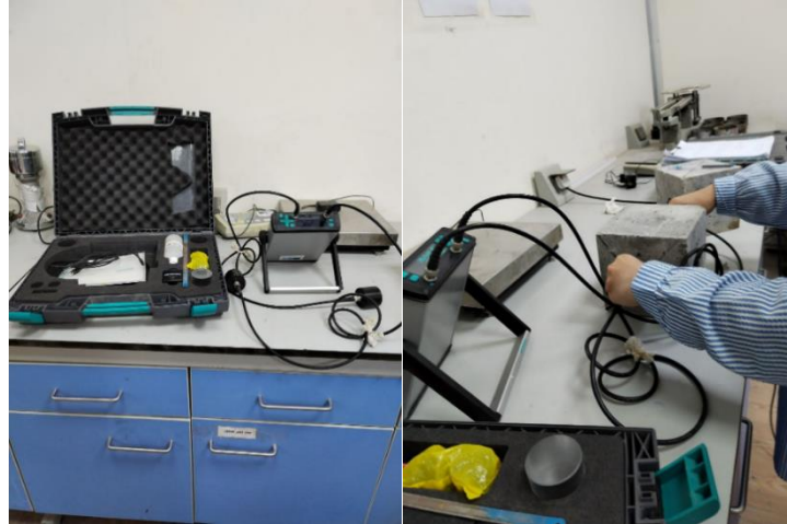
Figure 3.16 Ultrasonic Pulse Velocity (UPV) Test for Concrete Cubes.
