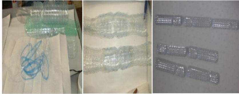
Figure 2.11 Forms of PET used (Circular fibers ,half bottles ,and strips) [22].
