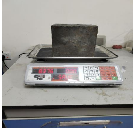
Figure 3.14 Dry Density Test of The Concrete Cubes.
