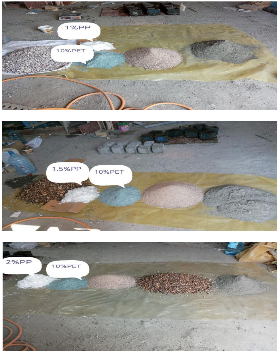
Figure 3.4 The Components of the concrete mixture.
