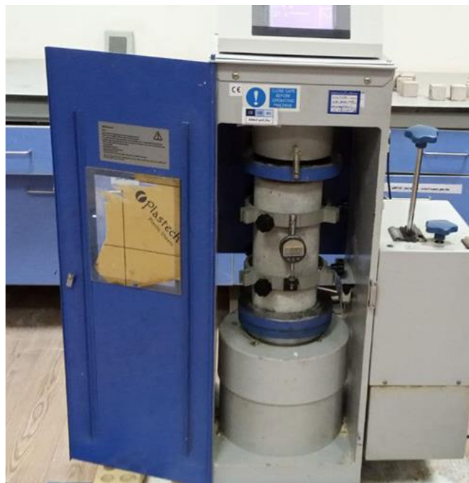
Figure 3.13 Modulus of Elasticity Test for Cylindrical Specimens.
