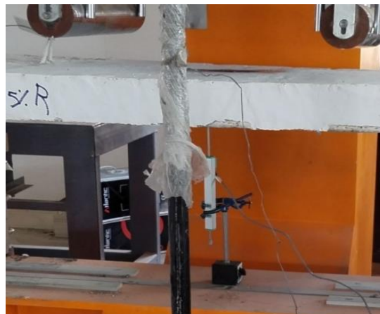
Figure 3.21 The Position of LVDT on the Slab.
