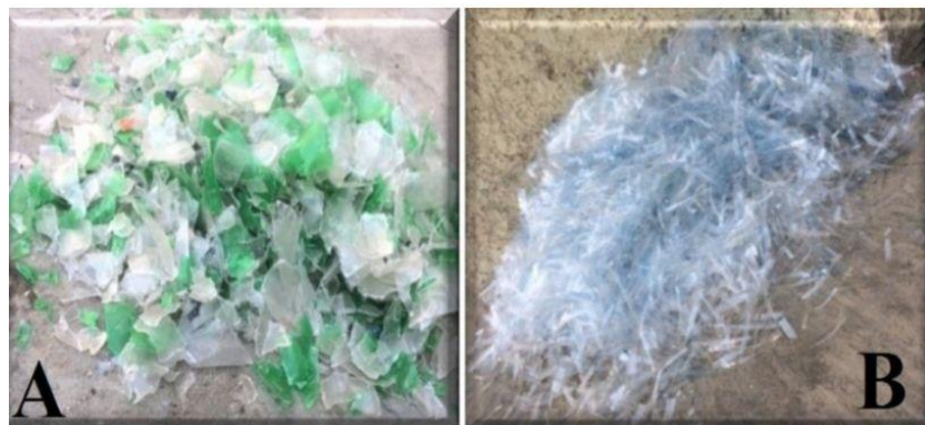
Figure 2.10 Type of PET Waste Fibers [21].
