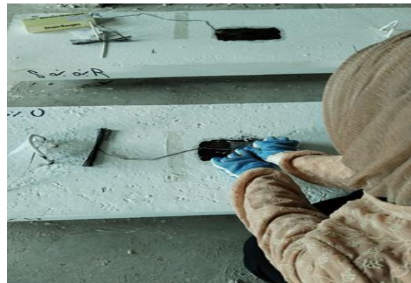
Figure 3.23 Paste Gauges on The Concrete Slabs.
