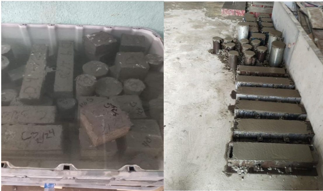
Figure 3.8 Process of Casting and Curing.
