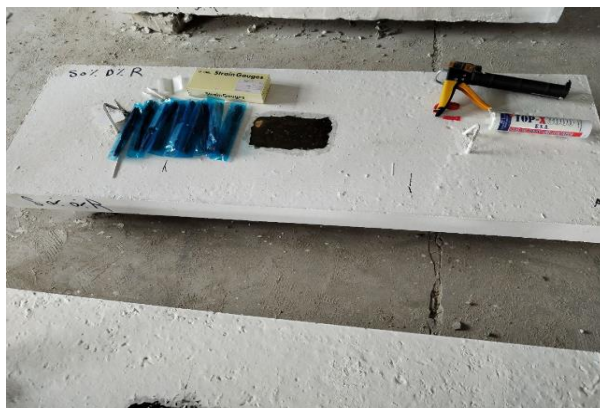
Figure 3.23 Paste Gauges on The Concrete Slabs.
