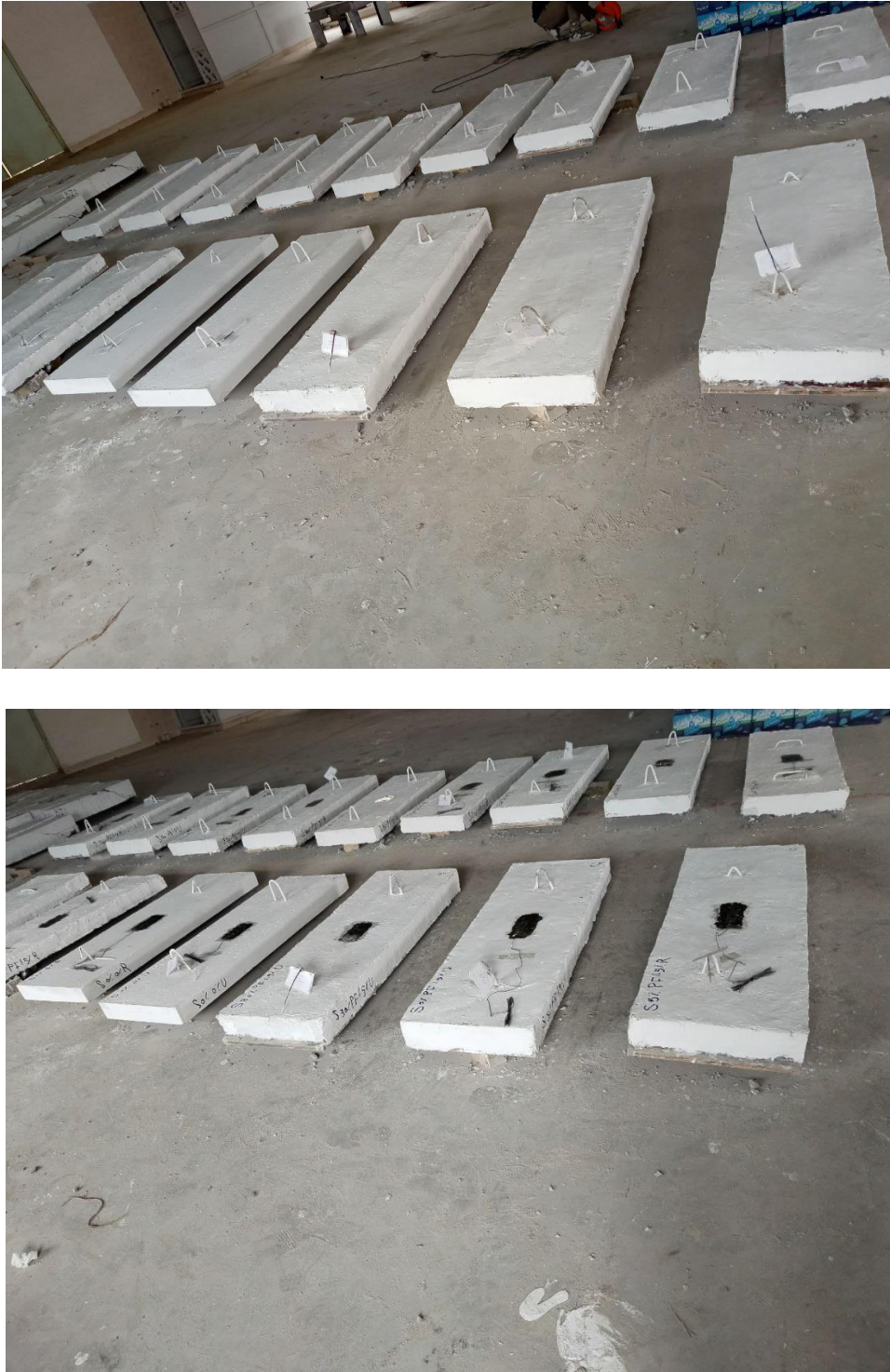
Figure 4.12 Concrete Slab Specimens used for all PET /SAND Percentage.
