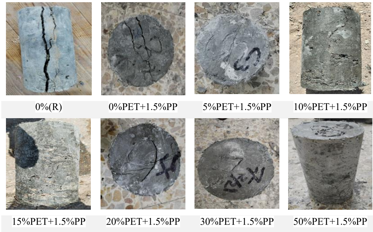
Figure 4.5 Mode Failure of Splitting Tensile Specimens.
