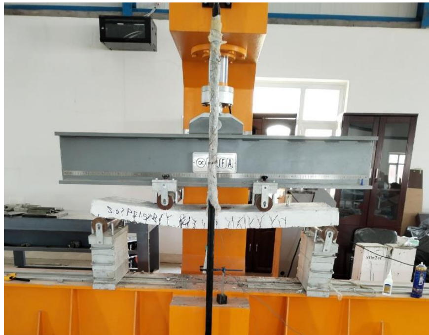
Figure 3.24 Flexural Test of Slabs.
