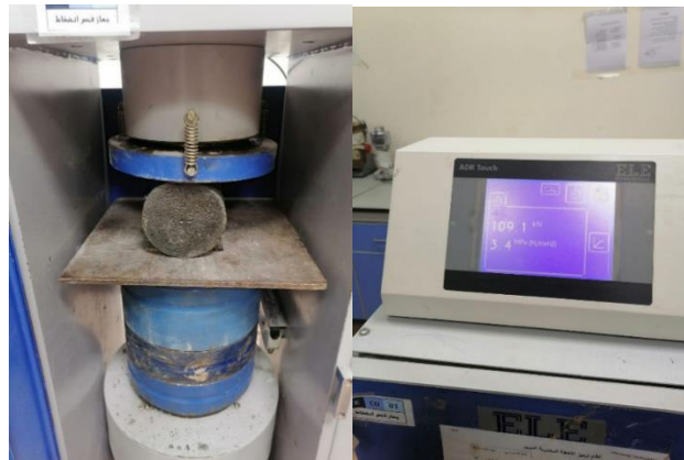
Figure 3.12 Splitting Tensile for Test Concrete Cylinders.
