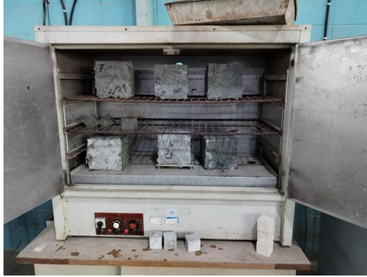
Figure 3.15 Water Absorption Test of Concrete Cubes Specimens.
