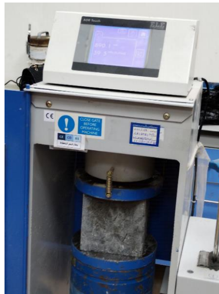
Figure 3.10 Compression Testing Machine for Concrete Cubes.
