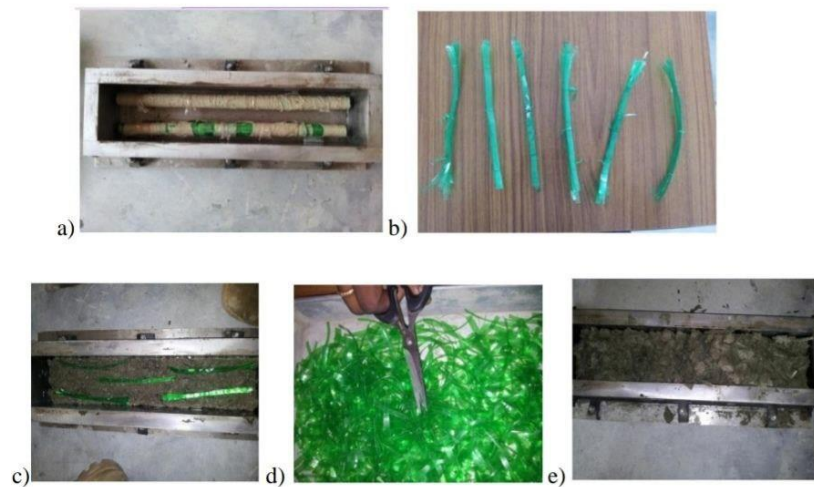
Figure 2.13 :a) PET Hollow Bars, b) PET Long strips, c) PET Long strips as reinforcement along with steel, d) PET Short strips, and e) Concrete with PET Short strips filled in beam mold [23].
