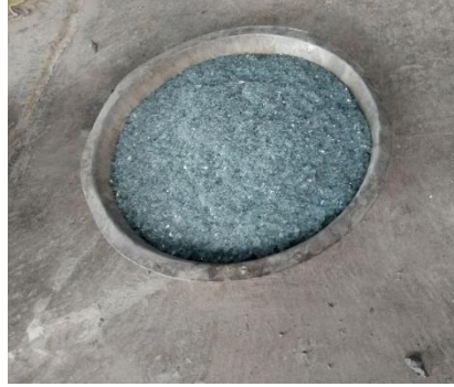
Figure 3.1 PET Molecules Produced by Chopping Water Bottles and Soft Drinks.
