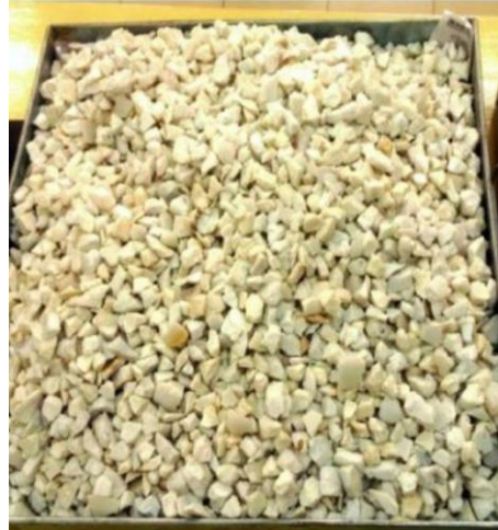
Figure 2.5 PET as a Coarse Aggregate [15].
