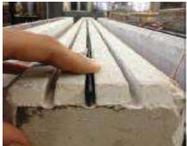
b) NSM strips in the grooves.
