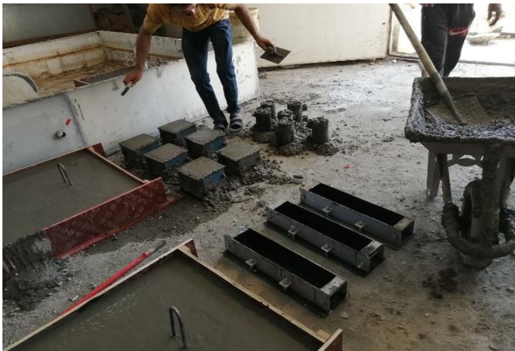
Figure 3.19 Take of concrete samples
