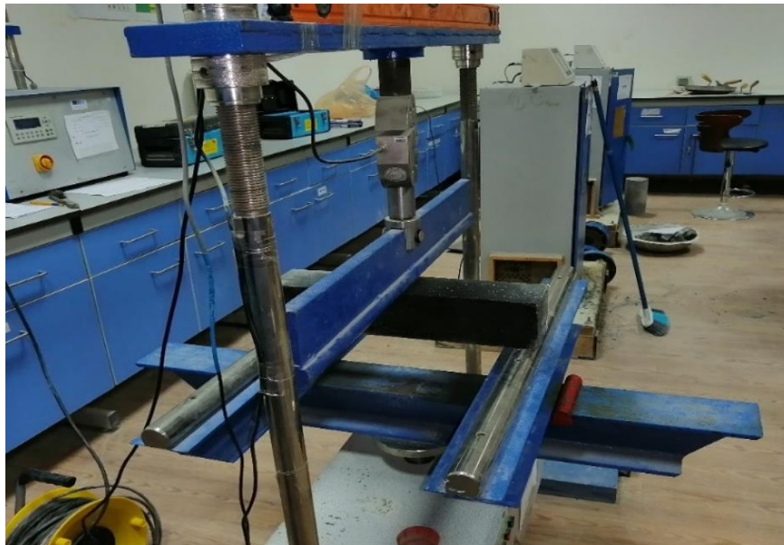
Figure 3.23 Flexural test of specimen
