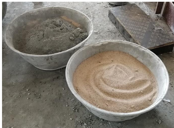
Figure 3.3 Krista portland cement and sand
