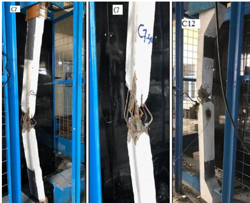
Figure 2-13 Failure Mode of Specimens [4].
