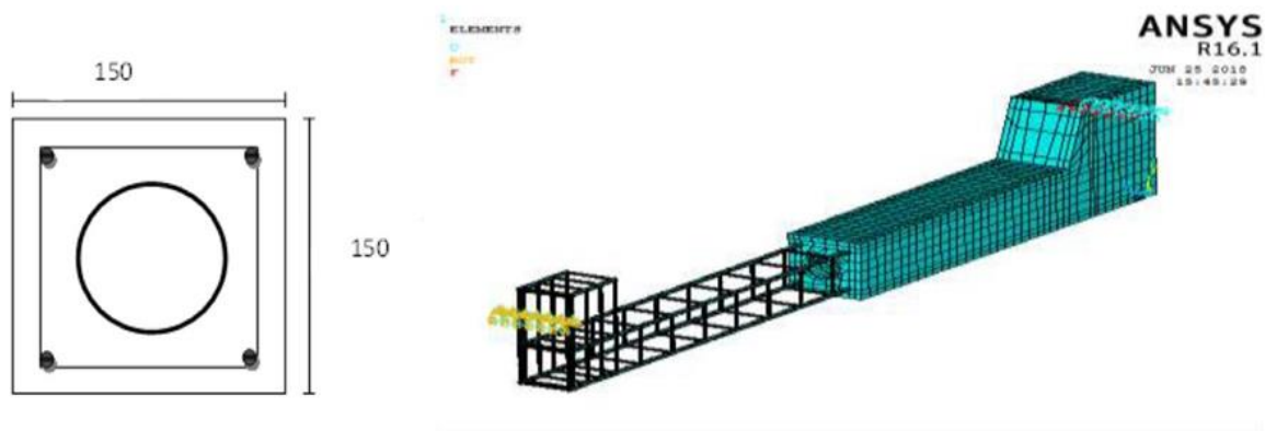
Figure 2-7 Modeling and Meshing of the Analyzed Columns by [45].
