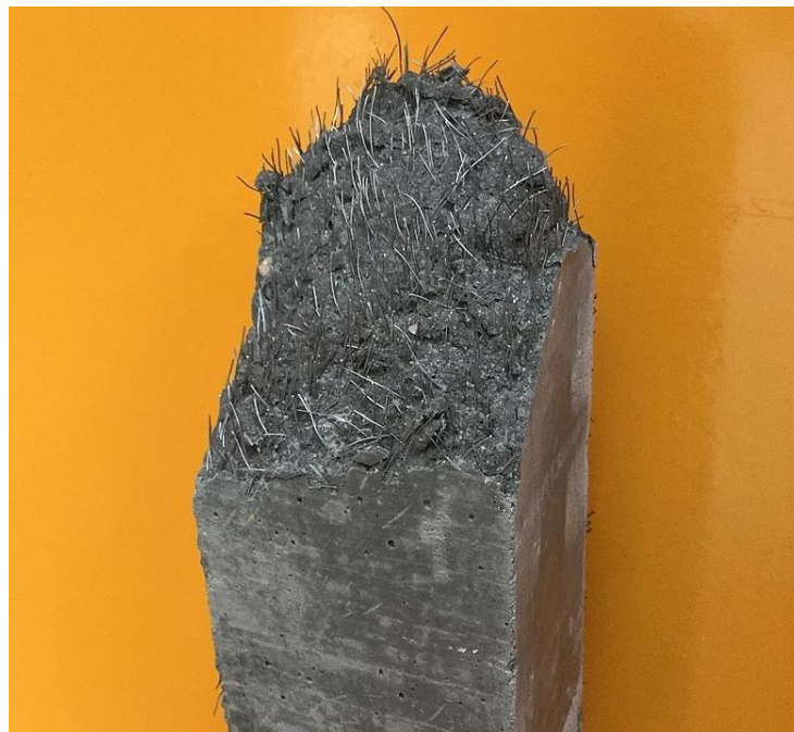
Figure 1-9 Steel Fiber Reinforced Concrete Column (SFRCC).
