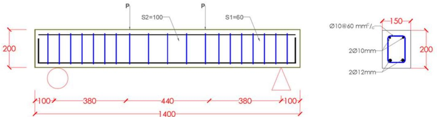
Fig. (3-11) Dimensions and details of beam specimen
