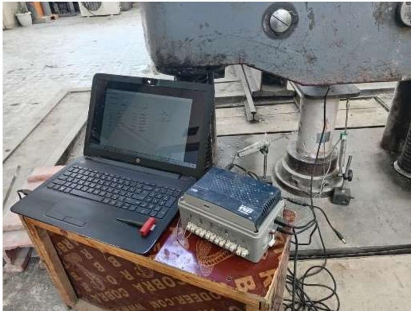
Fig. (4-11) Energy absorption and elastic modulus test
