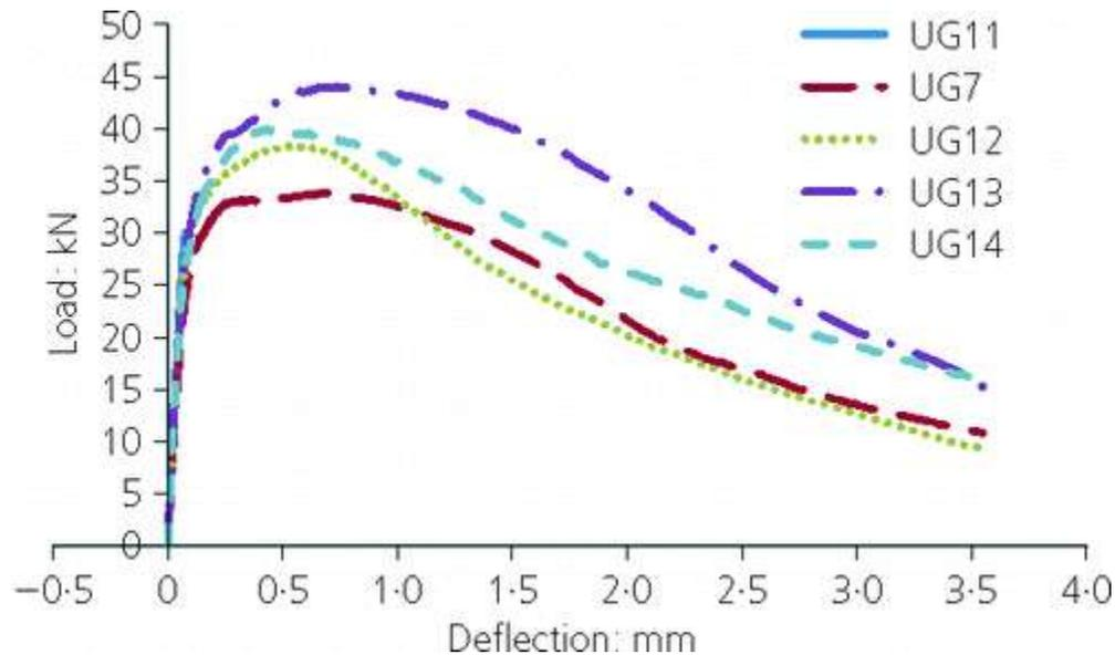
Fig. (2-2) Load–deflection for UHPGPCs with (UG7, UG12–UG14) and without (UG11) fibre [68]
