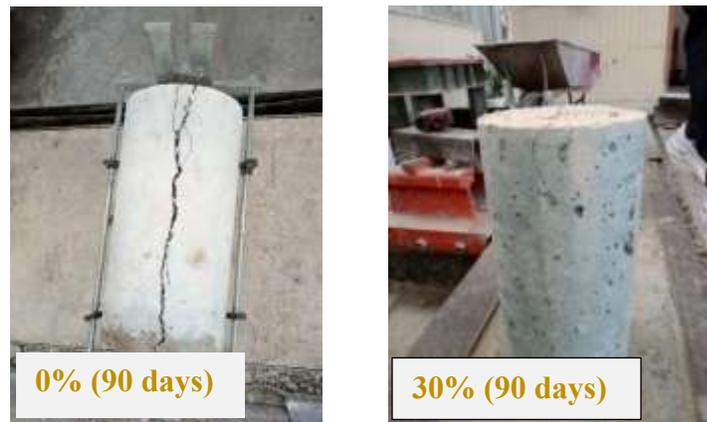
Fig. (4-5) Concrete cylinders failure modes for PET percentages as a sand replacement
