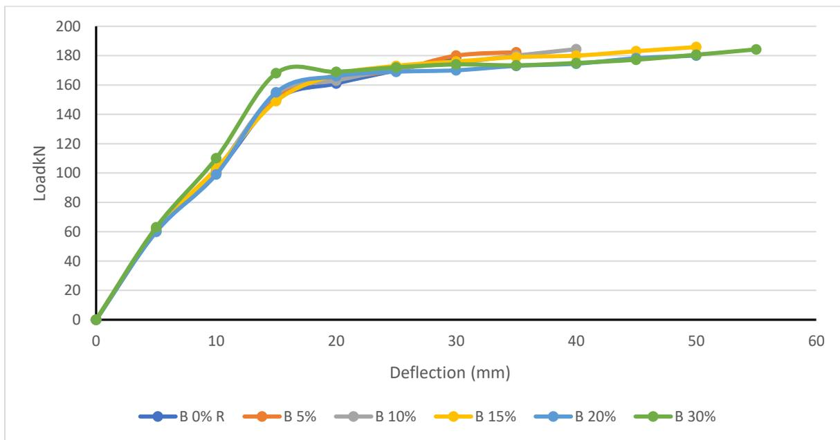
Fig. (4-19) Load to deflection curve for beams specimens
