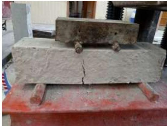
Fig. (3-15) Flexural Strength Test
