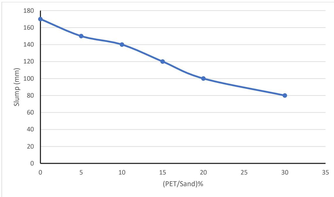
**Fig. (4-1) Slump for PET percentages as a sand replacement**
