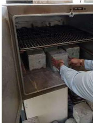
Fig. (3-16) Drying the specimens of absorption test in the oven
