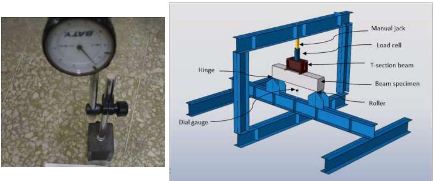
Fig. (3-19) Dial gauges used in tests
