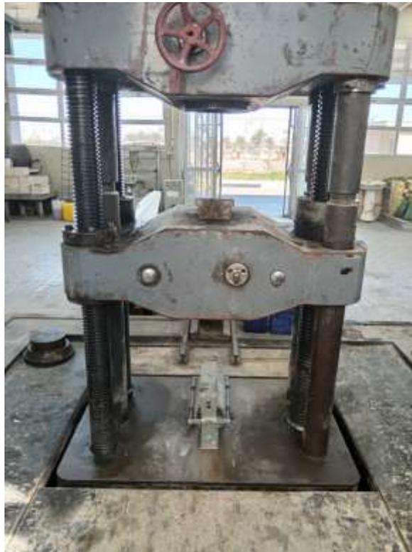
Fig. (3-14) The Universal testing machine
