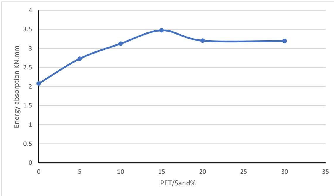
Fig. (4-14) Energy absorption to (PET/Sand) relation
