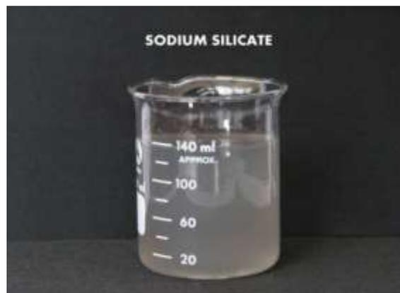
Fig. (3-2) Sodium Silicate Solution
