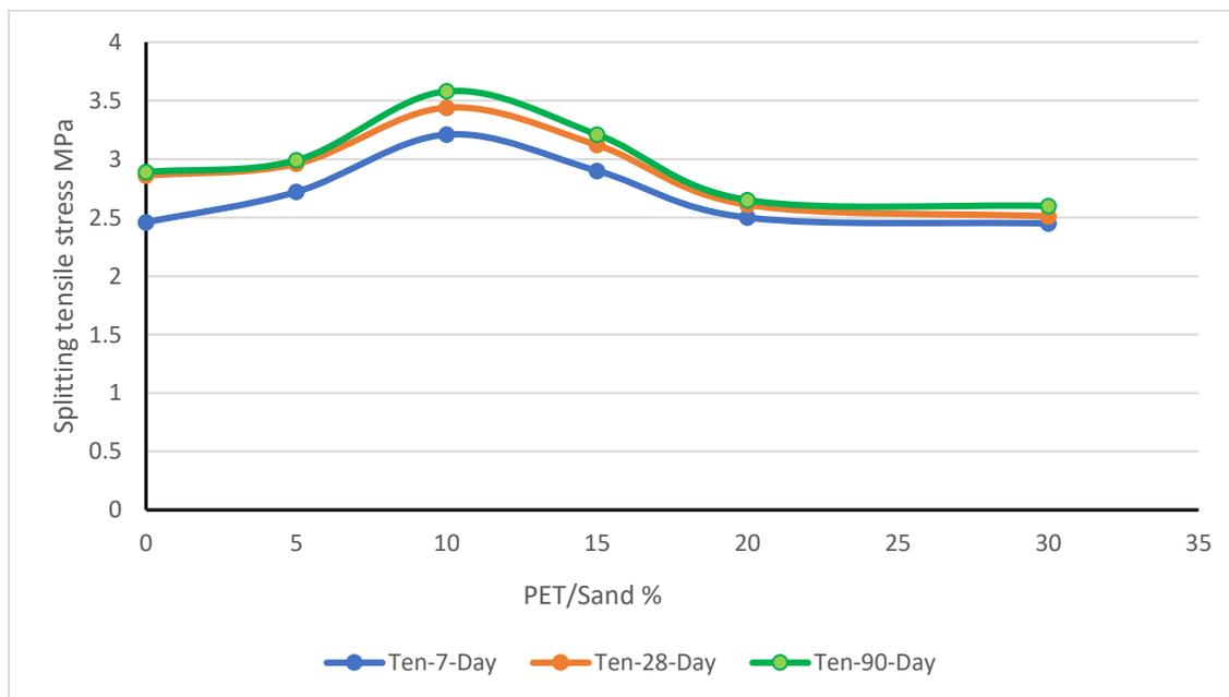
Fig. (4-4) Split tensile strength result for PET percentages as a sand replacement
