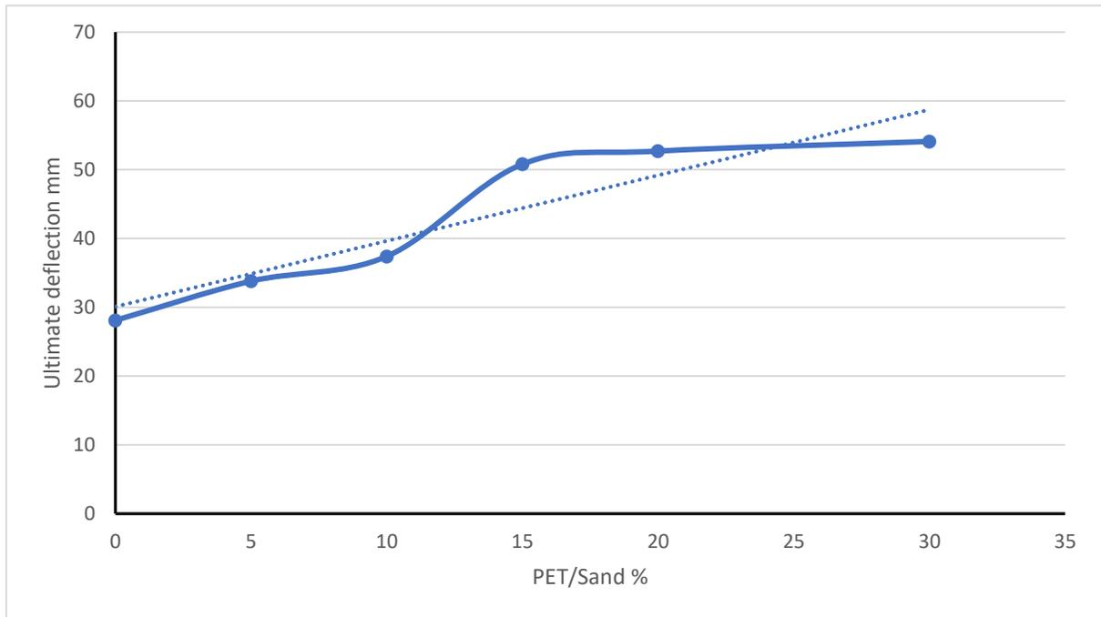
Fig. (4-18) Relation between maximum deflection to (PET/Sand) for beams specimens
