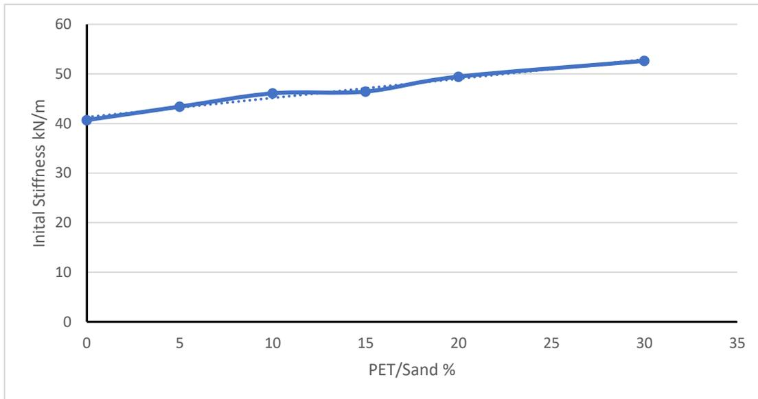
Fig. (4-22) Relation between Initial stiffness to (PET/Sand) for beams specimens containing PET as a sand replacement
