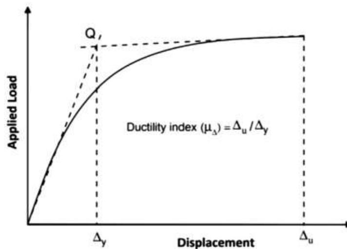
Fig. (4-21) The calculation method of Secant and Initial stiffness [55]
