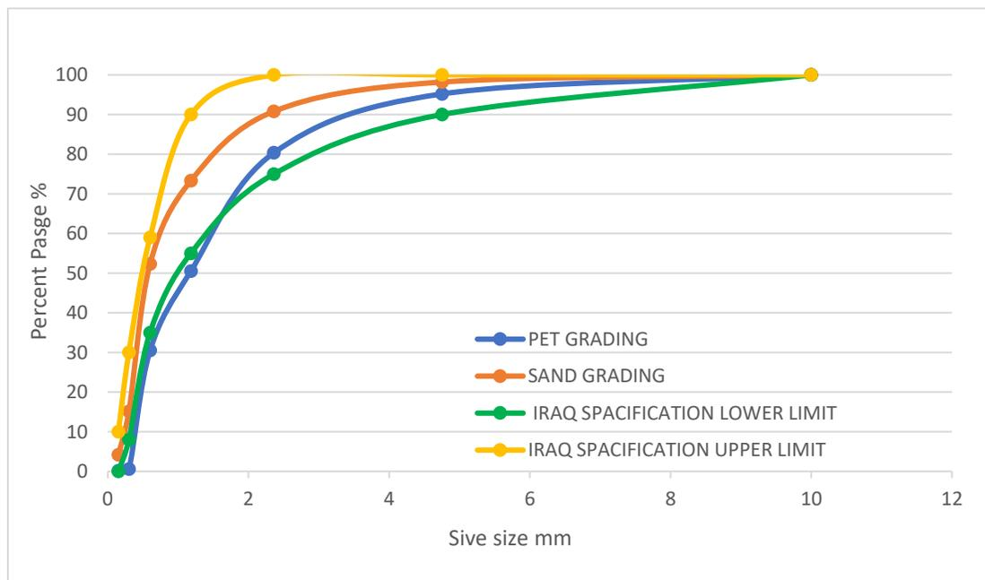
Fig. (3- 4) Grading curve for original PET waste and fine aggregate
