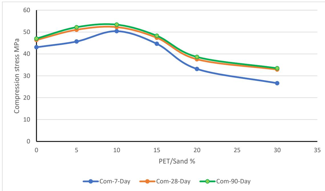
Fig. (4-2) Compressive strength curves for PET percentages as a sand replacement
