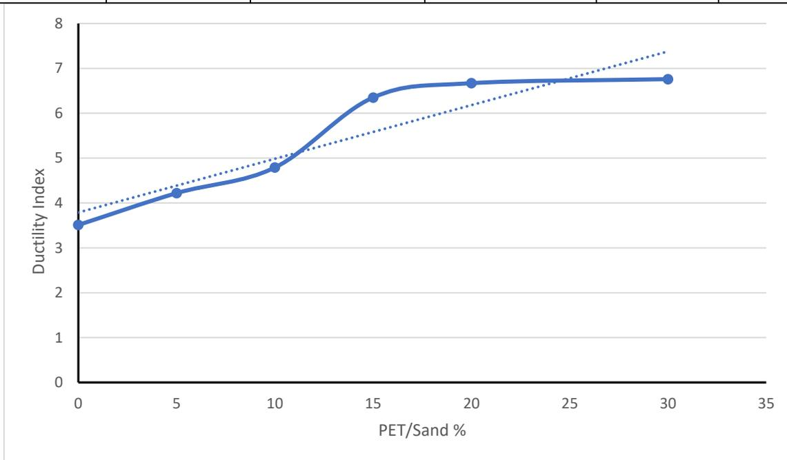
Fig. (4-20) Ductility index-(pet/sand) relation for beams containing PET as a sand replacement
