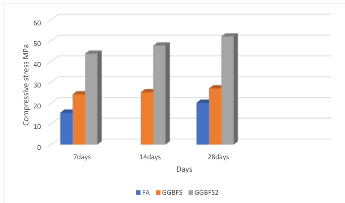
Fig. (3-8) Compression strength to geopolymer concrete cubes for the pre-trial experiment work
