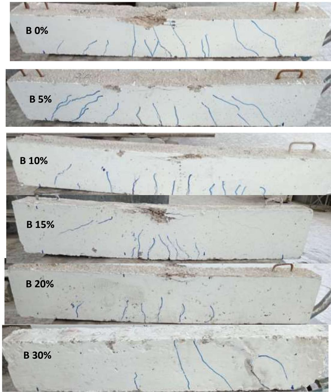
Fig. (4-27) Cracks pattern for beams specimens containing PET as a sand replacement
