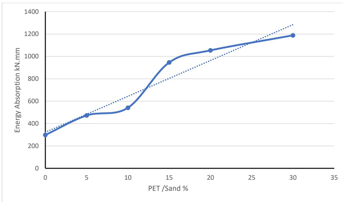
Fig. (4-24) Relation between Absorption of energy to (PET/Sand) curve for beams specimens containing PET as a sand replacement
