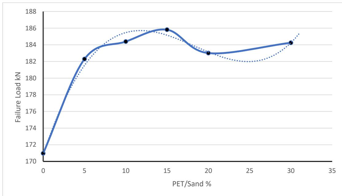
Fig. (4-17) Ultimate load to (PET/Sand) relation curve for beams specimens containing PET as a sand replacement
