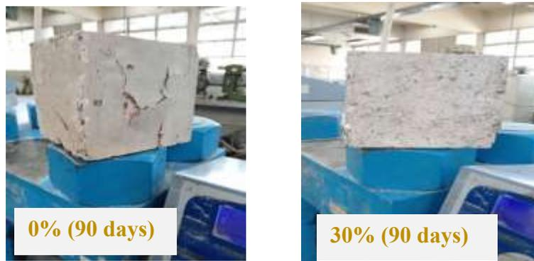
Fig. (4-3) Concrete cubes failure modes for PET percentages as a sand replacement
