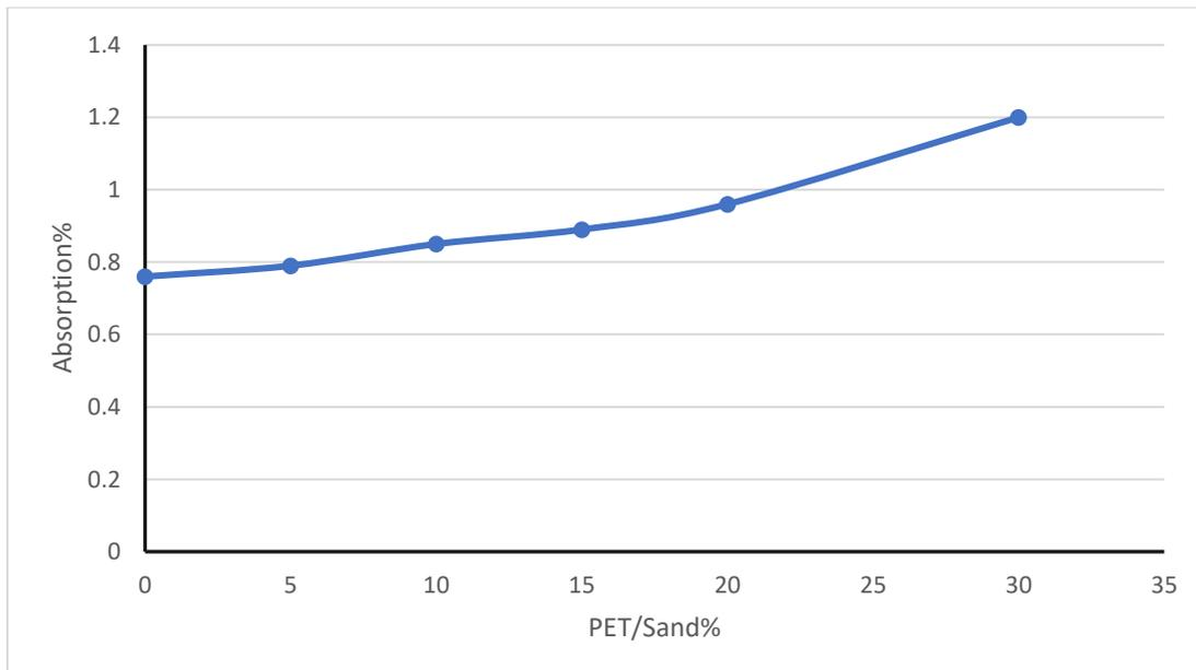
**Fig. (4-9) The absorption curve for PET percentages as a sand replacement**
