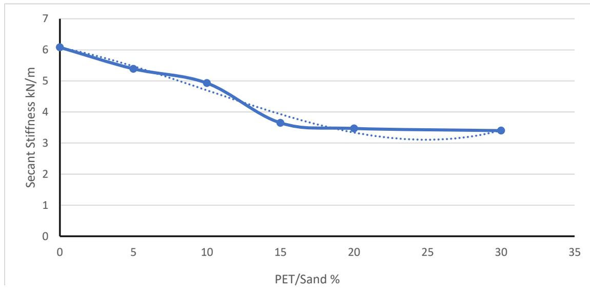
Fig. (4-23): Relation between Secant stiffness to (PET/Sand) for beams specimens containing PET as a sand replacement
