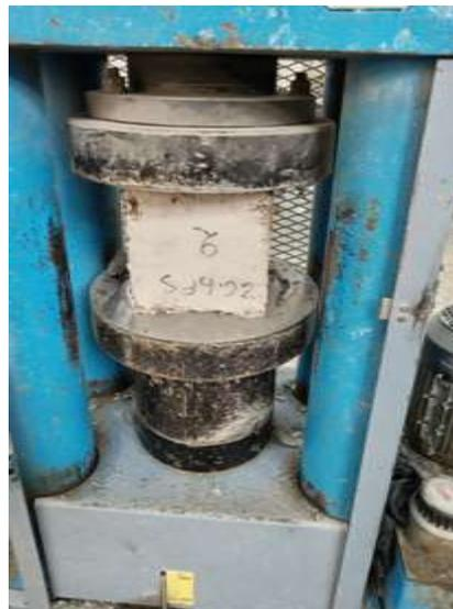
Fig. (3-13) Compression machine test
