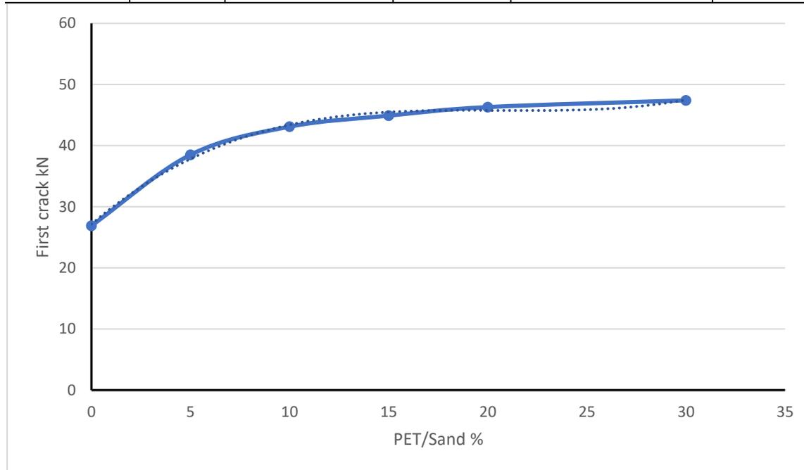
Fig. (4-25) Relation between Initial crack to (PET/Sand) curve for beams specimens containing PET as a sand replacement
