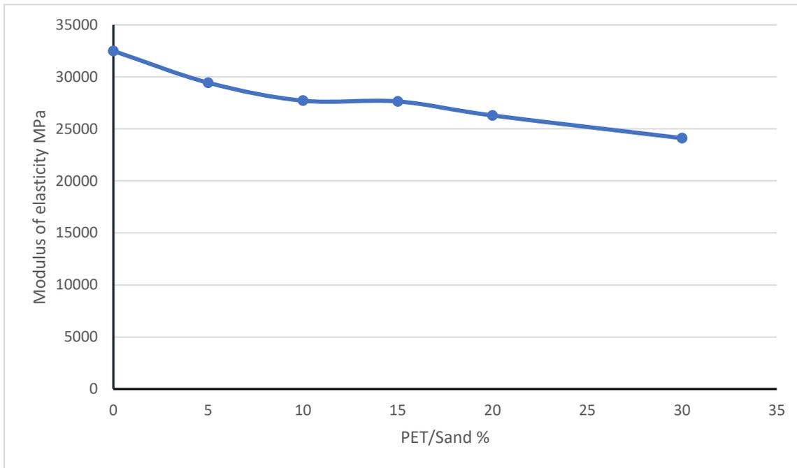
Fig. (4-13) Modulus of elasticity to (PET/Sand) relation
