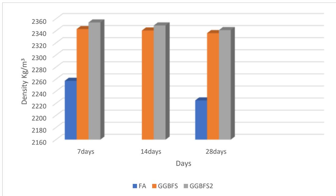
Fig. (3-9) Density to geopolymer concrete cubes for the pre-trial experiment work
