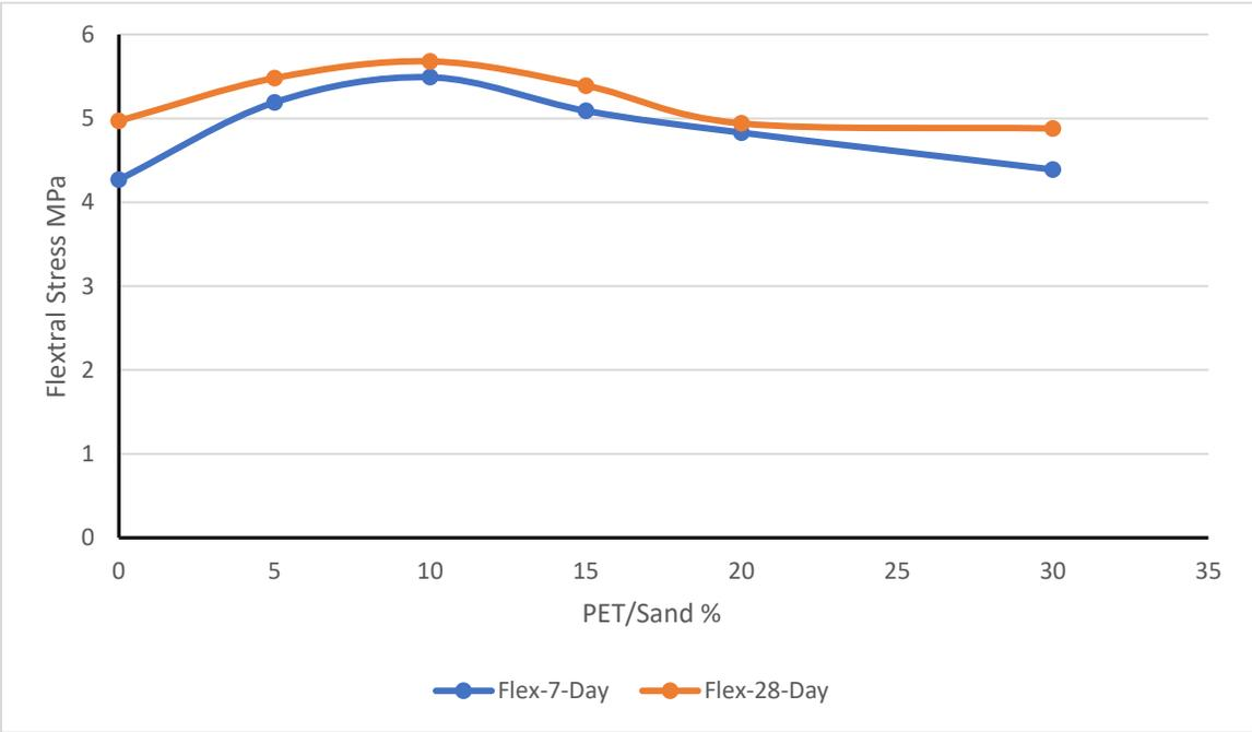
Fig. (4-6) Flexural strength results for PET percentages as a sand replacement
