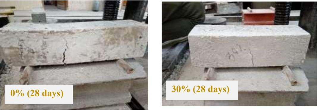
Fig. (4-7) Prisms failure modes for PET percentages as a sand replacement
