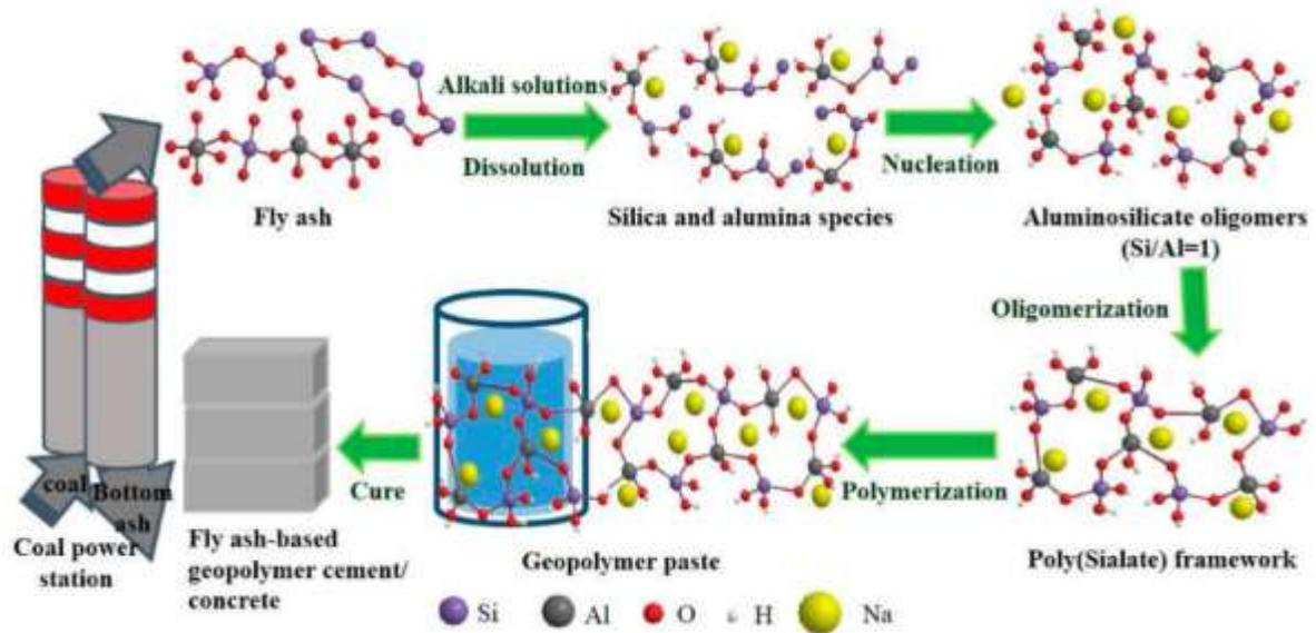
Fig. (1-2) Geopolymerization processes using fly ash [54]
