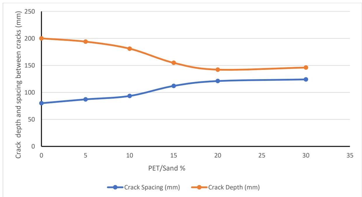
Fig. (4-26) Crack depth and spacing of crack for beams containing PET as a sand replacement
