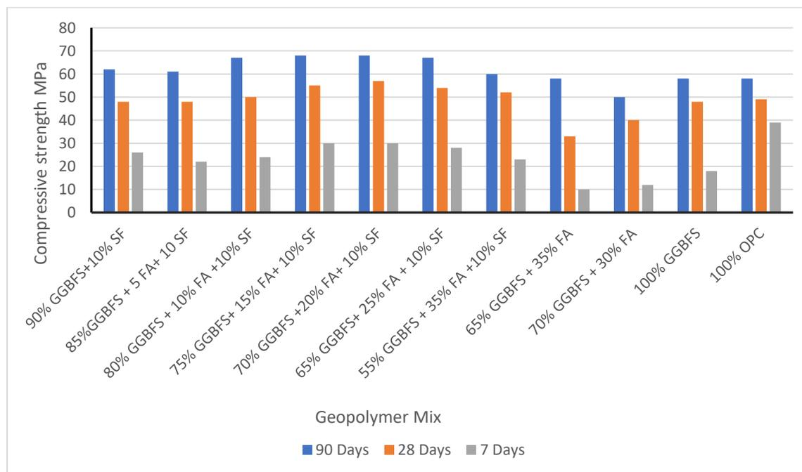
Fig. (2-3) Compressive strength of geopolymer mixes [72]
