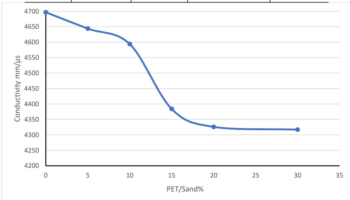
Fig. (4-10) Conductivity curve for PET percentages as a sand replacement
