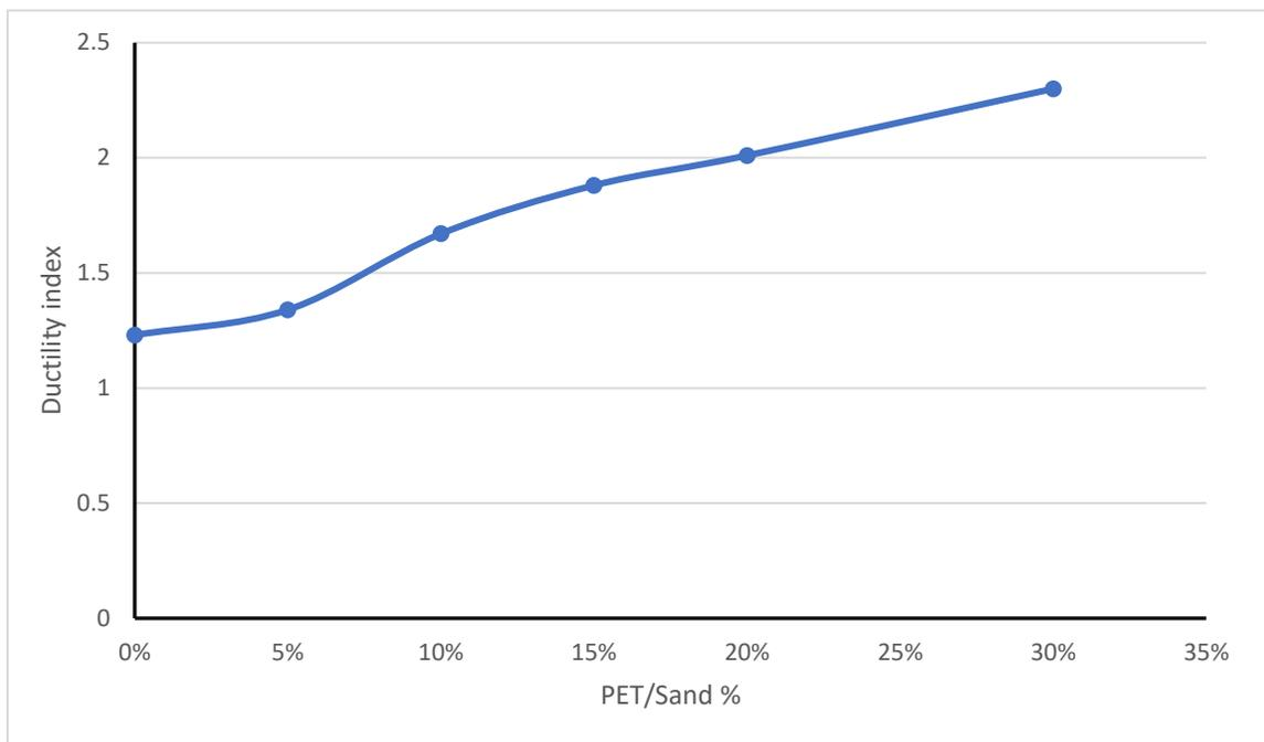
Fig. (4-16) Ductility index to (PET/Sand) relation
