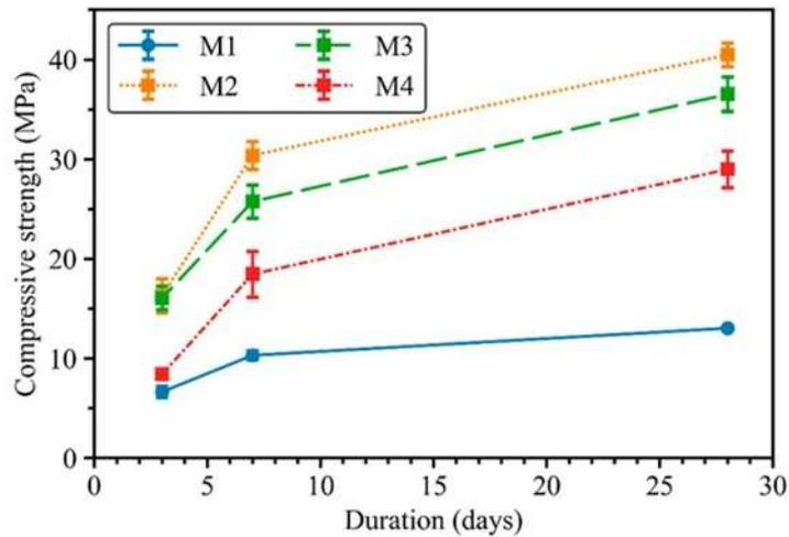
Fig. (2-4) Compressive strength of geopolymer mortar mixes [74]
