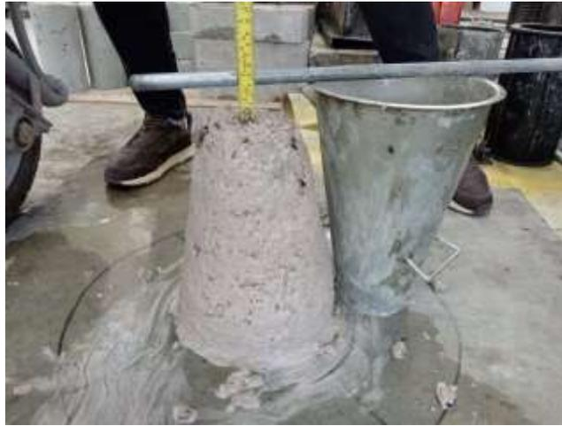
Fig. (3-12) Slump test
