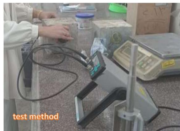
Fig. (3-17) Ultrasonic device and test method
