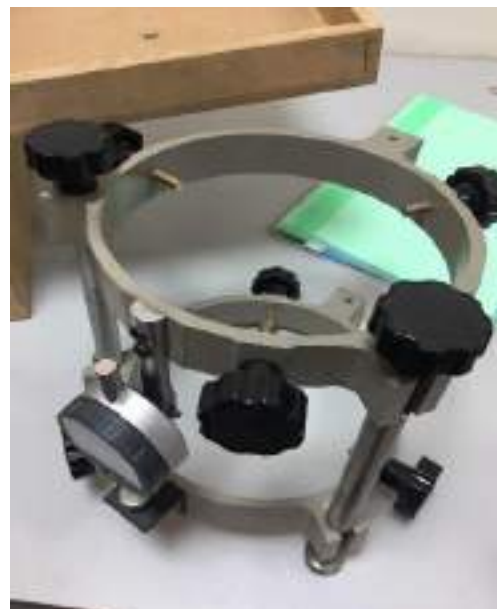
Plate (3.8) Concrete modulus of elasticity test.
