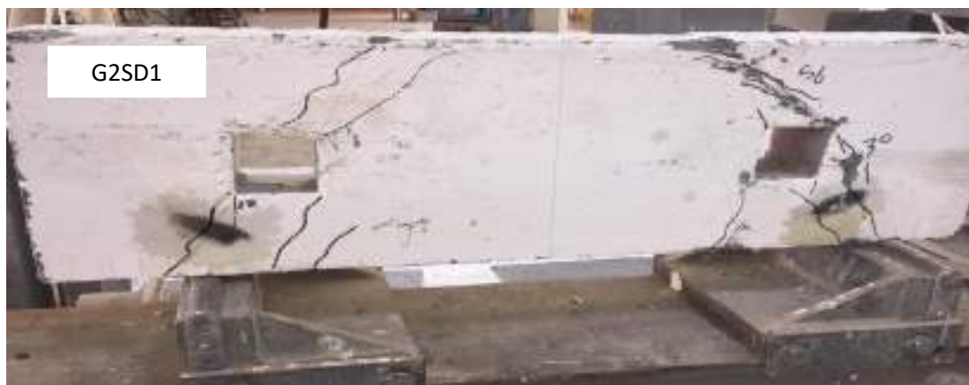
Plate (4.33a) Experimental Deep beam (front view) G2SD1 (9%SF) after failure.
