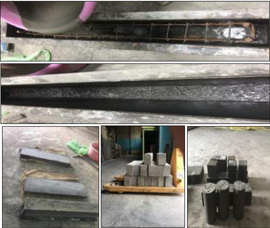
(Plate 3.15) a: Silica fume mix with cement b: Silica fume and cement mix with sand
