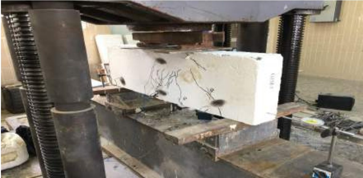
Plate (4.8) Experimental deep beam (G1SE1) after failure.
