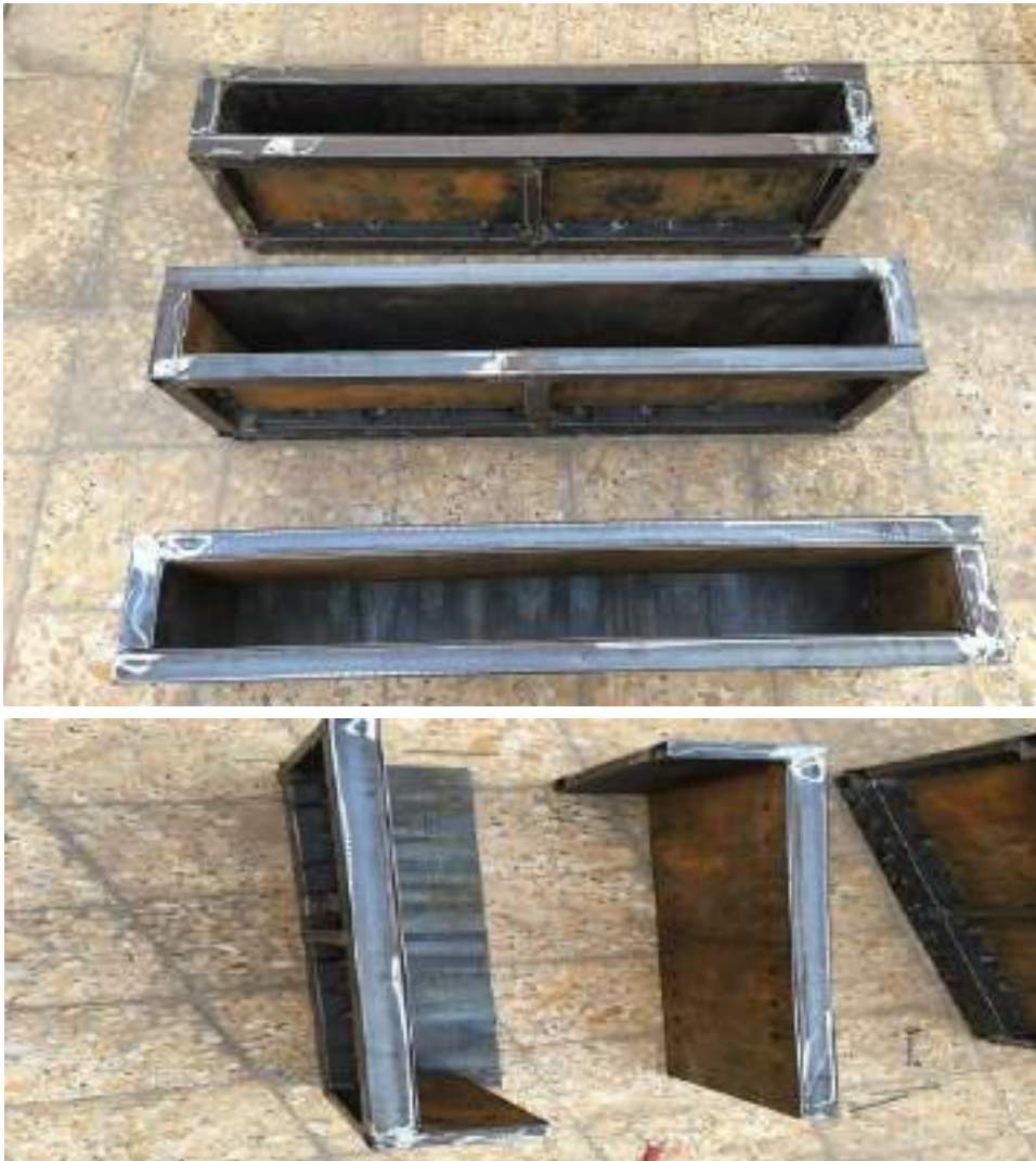
Plate (3.17) Steel molds used for fabrication of deep beams.
