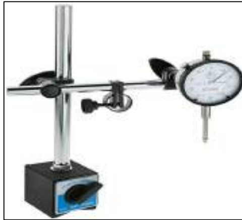
Plate (3.21) Dial gauge used for deflection measurements.
