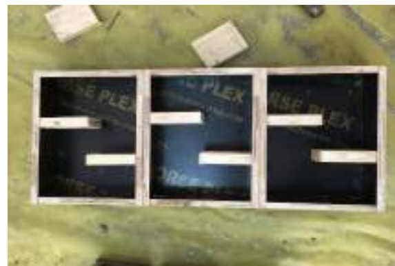
Plate (3.11) Details of double L shear specimen, mold and tests specimens.
