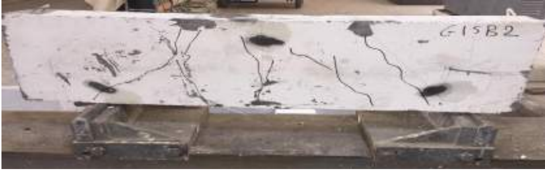
Plate (4.3) Experimental deep beam G1SB2 (7.5%) after failure.
