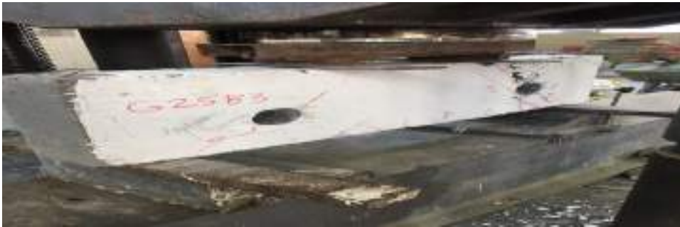
Plate (4.12) Experimental Deep beam SB3 (9%SF) after failure.
