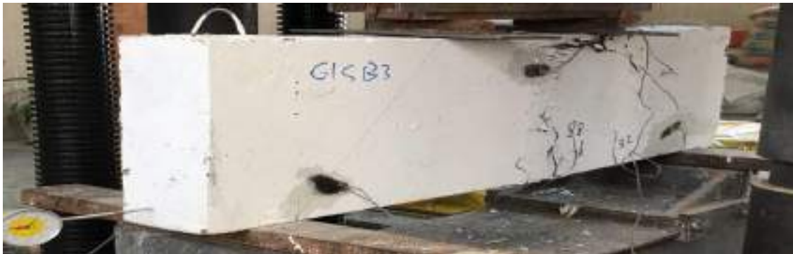
Plate (4.4) Experimental deep beam G1SB3 (9%) after failure.
