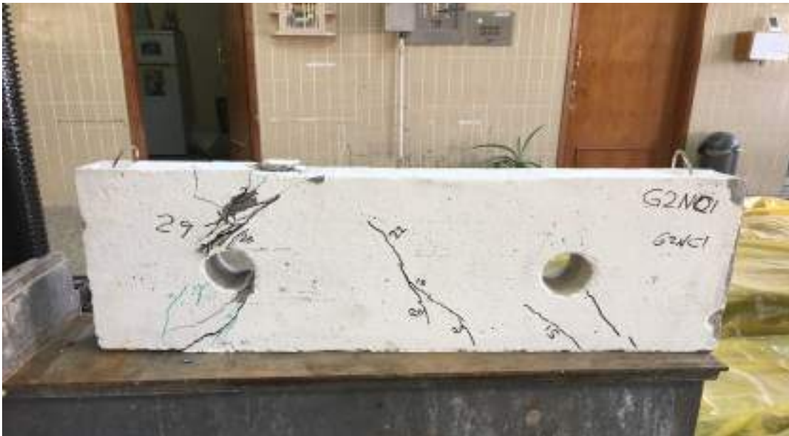
Plate (4.13) Experimental Deep beam G2NC1 (0%SF) after failure.
