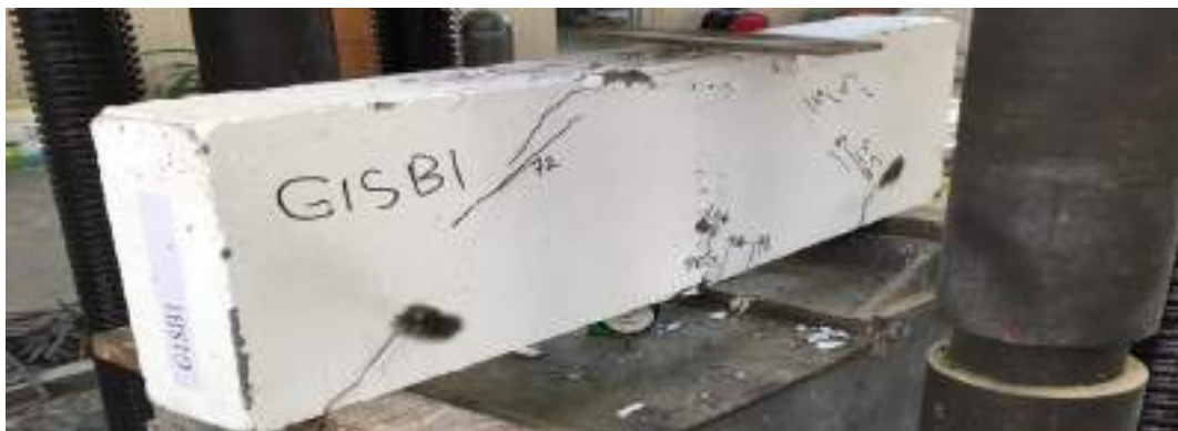
Plate (4.2) Experimental deep beam G1SB1 (6%) after failure.
