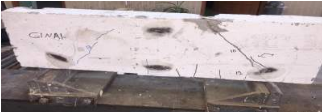
Plate (4.1) Experimental Deep beam G1AN1 (0%SF) after failure.
