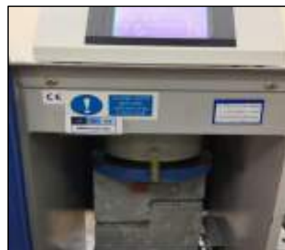
Plate (3.5) Casting and testing of sifcon specimens
