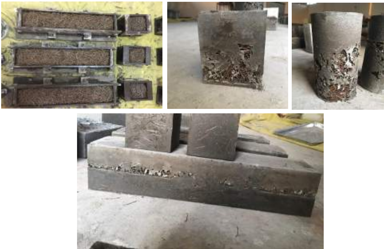
Plate (3.6) Failed samples due to the lack of fluidity of slurry.
