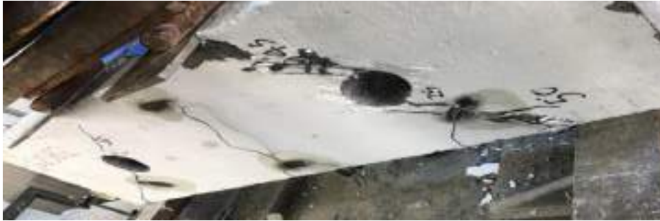
Plate (4.11) Experimental Deep beam G2SB2 (7.5%SF) after failure.
