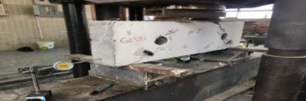
Plate (4.10) Experimental Deep beam G2SB1 (6%SF) after failure.
