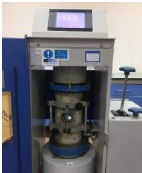
Plate (3.8) Concrete modulus of elasticity test.
