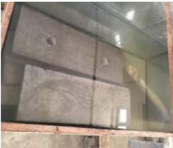
Plate (3.19) Curing of specimens
