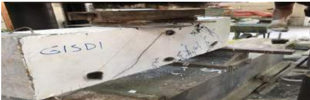
Plate (4.6) Experimental deep beam (G1SD1) after failure.
