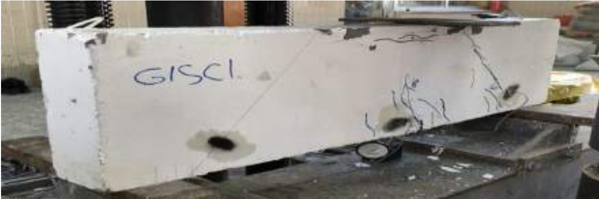
Plate (4.5) Experimental deep beam G1SC1 after failure.
