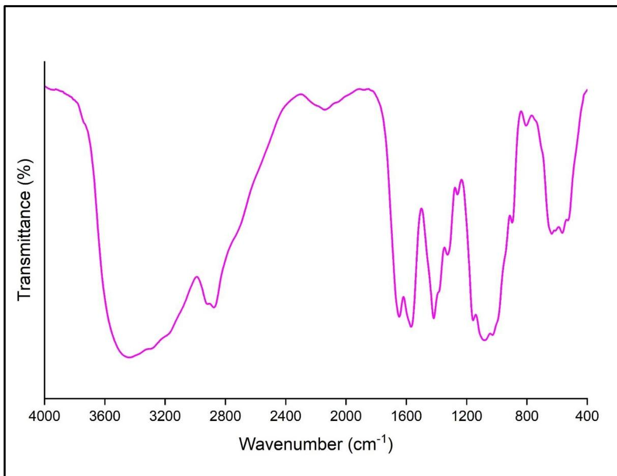
**Figure 3-2** FT-IR spectra of Pure Chitosan (Chi)
