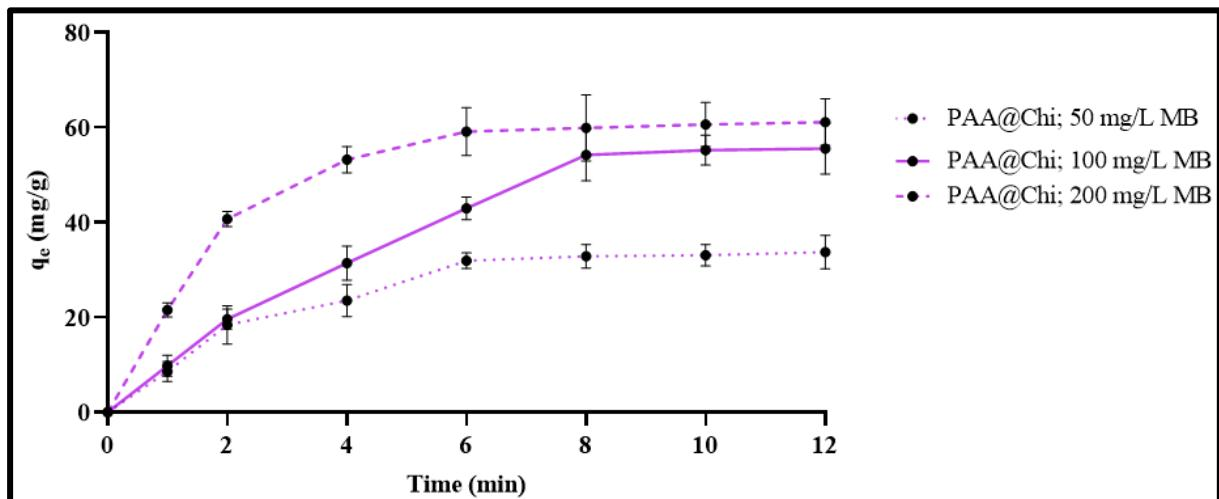
Figure 3-16 Effects of MB Solution Concentrations
