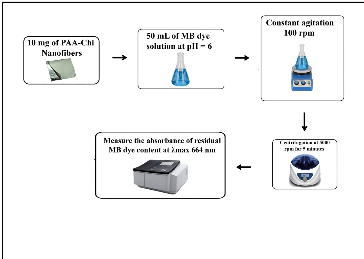
**Figure 2-2** Flow diagram of methylene blue adsorption experiment
