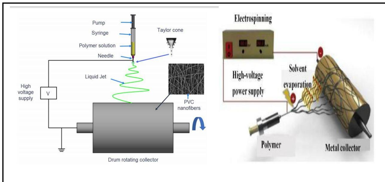
**Figure 1-3** Schematic setup illustrations for the electrospinning process [29].
