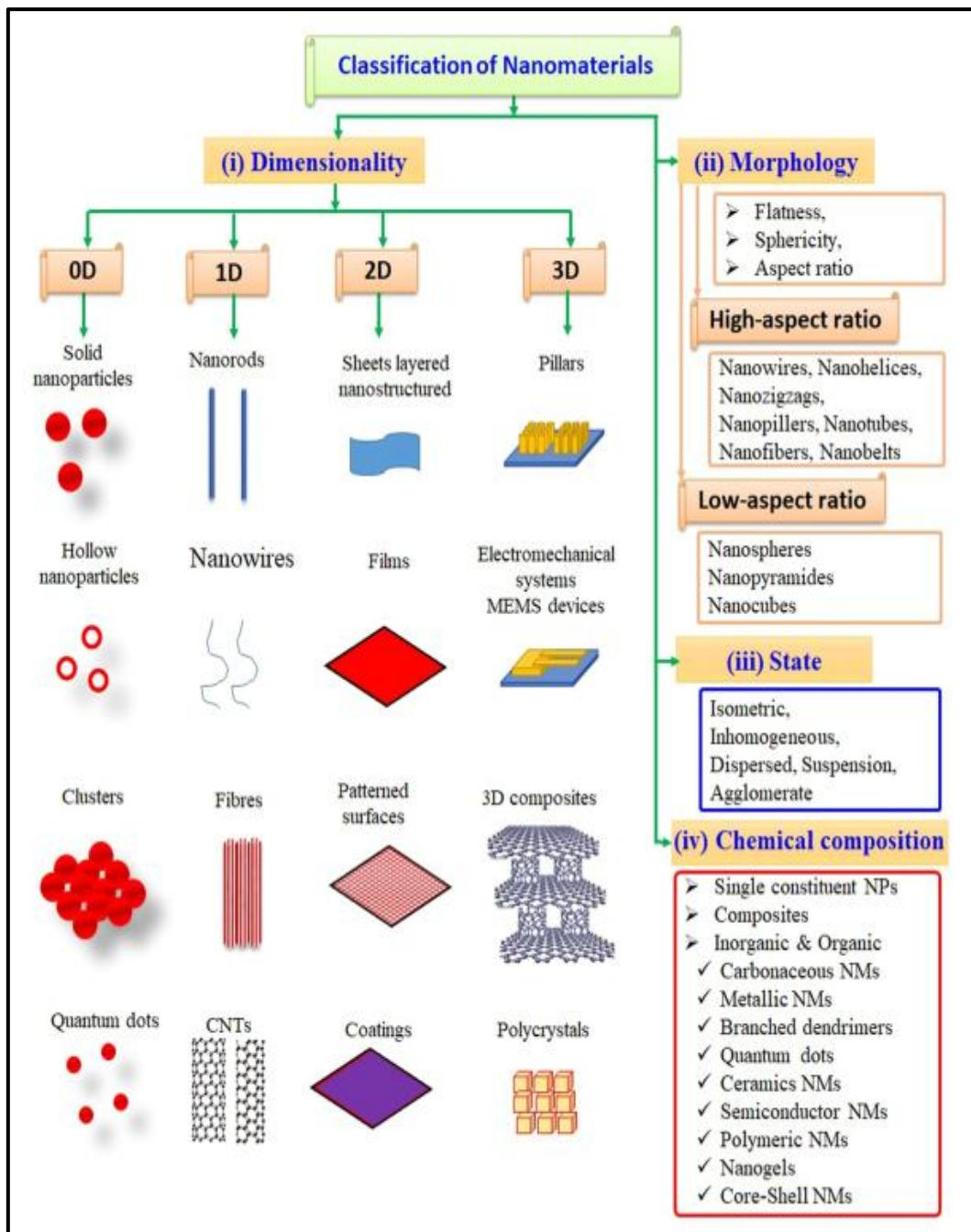
**Figure 1-1** Schematic illustration of the classification of nanomaterials based on different criteria [7].
