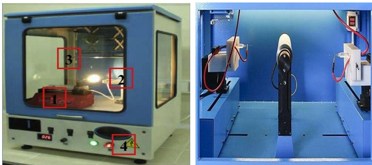
**Figure 1-2** Electrospinning equipment: 1 is the syringe pump, 2 is the tip of the needle and where the voltage is applied, 3 is the collector plate, and 4 is the power supply [20]
