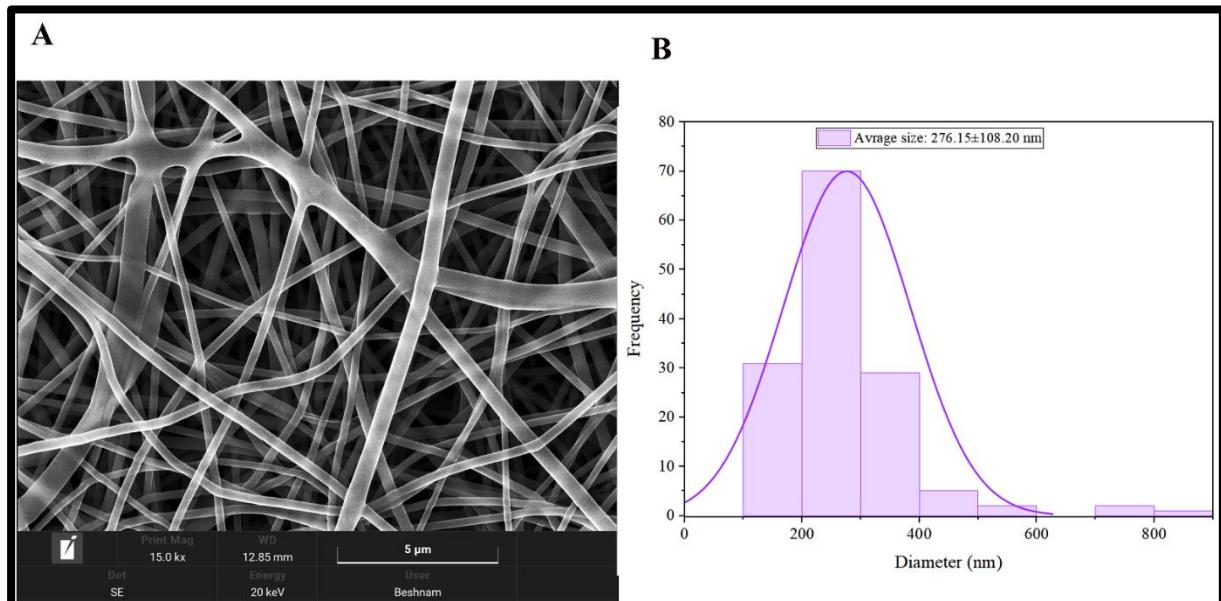
**Figure 3-4** FESEM images of the PAA–Chi nanofibers along with histograms of their diameter distributions (A,B).
