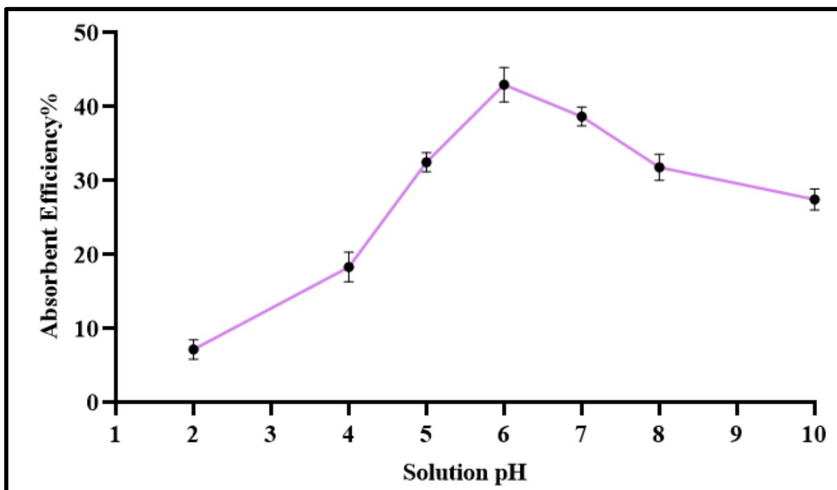
**Figure 3-15** Effects of MB Solution pH
