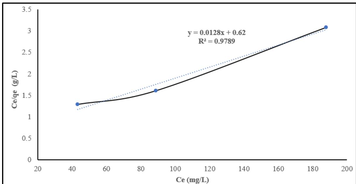
**Figure 3-19** The Adsorption Isotherms (Langmuir model)
