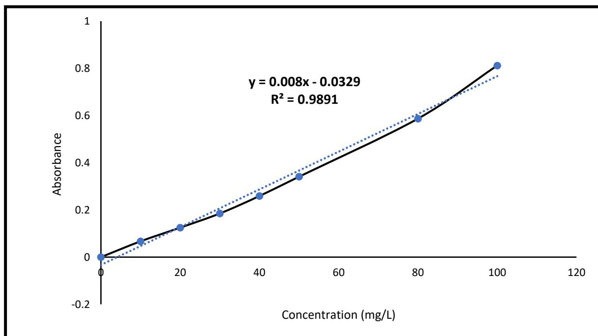
**Figure 3-8** The Standard Calibration Curve for Methylene Blue Dye
