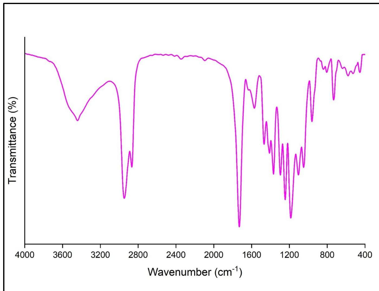
**Figure 3-1** FT-IR spectra of pure Polyacrylic Acid (PAA)
