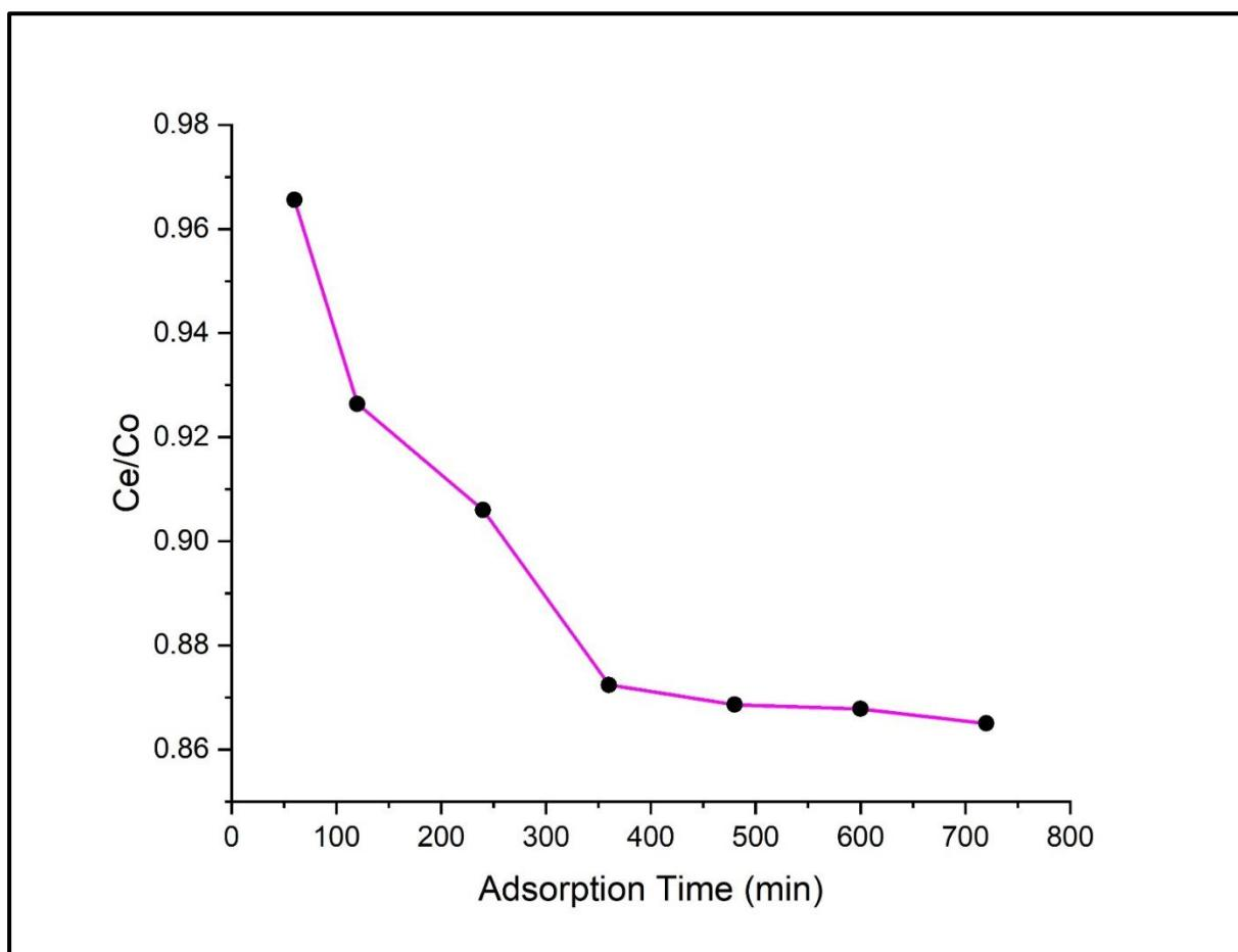
**Figure 3-10 Adsorption efficiency of MB dye (50 mg.L-1) by PAA-Chi Nanofibers**
