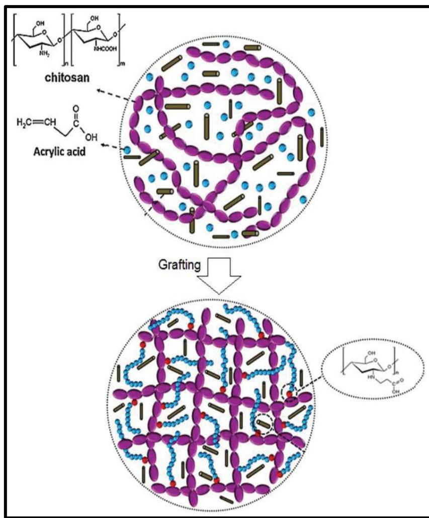
**Figure 1-8** Synthesis of poly(acrylic acid)-grafted chitosan incorporating cellulose nanofibers [106]
