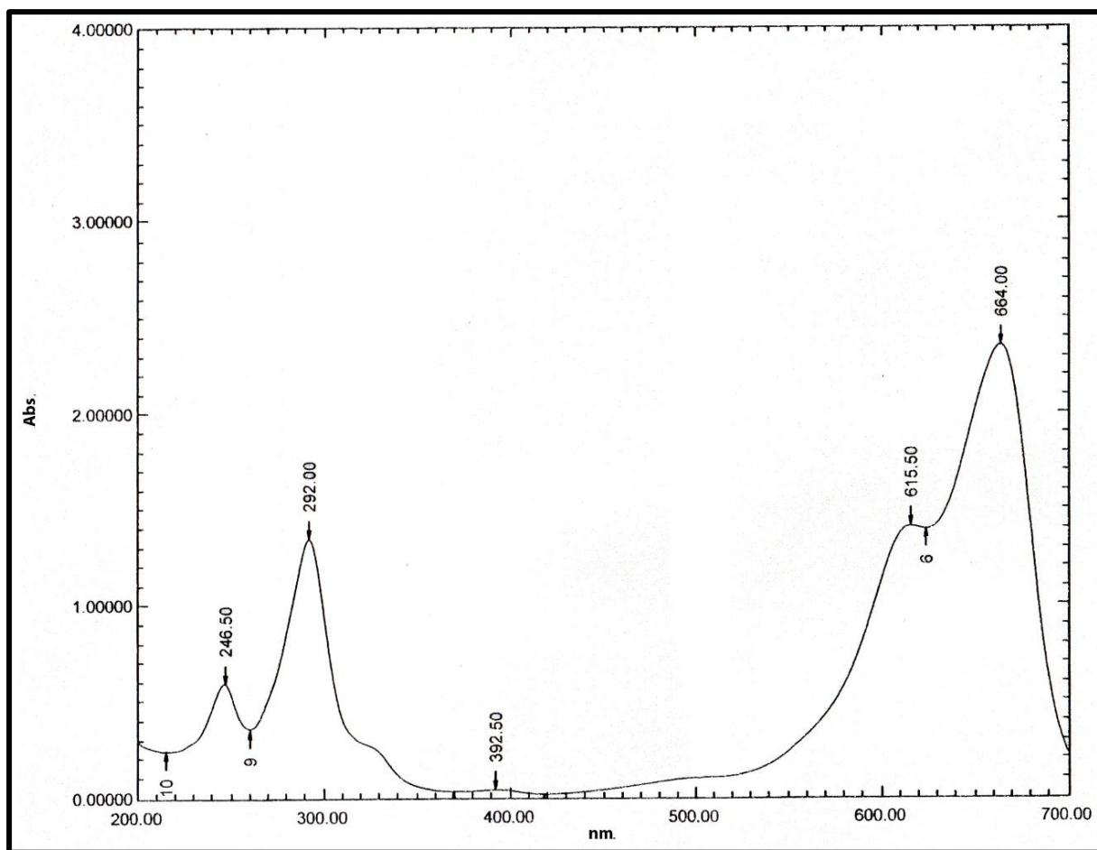
**Figure 3-9** Absorption spectrum of MB dye
