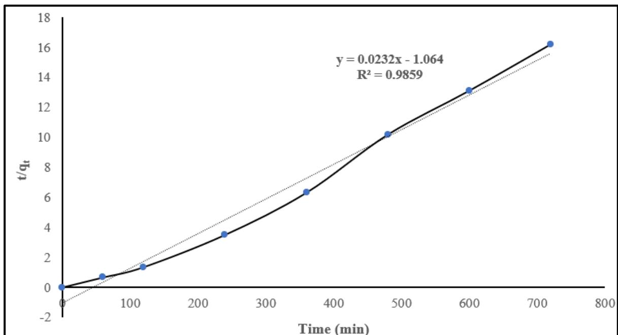
**Figure 3-18** The pseudosecond order was employed to analyze the adsorption kinetics of MB dye onto PAA-Chi NFs. The black line denotes the primary findings, whereas the blue line signifies the anticipated outcomes.
