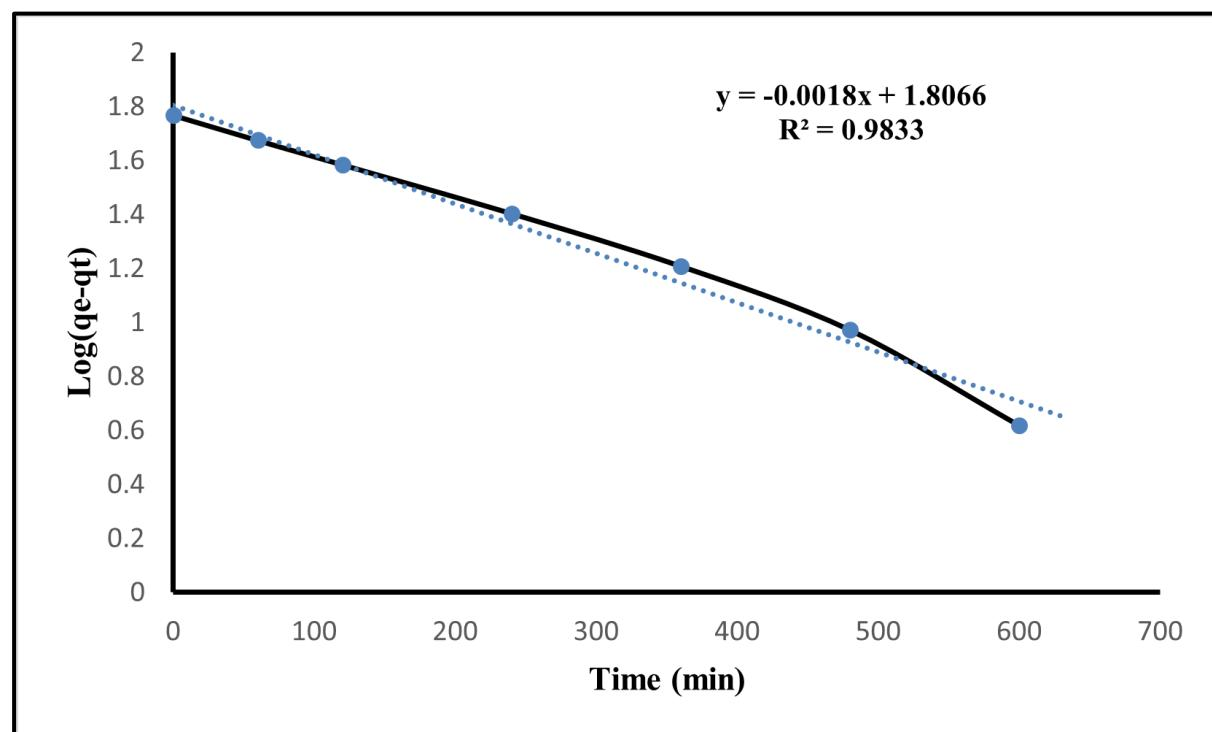
**Figure 3-17** The pseudofirst order was employed to analyze the adsorption kinetics of MB dye onto PAA-Chi NFs. The black line denotes the primary findings, whereas the blue line signifies the anticipated outcomes.
