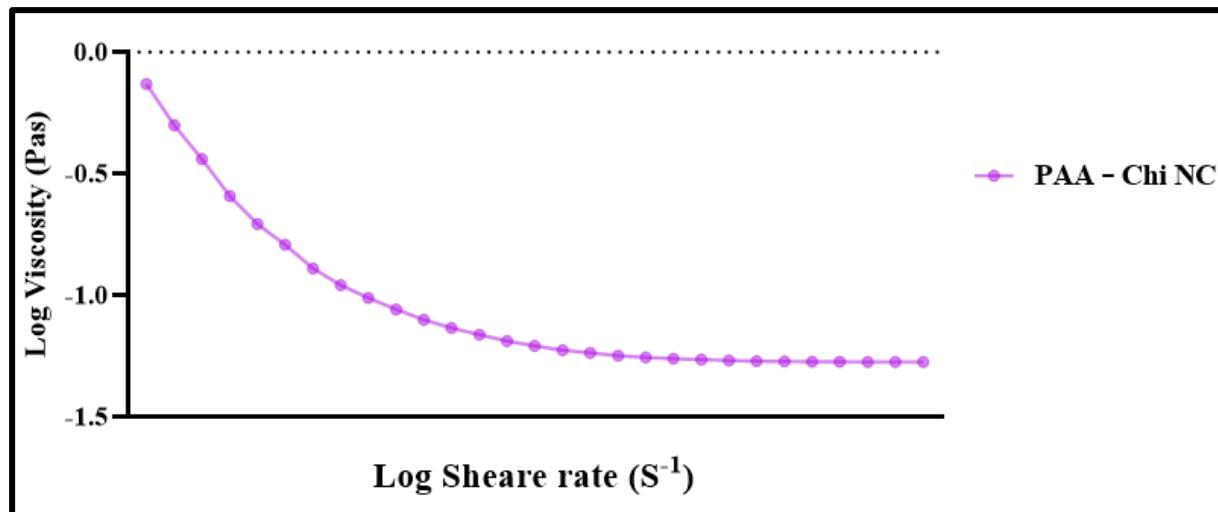
**Figure 3-7** Apparent viscosity (Pa) in terms of shear rate ( $S^{-1}$ ) for the PAA-Chi NFs
