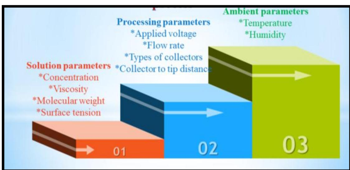
**Figure 1-4** The different parameters affecting the electrospinning process [34].
