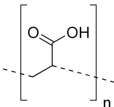
**Figure 1-7** Chemical structure of Polyacrylic acid
