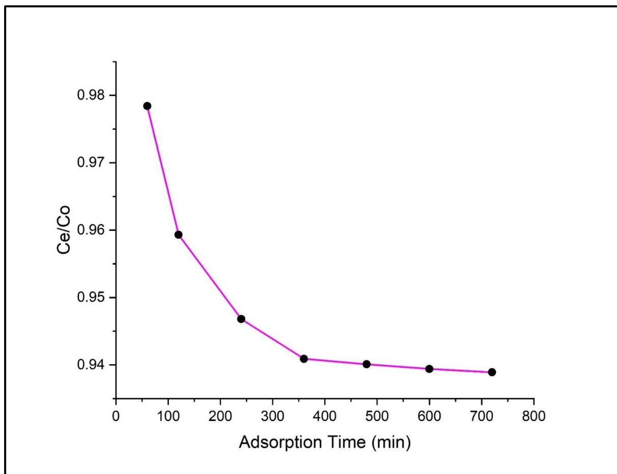
**Figure 3-12 Adsorption efficiency of MB dye (200 mg.L-1) by PAA-Chi Nanofibers**
