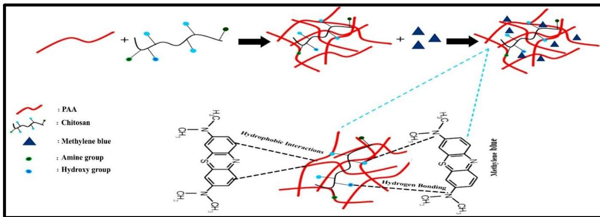
**Figure 3-13** The adsorption mechanism of nanofibers (PAA-Chi)[171].
