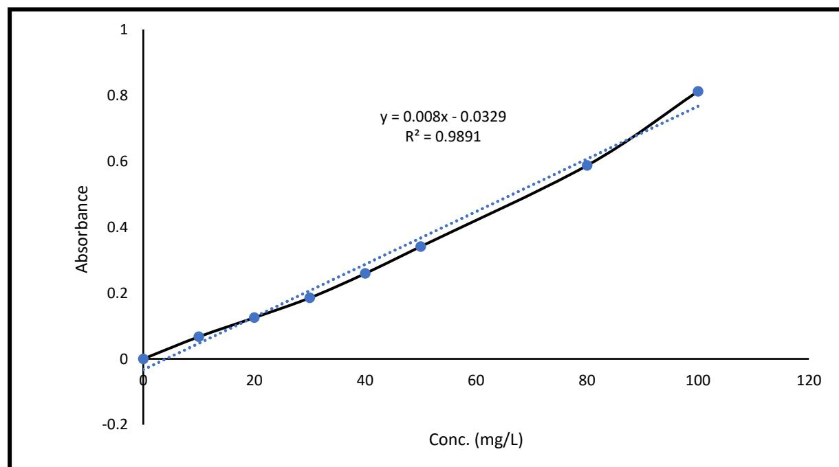
**Figure 2-1** Standard calibration curve for MB dye at 664 nm.
