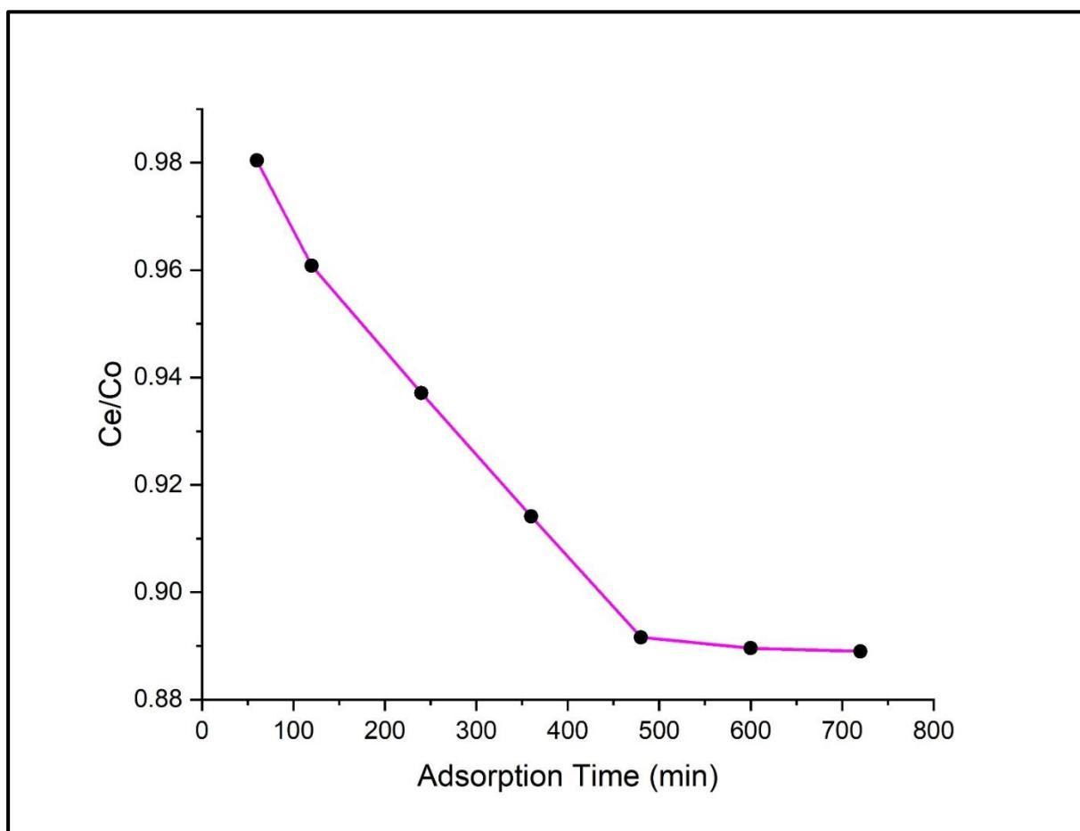
**Figure 3-11 Adsorption efficiency of MB dye (100 mg.L-1) by PAA-Chi Nanofibers**
