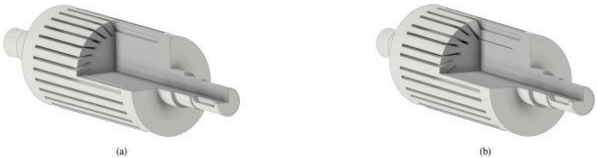
Fig.2.6. ASSR with axial slits skewed in tangential and axial directions: (a) equal slits depth and (b) various depths of slits, [59].
