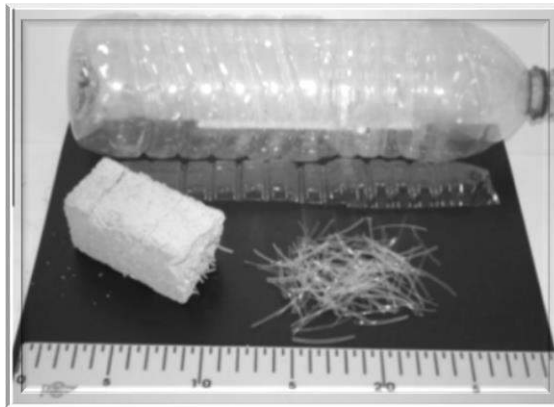
Fig. (2-20): Form of PET Bottle Used for Fiber Reinforcement.
