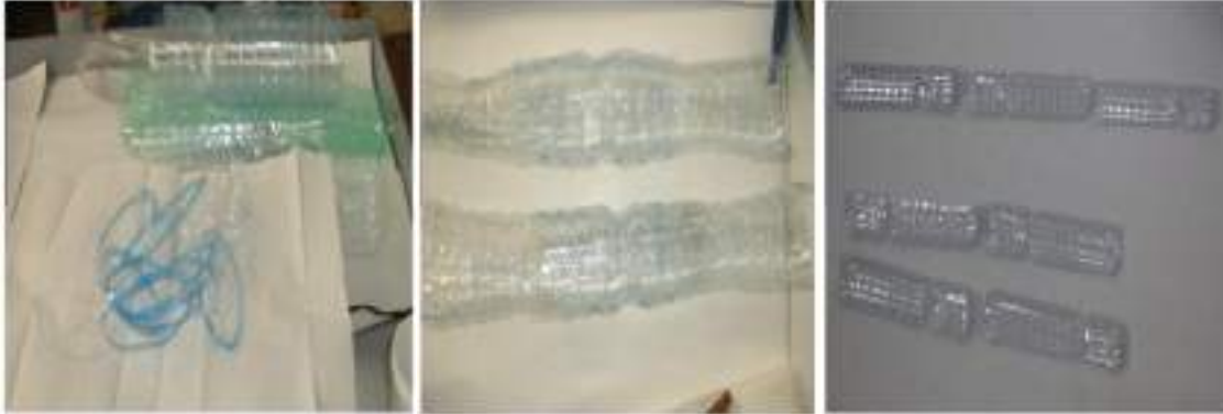
Fig. (2-24): Forms of PET used (Circular fibers, half bottles, and strips).
