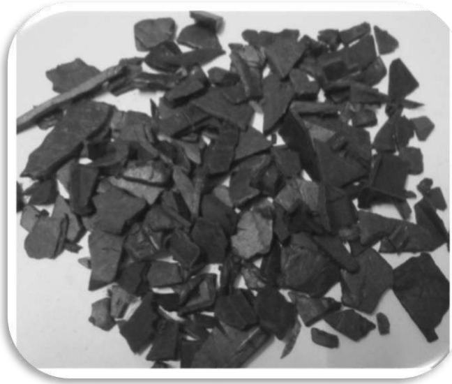
Fig. (2-2): Form of E- plastic waste after cutting.
