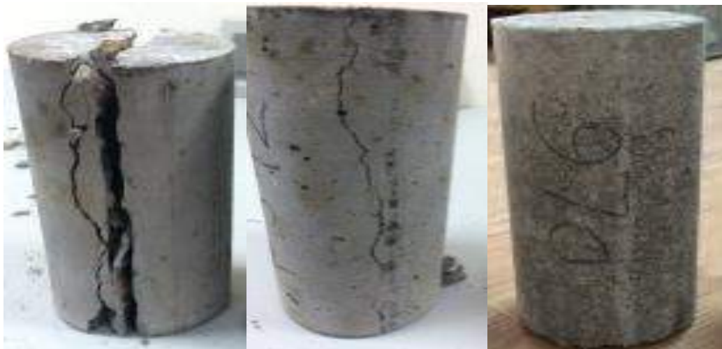
Fig. (4-8): Result of Split Tensile Strength for plastic waste
