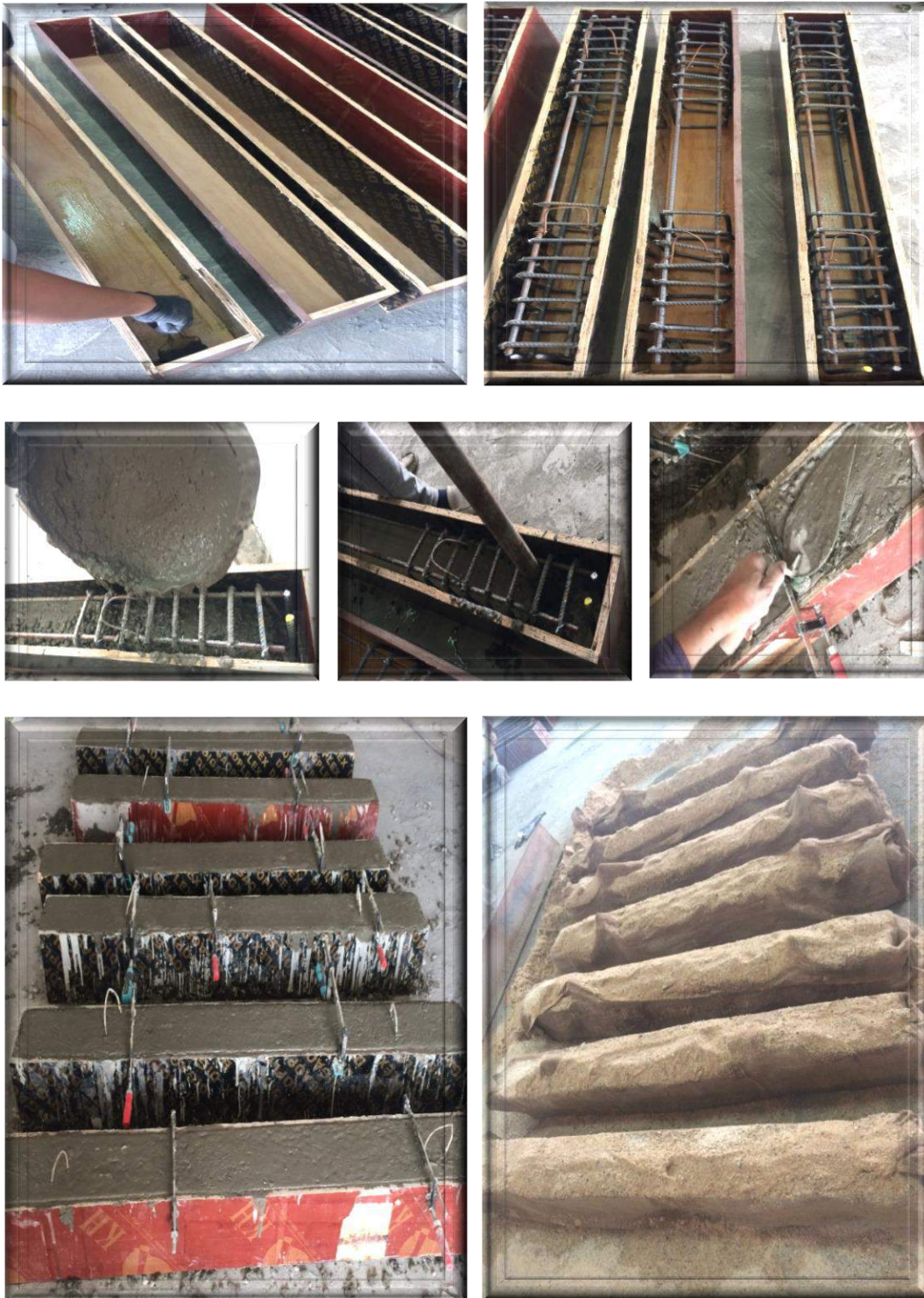
Fig. (3-18): Casting and curing of beams.
