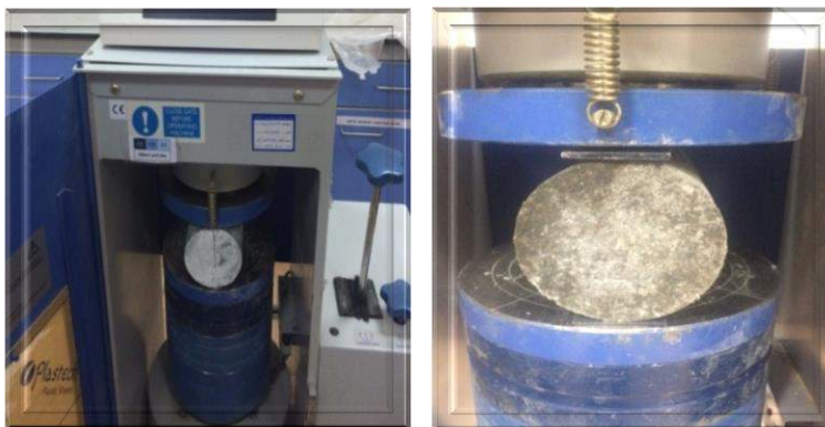
Fig. (3-21): Split tensile strength Test.
