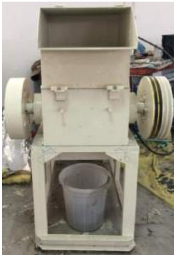
Fig. (3-9): Machine used to cut plastic waste a) Side view b) Internal composition of the machine.
