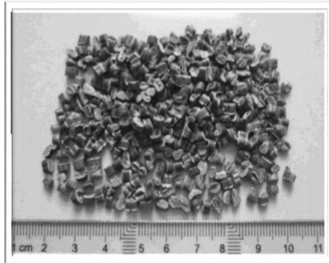
Fig. (2-4): Form of polypropylene (PP) after cutting.
