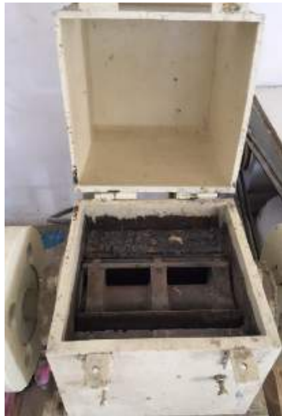
Fig. (3-9): Machine used to cut plastic waste a) Side view b) Internal composition of the machine.
