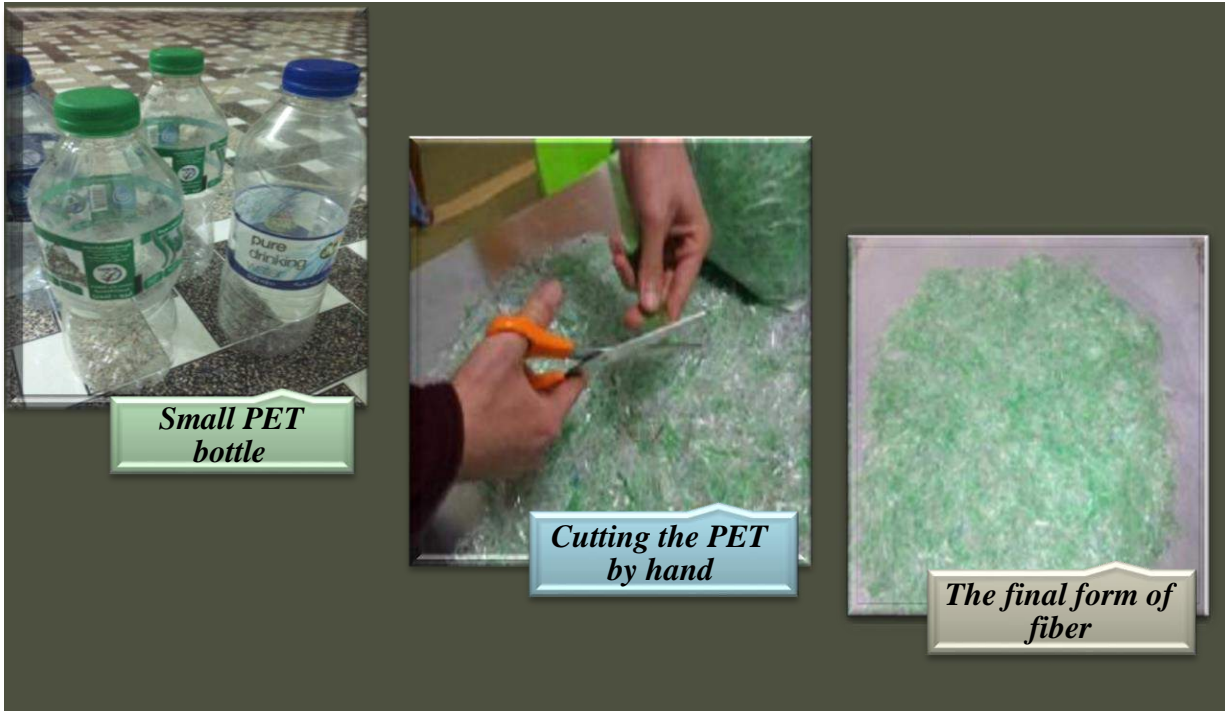
Fig. (3- 12): Steps to prepare the particles of regular hand PET fiber.
