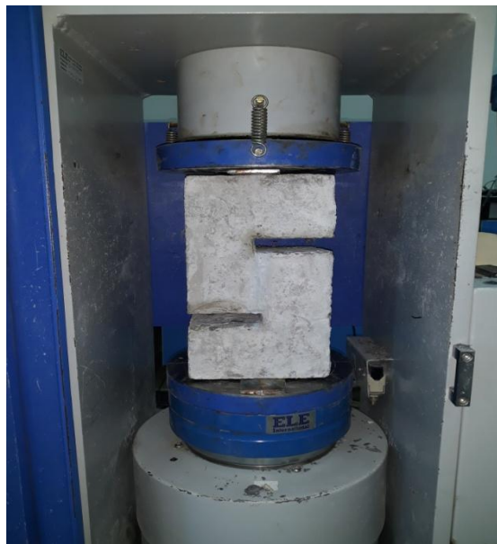
Fig. (3-12): Shear test method
