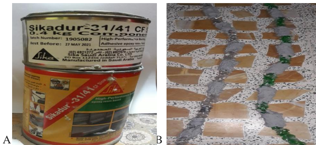
Fig. (3-1): A-High performance building adhesive epoxy. B- Using epoxy as knots along PET bars
