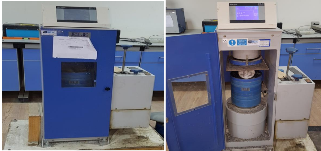
Fig. (3-10): Splitting tensile test
