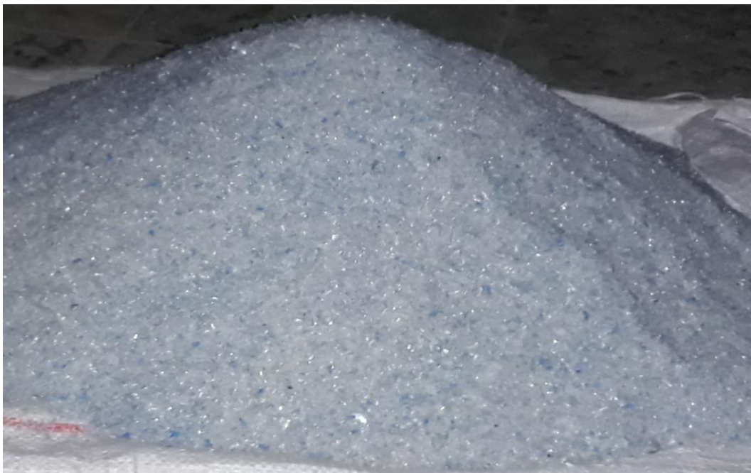
Fig. (3-2): PET molecules produced by chopping water bottles and soft drinks
