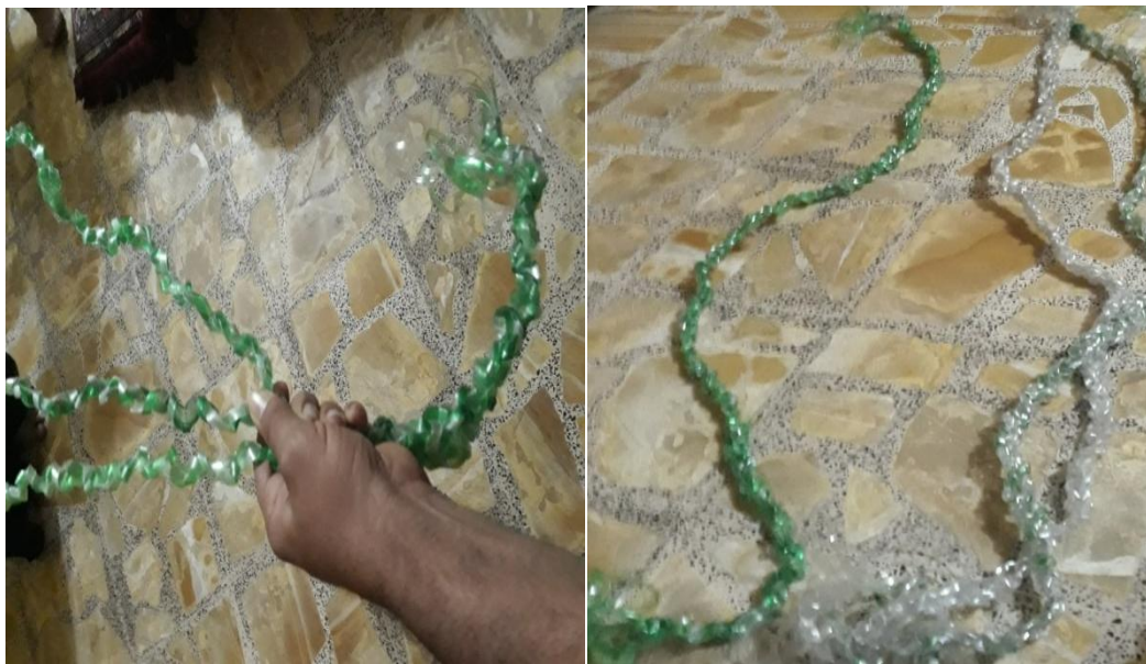
Fig. (3-22): Main braid forming method 36 strips (3secondary braids)
