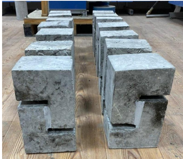
Fig. (4-8): Shear test double L- shape specimens for PET percentages as a sand replacement
