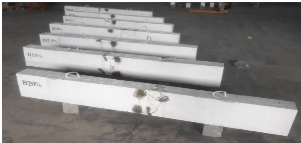
Fig. (4-22): Reinforced concrete Beam specimens for all PET/Sand percentages
