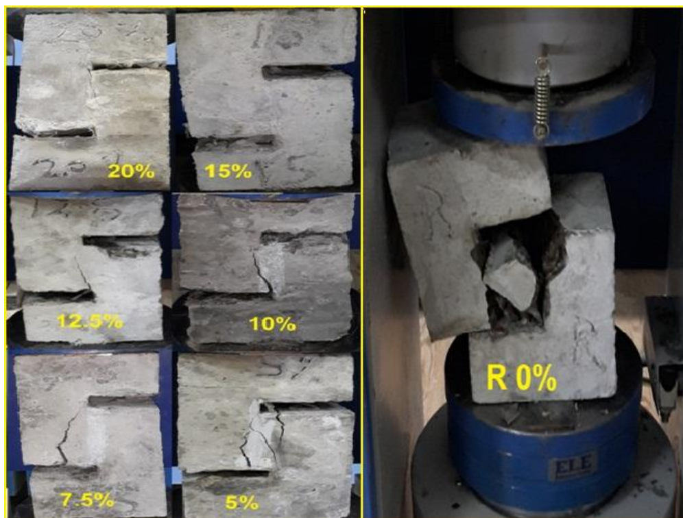
Fig. (4-10): Failure mode of double L- shape concrete specimens for PET percentages as a sand replacement
