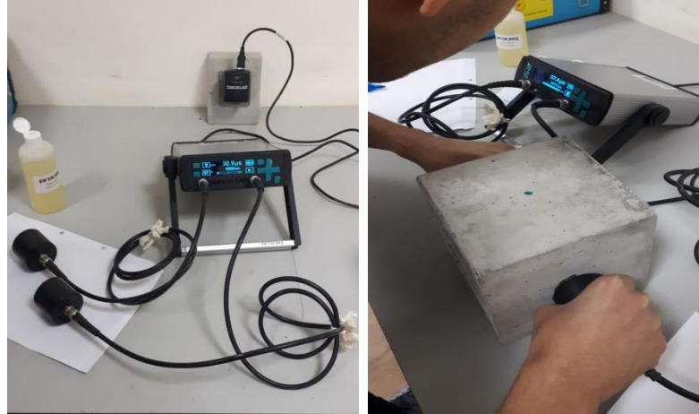
Fig. (3-14): Ultrasonic device and test method
