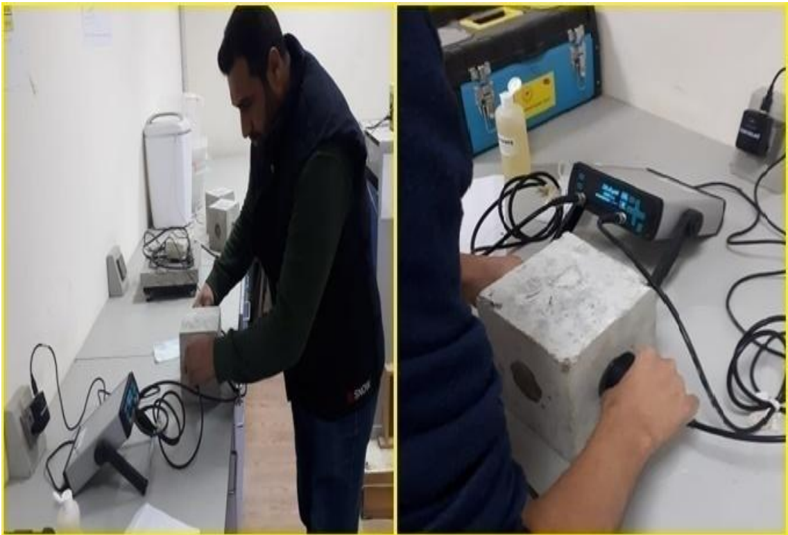
Fig. (4-17): Ultrasonic testing method
