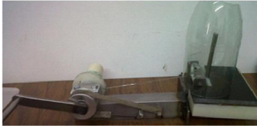
Fig. (2-16): Device used to obtain recycled PET fibers [38]
