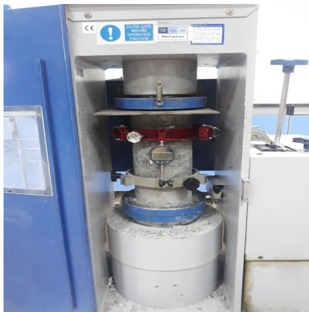
Fig. (3-15): Modulus of elasticity and energy absorption tests
