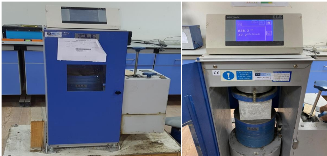
Fig. (3-9): Compression machine test
