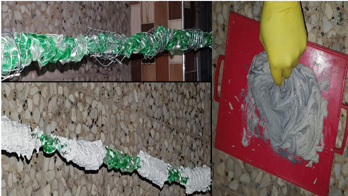
Fig. (3-35): Forming BP2 braids procedure
