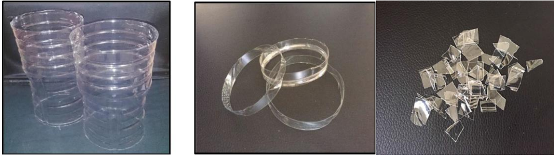
a- Ring shape PET fiber b- Irregularly shaped PET particles Fig. (2-4): The PET waste fibers types [21]
