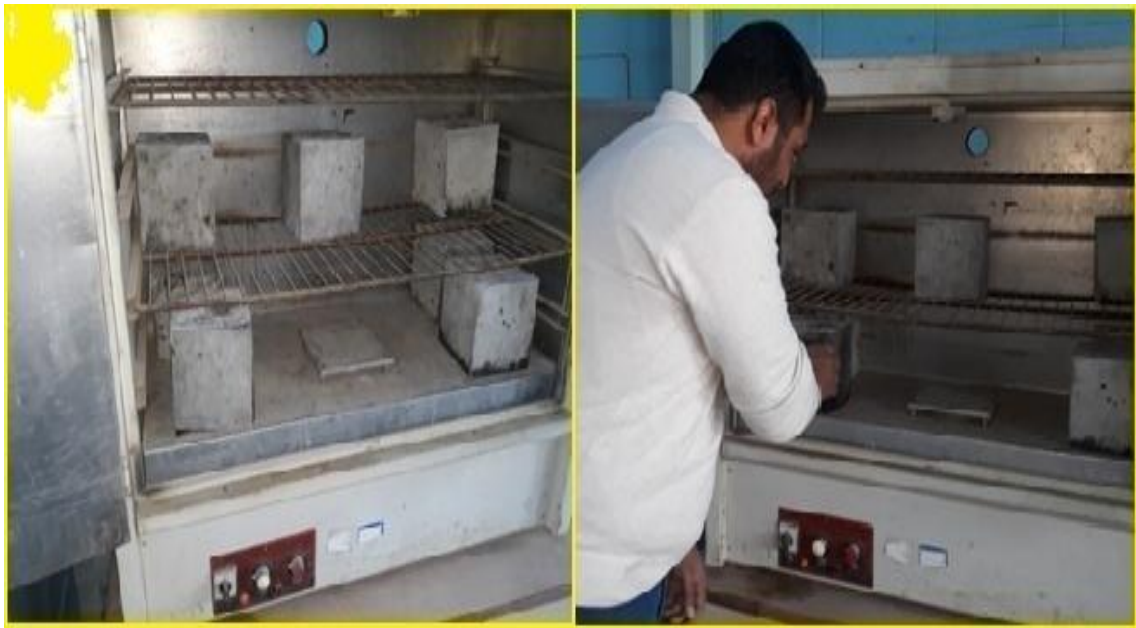
Fig. (4-15): Drying the Specimens of absorption test in the oven
