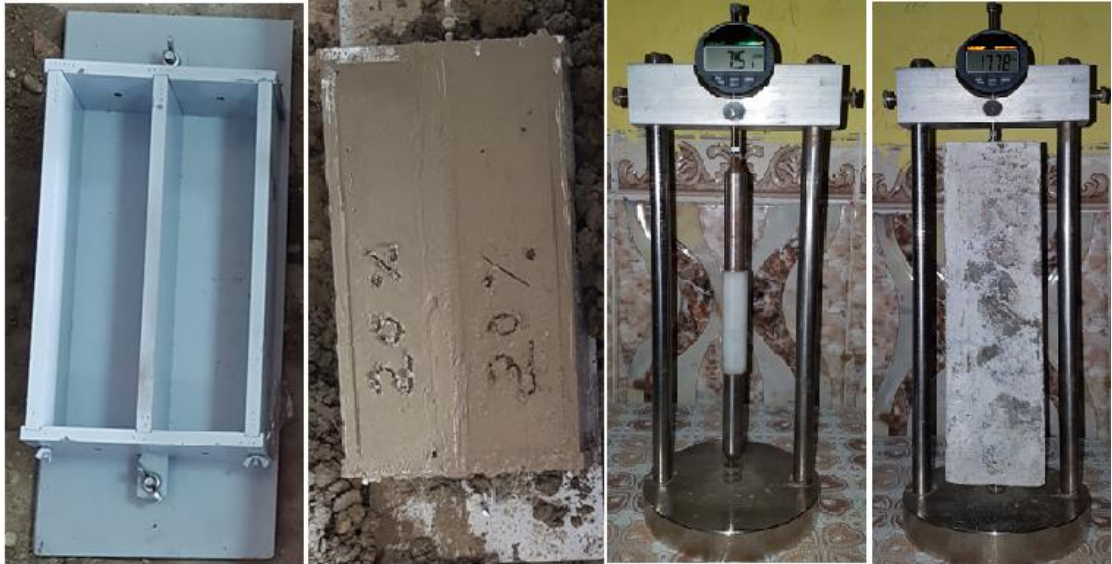
Fig. (3-13): Shrinkage specimens and test method
