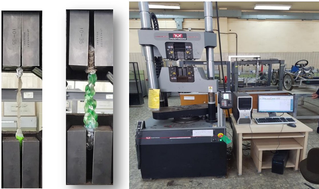
Fig (3-26): Braid and strips tensile testing machine
