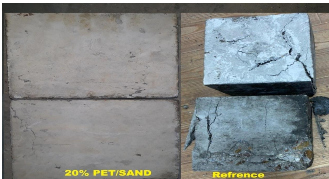
Fig. (4-2): Concrete cubes failure modes for reference cube and 20% (PET/Sand) percentage
