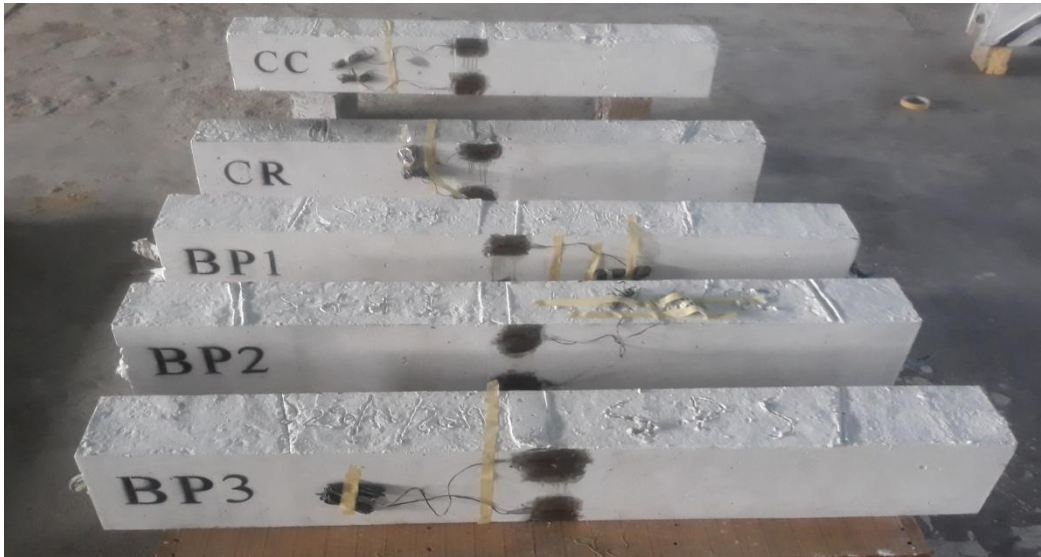
Fig. (4-36): Beams specimens for the part of replacing main reinforcement by PET bars
