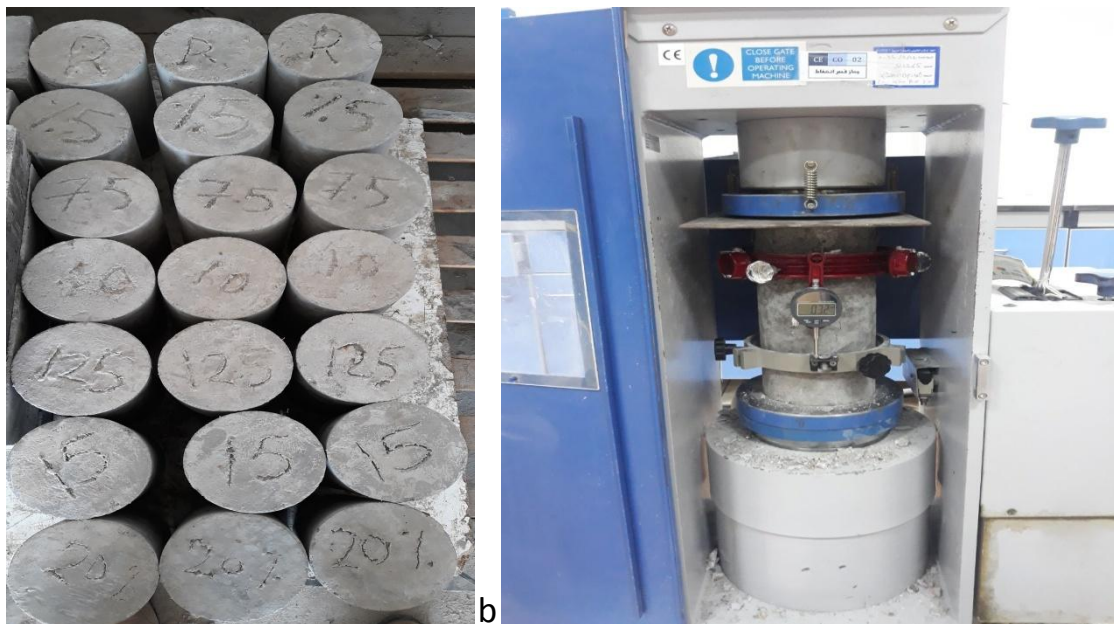
Fig. (4-18): a- Modulus of elasticity and energy absorption specimens. b- Modulus of elasticity test.
