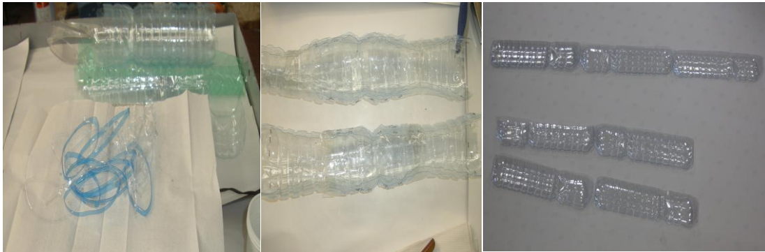
(a) Circular PET fibers (b) Half bottle reinforcement (c) PET strips utilized in test 2. Fig. (2-14): PET bottle waste samples [37]
