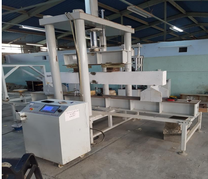
Fig. (3-18): Automatic compression machine
