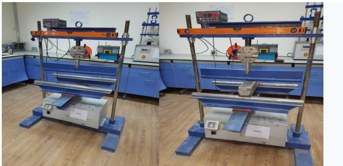
Fig. (3-11): Flexural strength test
