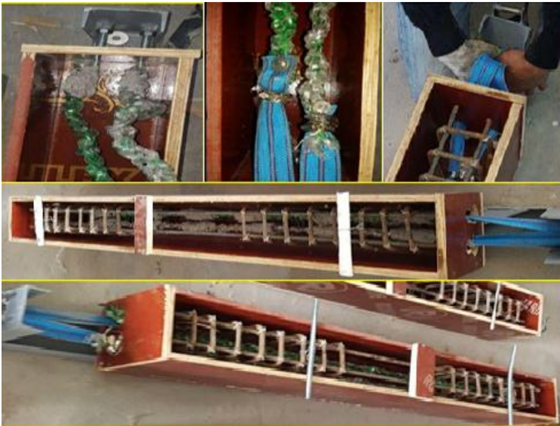
Fig. (3-34): Braids tightening method and installation to the pre tension tool procedure
