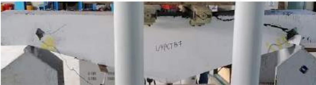
Fig. 4-38 Crack pattern at failure of TB 7.
