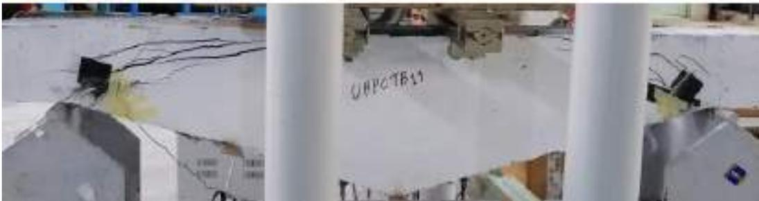
Fig. 4-50 Crack pattern at failure of TB 19.
