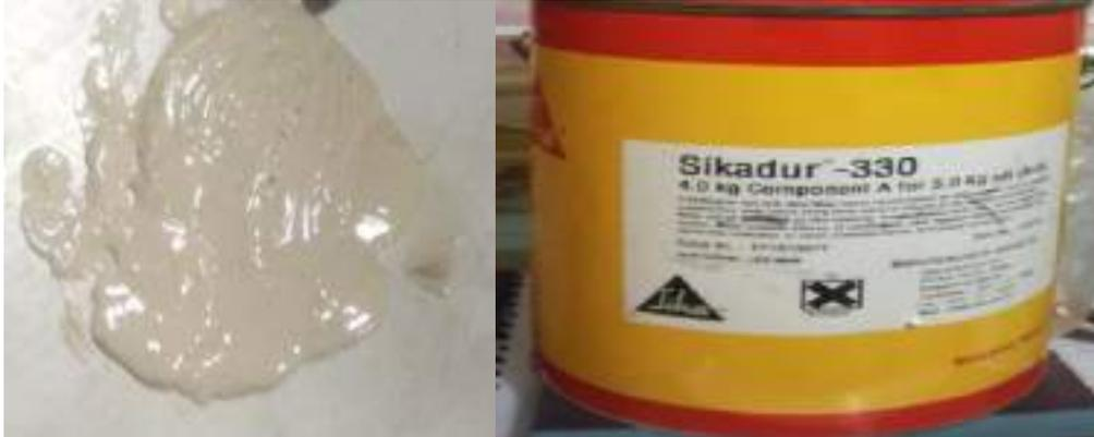
Fig. 3-21 Component A of Sikadur-330.
