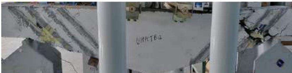
Fig. 4-43 Crack pattern at failure of TB 12.
