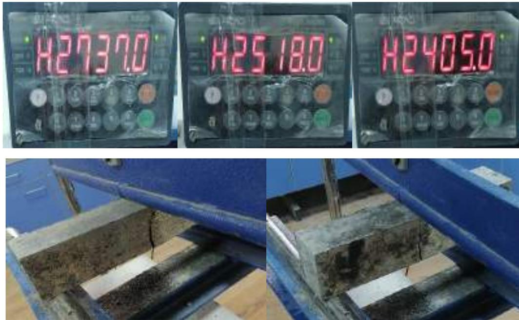
Fig. 4-1 Results of modulus of rupture for prism.
