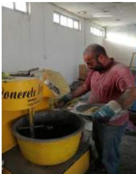
Fig. 3-16 Adding of steel fiber.
