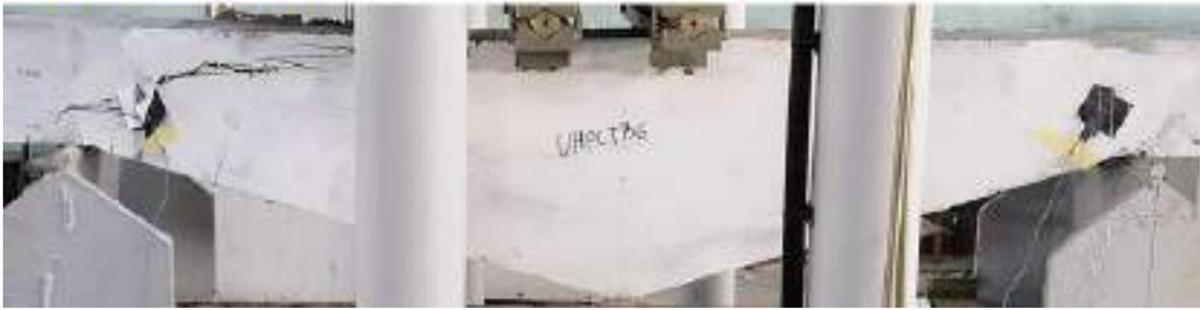
Fig. 4-37 Crack pattern at failure of TB 6.
