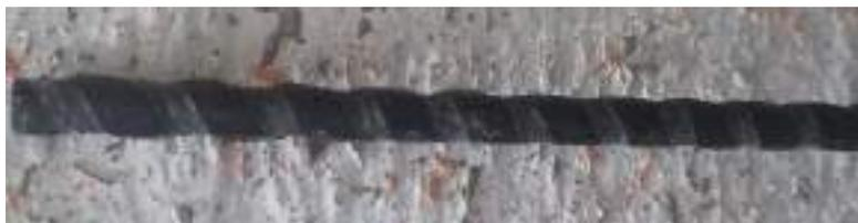
Fig. 3-6 NS CFRP bar (deformed type).
