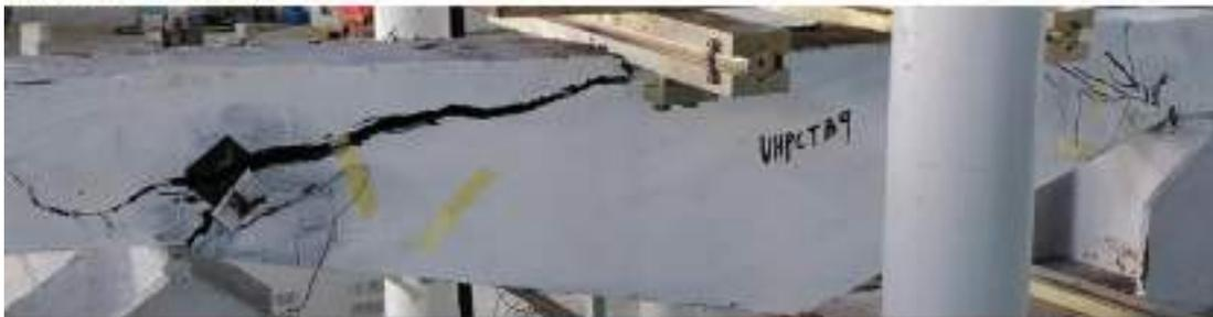
Fig. 4-40 Crack pattern at failure of TB 9.
