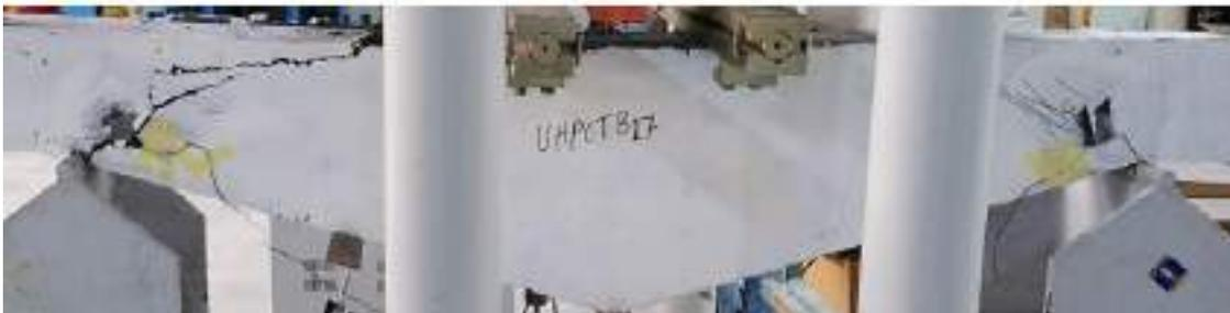
Fig. 4-48 Crack pattern at failure of TB 17.
