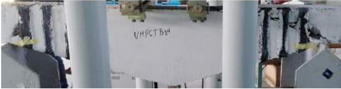
Fig. 4-45 Crack pattern at failure of TB 14.
