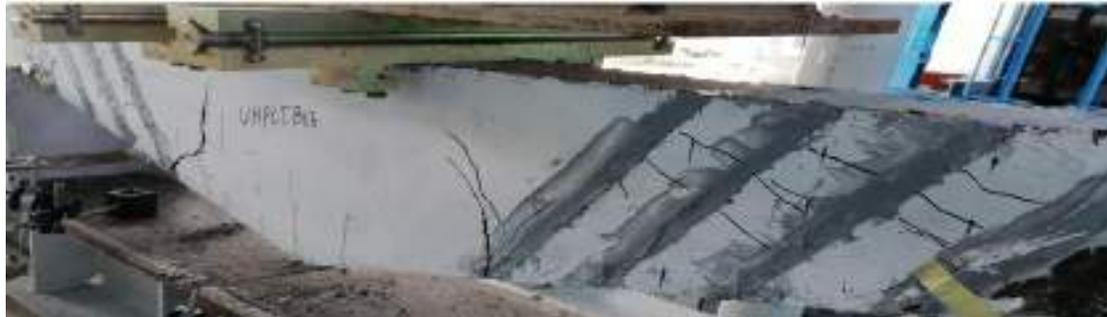
Fig. 4-44 Crack pattern at failure of TB 13.
