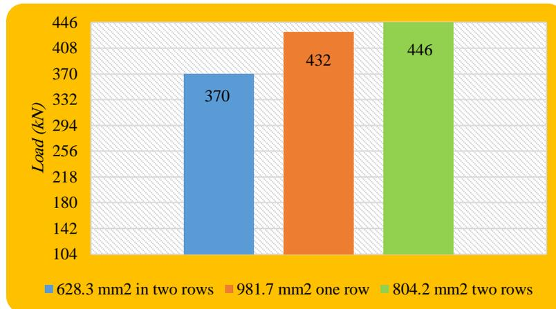
Fig. 4-11 Failure load versus area of tensile bars.
