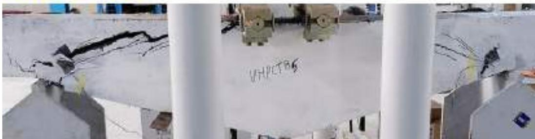
Fig. 4-36 Crack pattern at failure of TB 5.
