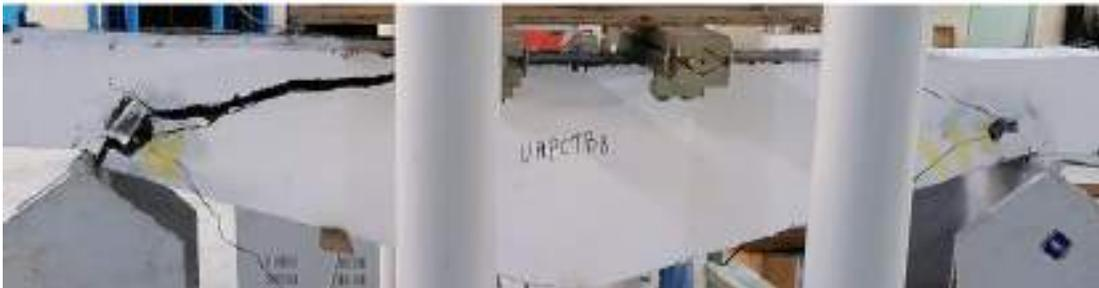
Fig. 4-39 Crack pattern at failure of TB 8.
