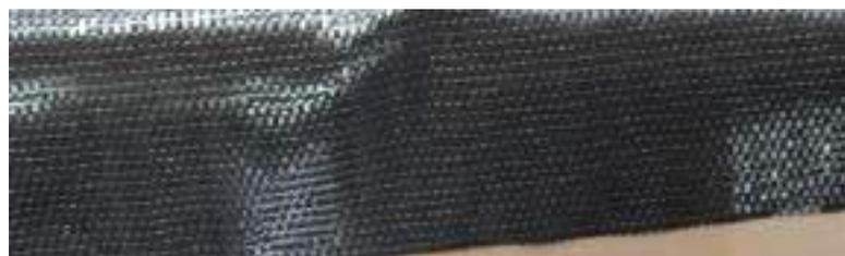
Fig. 3-7 CFRP strip.
