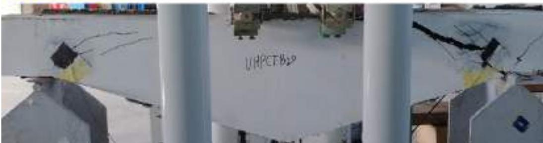
Fig. 4-51 Crack pattern at failure of TB 20.
