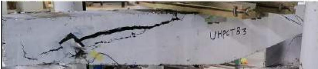
Fig. 4-35 Crack pattern at failure of TB 3.
