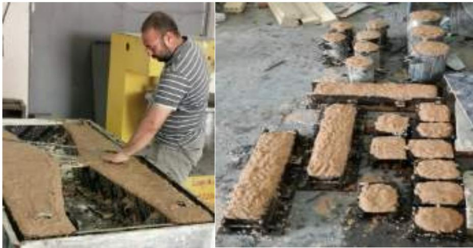
Fig. 3-18 Using of wet sand to cover specimens.
