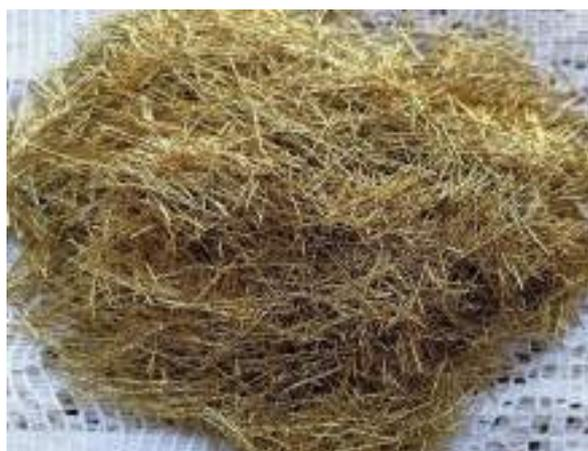
Fig. 3-5 Type of steel fiber.
