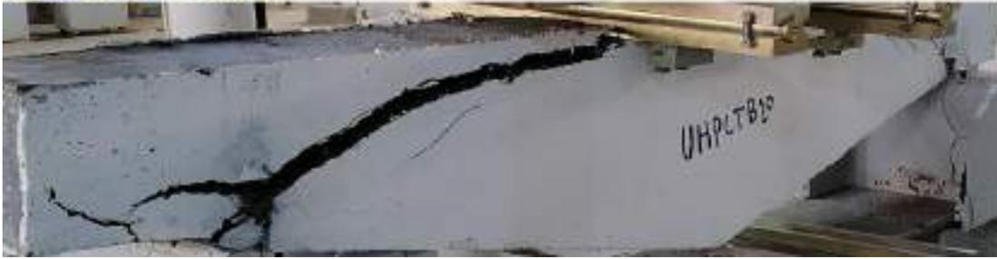
Fig. 4-41 Crack pattern at failure of TB 10.
