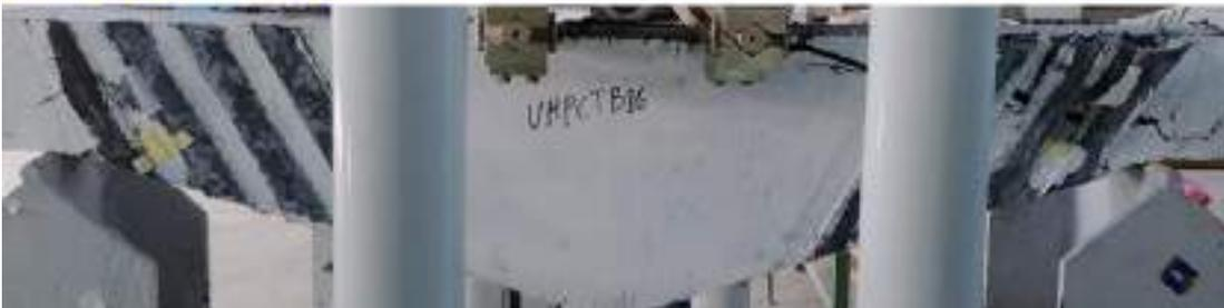
Fig. 4-47 Crack pattern at failure of TB 16.
