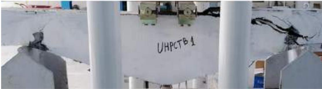
Fig. 4-33 Crack pattern at failure of TB 1.
