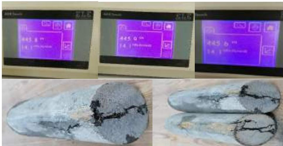
Fig. 4-3 Splitting test result with tensile failure mode.
