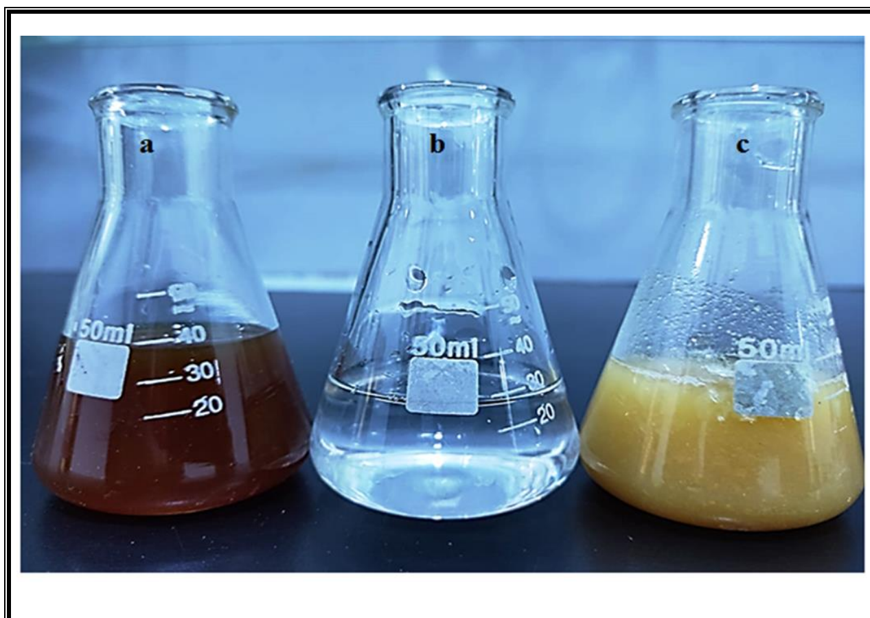
Figure( 3-1). The visual appearance of the synthesized ZnO NPs using C. spinosa L. fruit extract: (a) fruit extract solution; (b) zinc acetate; and (c) mixture of zinc acetate and aqueous fruit extract
