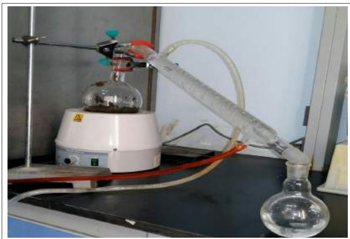
Figure (3-2) hydro distillation technique Clevenger-type apparatus
