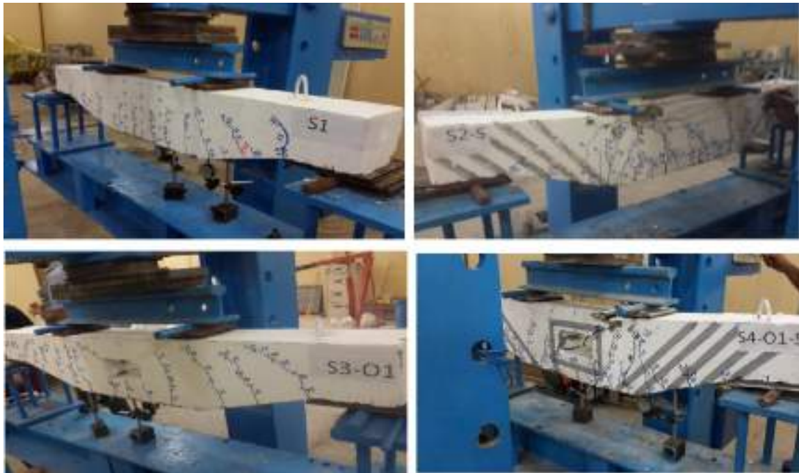
Figure (2-7): Crack Pattern of Shear Beams [33].
