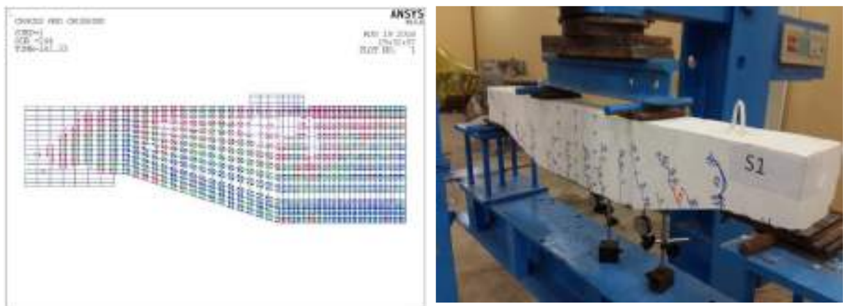
(e) Crack patterns for numerical and experimental beam (S1).
