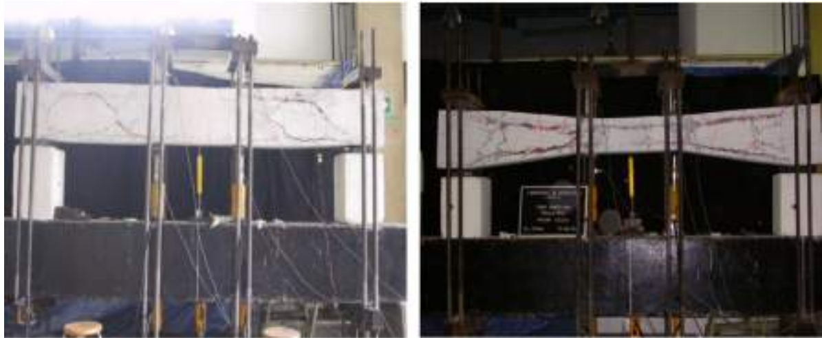
(a) Prismatic beam without stirrups.
