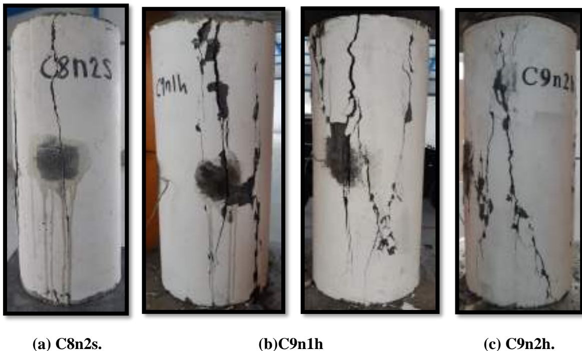
Figure (4-34): Crack pattern and failure mode of series D columns.
