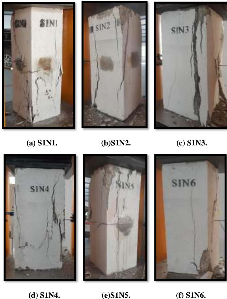
Figure (4-3): Crack pattern and failure mode of G1 specimens.
