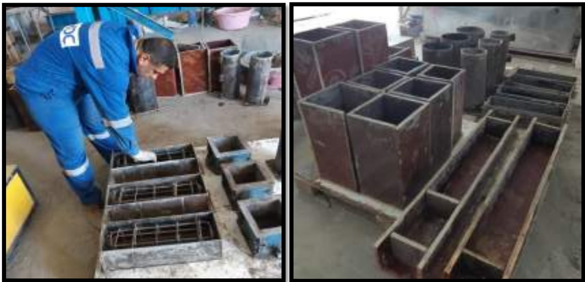
Figure (3-12): Moulds of the specimens.
