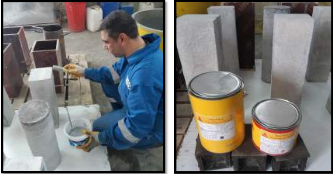
Figure (3-8): Using Sikadur®-32 epoxy for the bond purpose between the concrete column and the strengthening.
