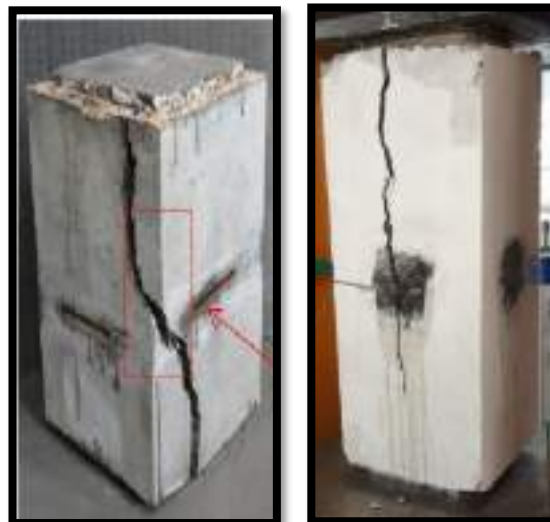
Figure (4-50): crack pattern and failure mode of typical confined column.
