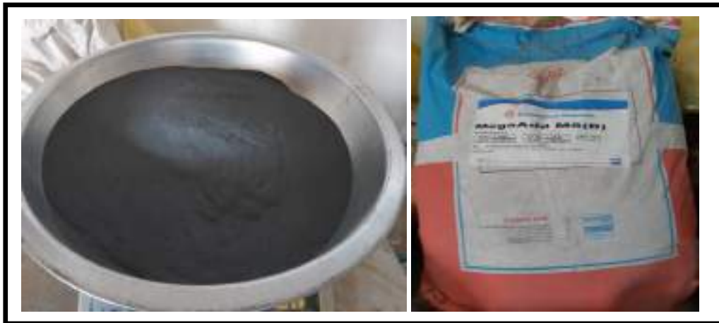
Figure (3-2): Silica fume material.
