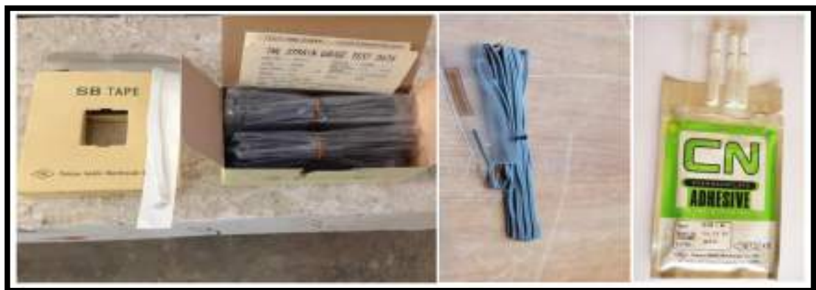
Figure (3-20): Strain gauge of concrete.
