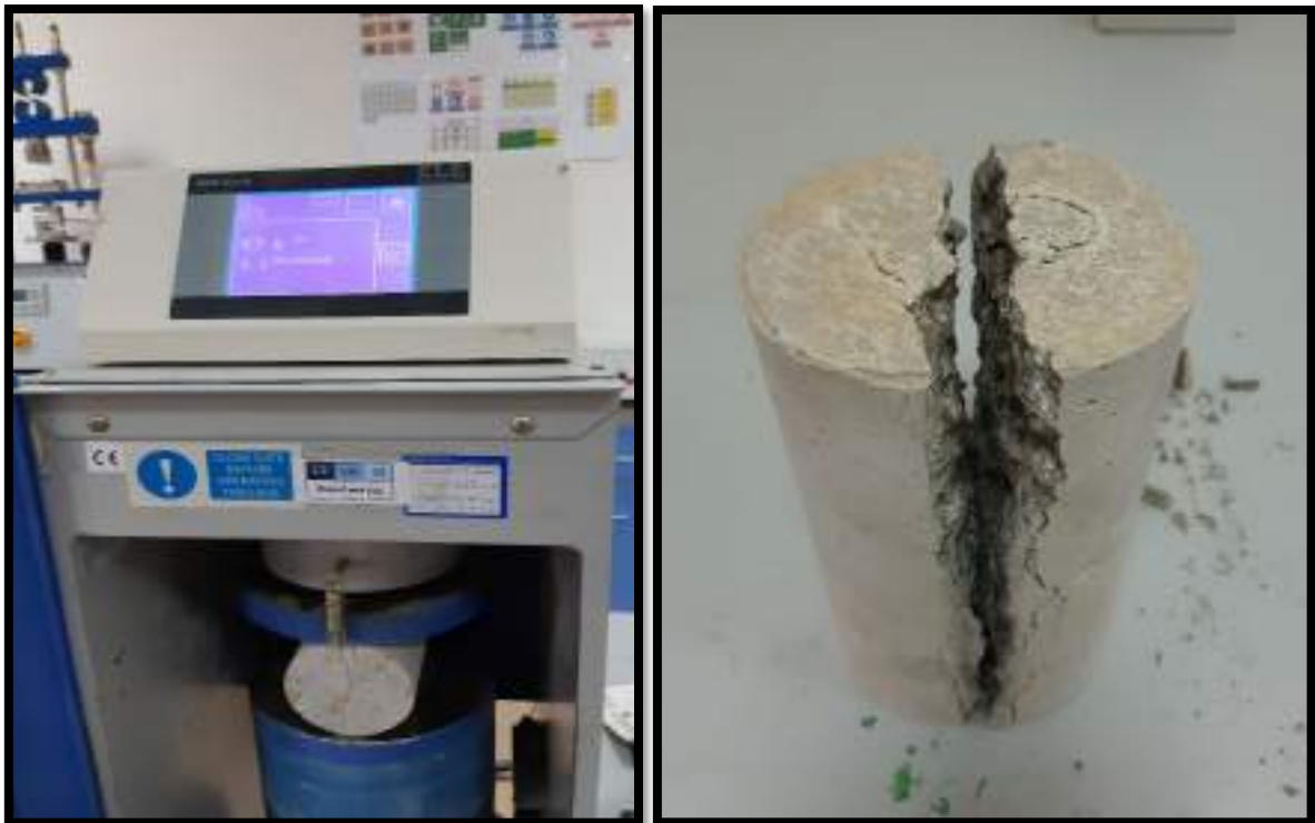
Figure (3-10): Split cylinder test with Failure pattern of cylinder specimen subjected to splitting stresses.
