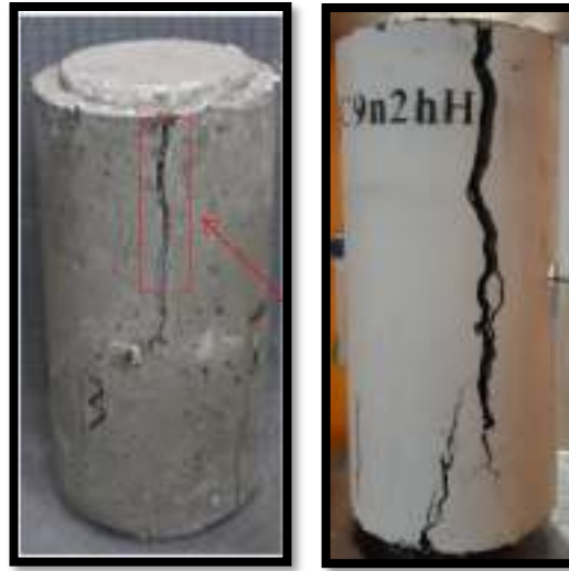
Figure (4-49): crack pattern and failure mode of typical confined column.
