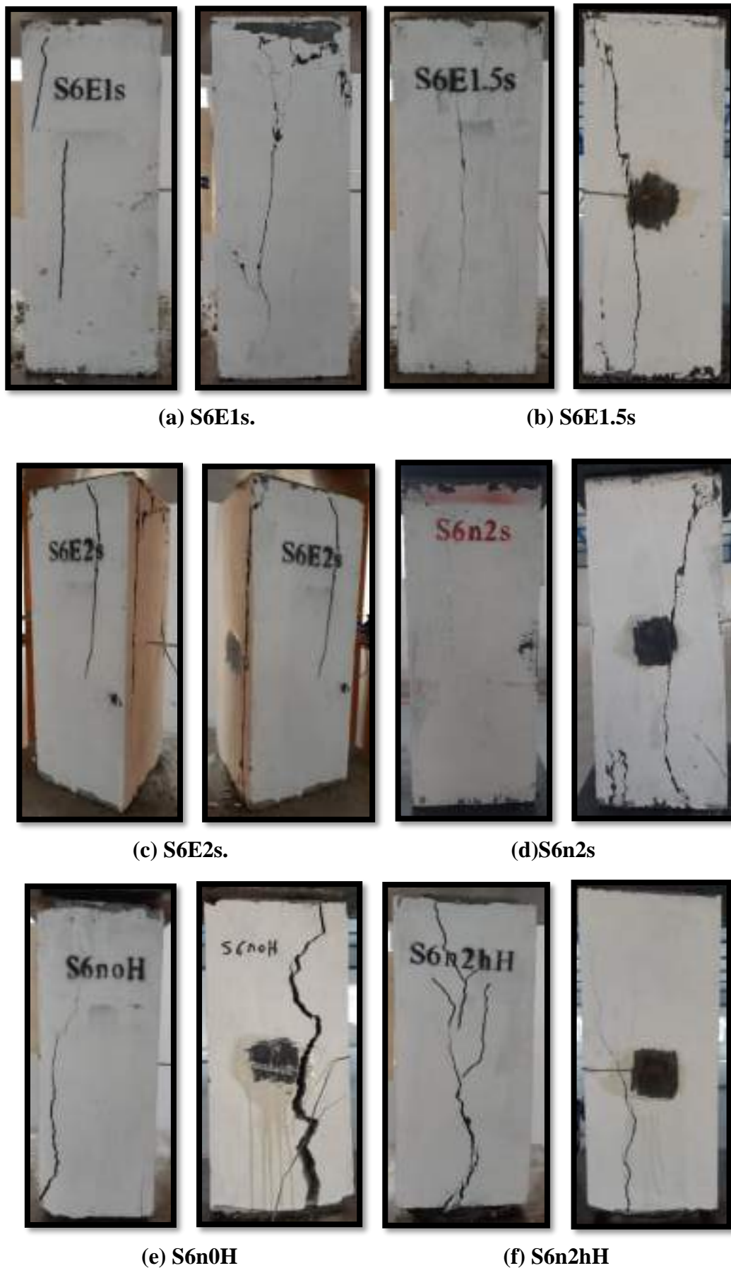
Figure (4-25): Crack pattern and failure mode of series C columns.
