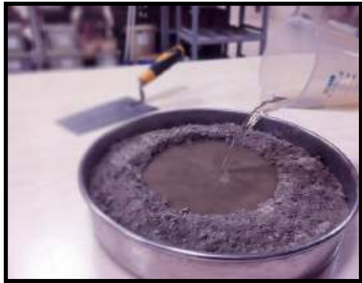
Figure (3-4): Adding potable water to the concrete mixture.
