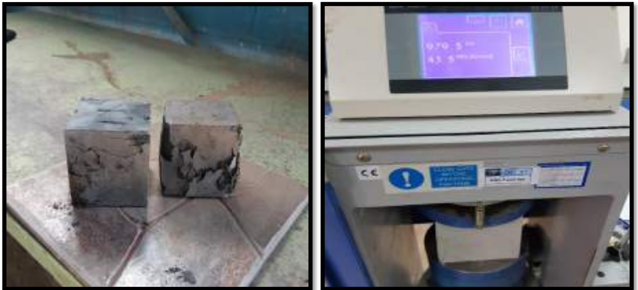
Figure (3-9): Compressive strength test with failure pattern of the specimen subjected to axial compressive stresses.
