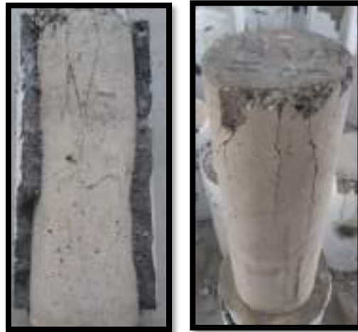
Figure (4-47): crack pattern and failure mode of typical confined column.
