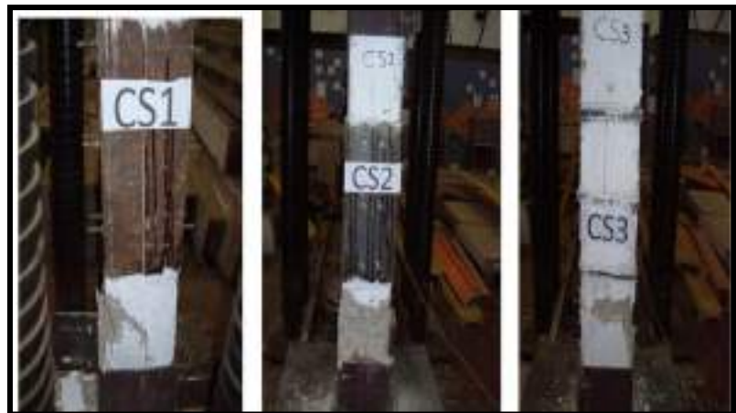
Figure (2-8). Failure modes of confined and unconfined concrete specimens.
