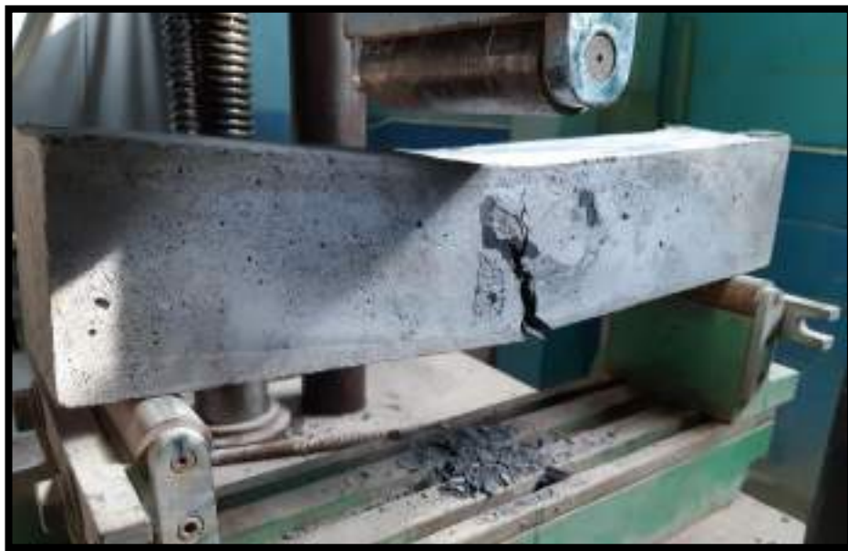
Figure (3-11): Flexural prism test for SFRC.
