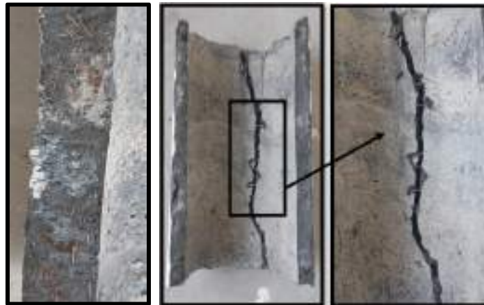
Figure (4-48): crack pattern and failure mode of typical confined column.
