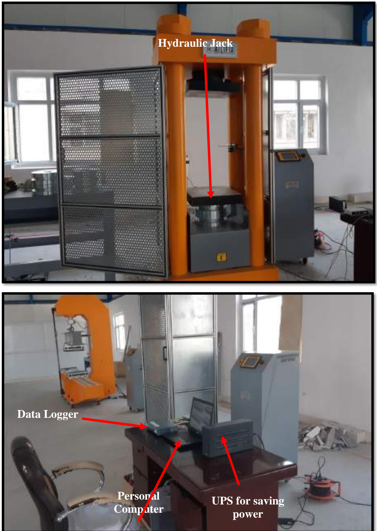
Figure (3-24): Setup of typical tested column.
