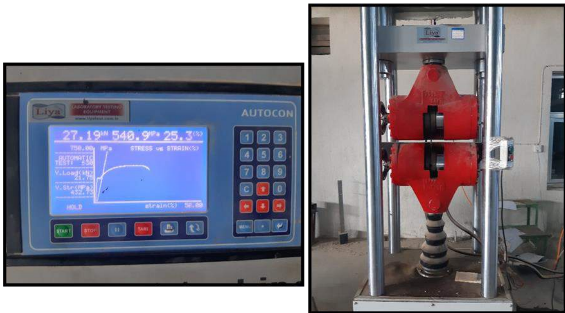
Figure (3-7): Steel reinforcement test.
