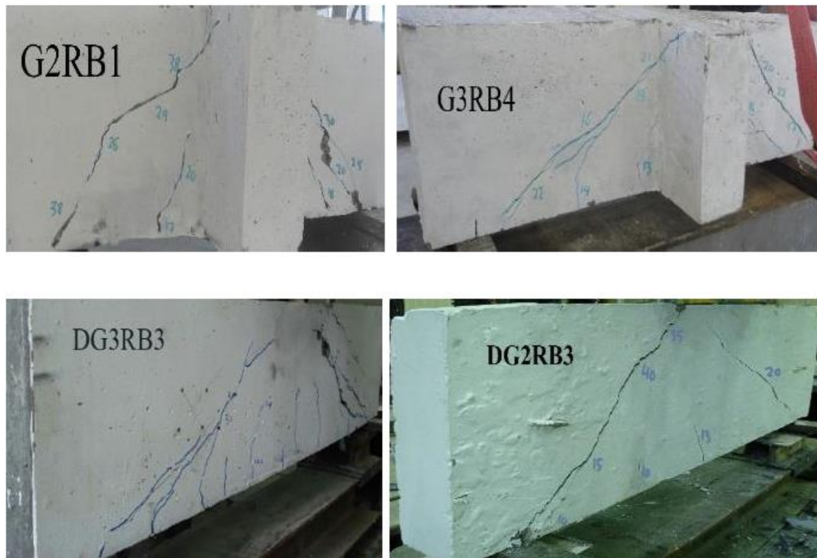
Figure 2- 9 Specimens tested by Alhussein and Khudhair
