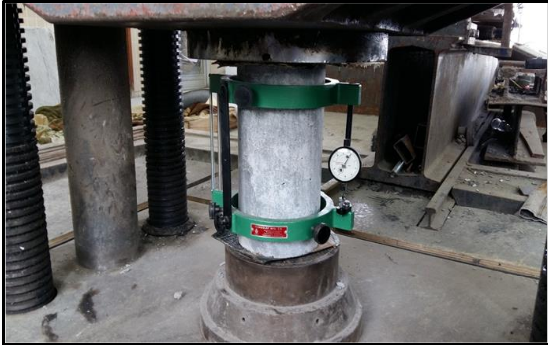
Figure 3- 7 Modulus of Elasticity Test.
