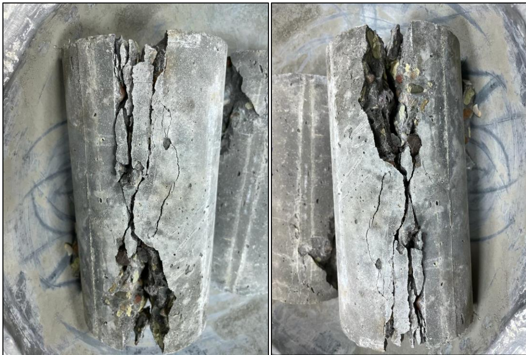
Figure 3- 5 splitting tensile test.
