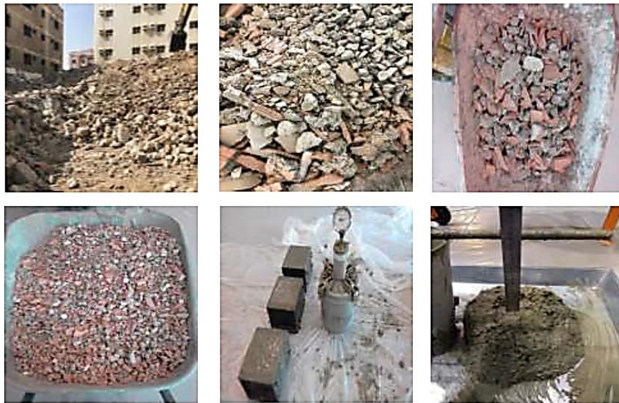
Figure 2- 4 Concrete mix with recycled construction demolition waste
