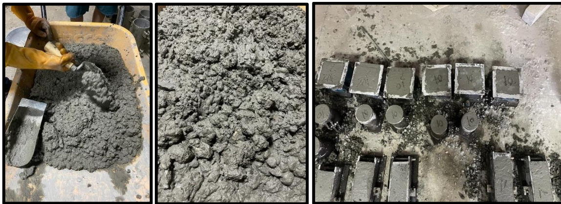
Figure 3- 4 Concrete specimens' fabrication.
