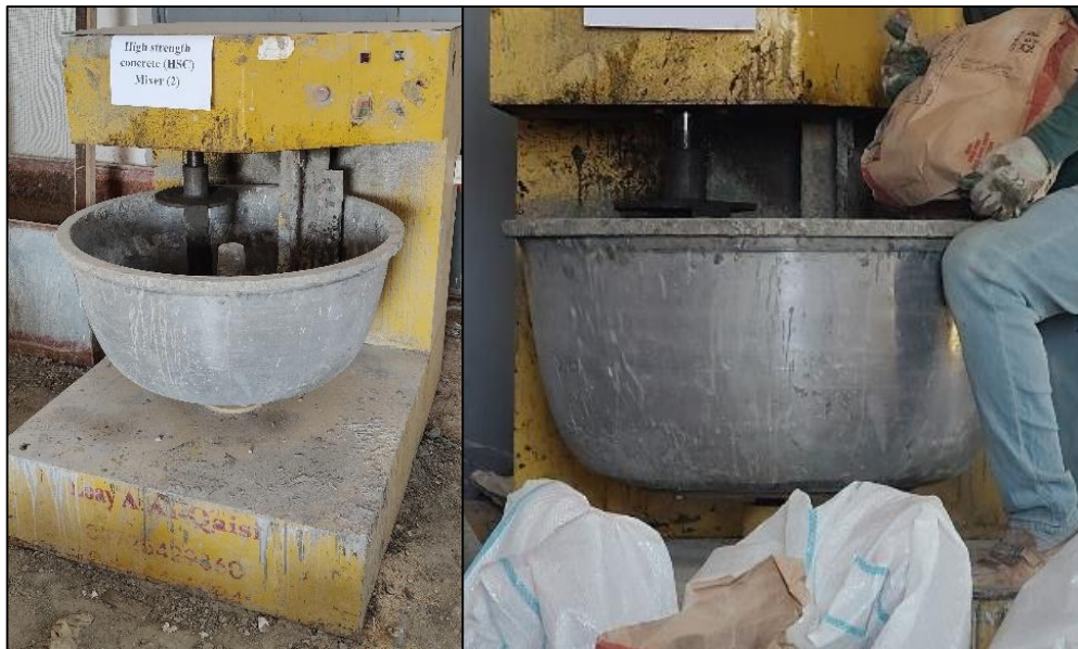
Figure 3.12 Mixer (2) for high strength concrete.
