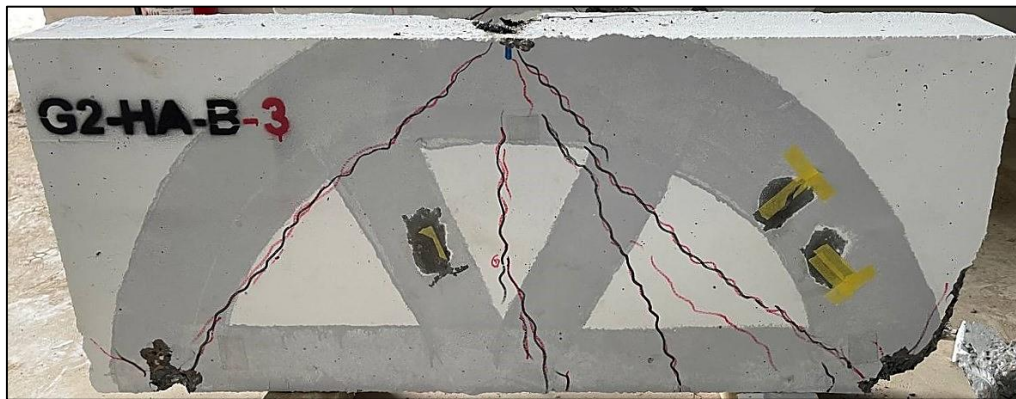
Figure 4.15 Cracks propagation for specimen G2-HA-B-3.
