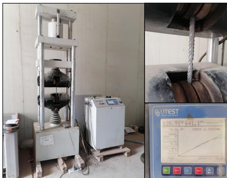
Figure 3.8 Reinforcement bar testing machine.
