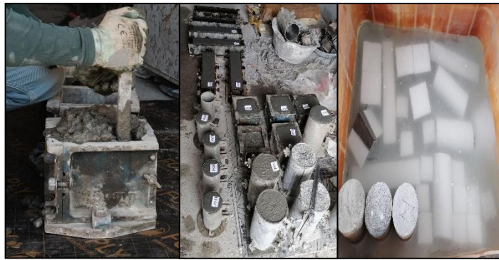
Figure 3.14 Sampling and curing of concrete specimens.
