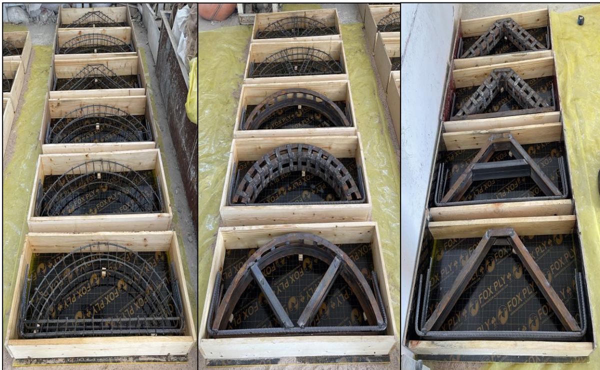
Figure 3.22 Preparing specimens for casting process.
