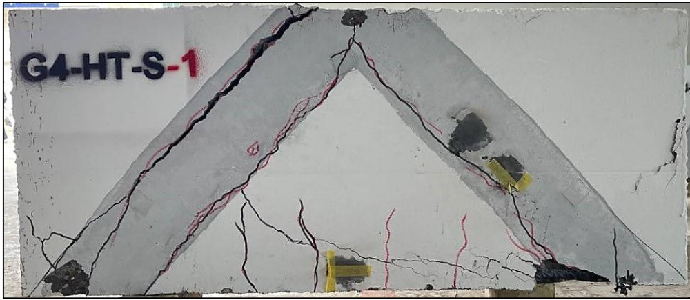
Figure 4.20 Cracks propagation for specimen G4-HT-S-1.
