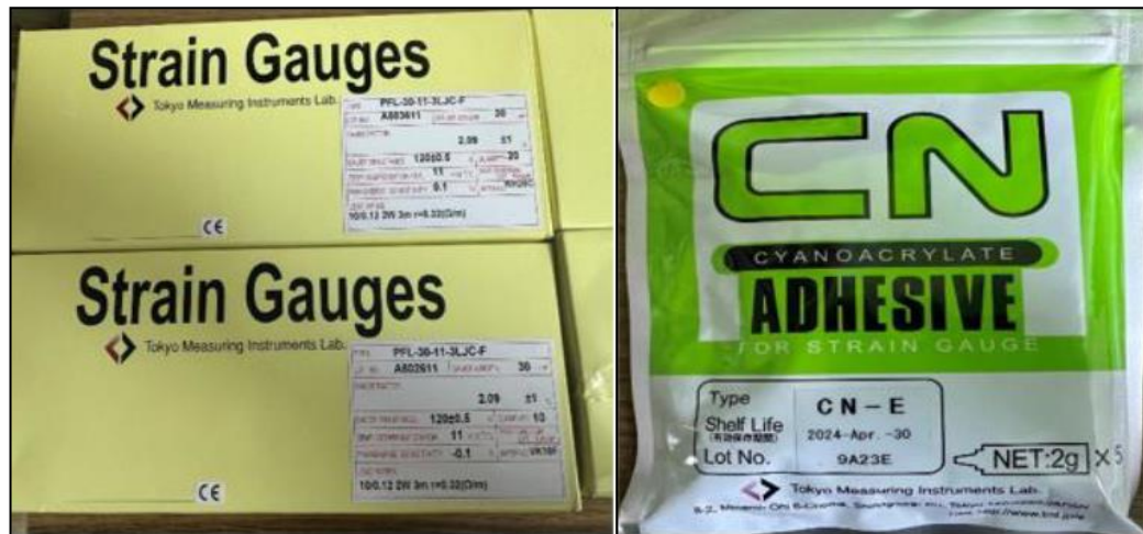
Figure 3.29 Concrete strain gauges and their glue.
