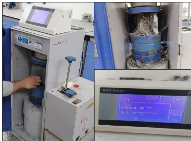
Figure 3.15 Compressive strength test.
