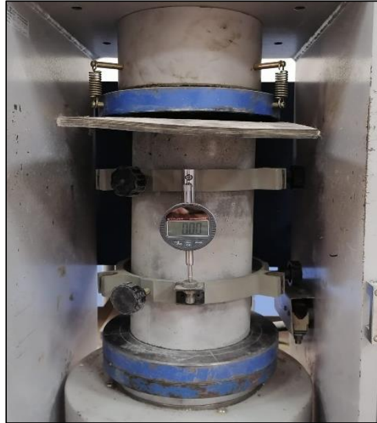
Figure 3.18 Modulus of Elasticity test.
