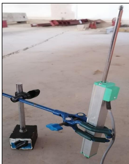
Figure 3.30 Linear variable differential transformers (LVDT).
