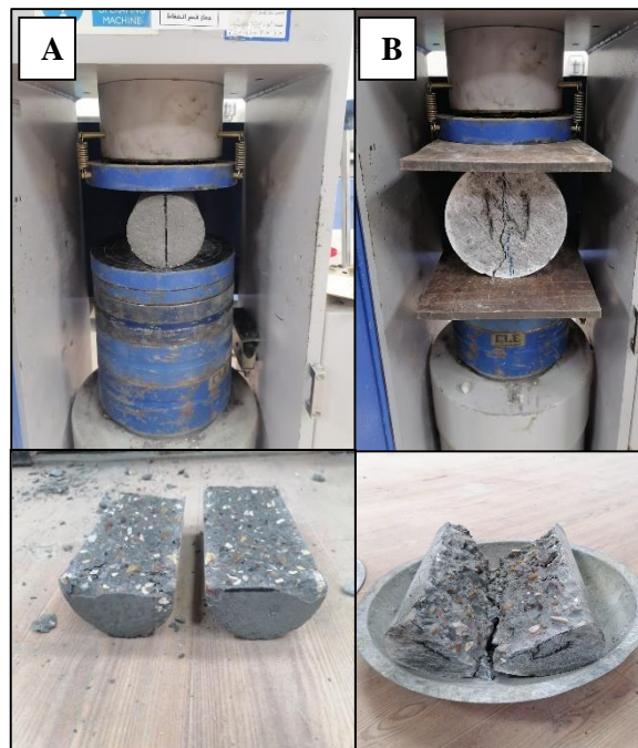
Figure 3.16 Splitting tensile strength test for (A)HSC, (B)NSC.
