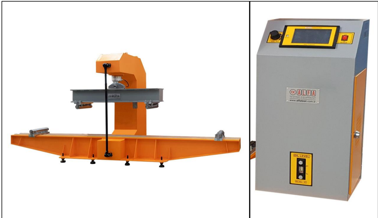
Figure 3.27 Flexural Test Machine.
