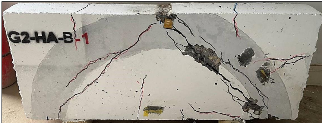
Figure 4.13 Cracks propagation for specimen G2-HA-B-1.
