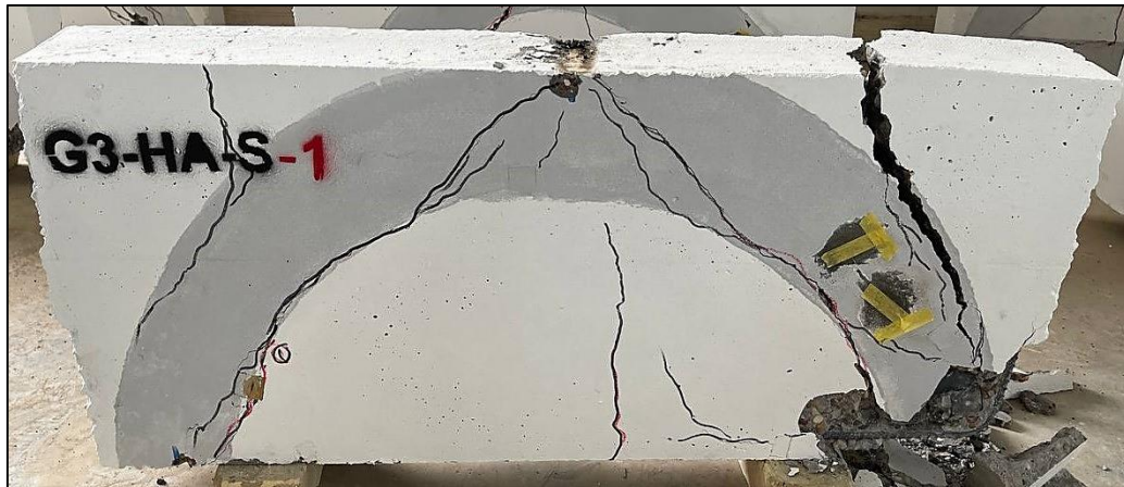
figure 4.17 cracks propagation for specimen G3-HA-S-1.
