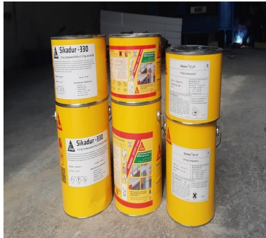
Figure 3.7 Types of adhesive material (epoxy)
