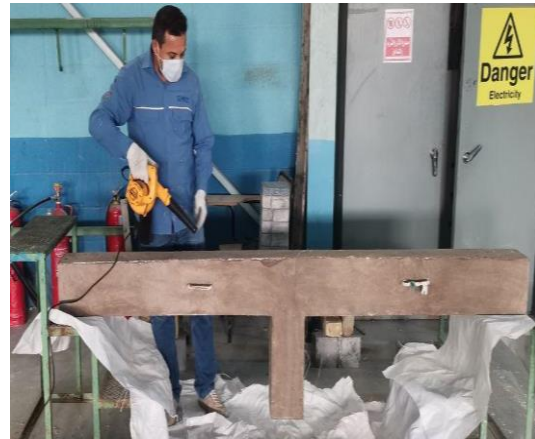
(b) Cleaning the surface
