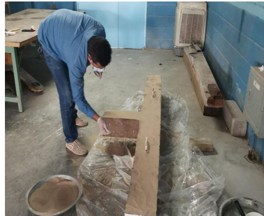
(d) Sprayed fine sand as anti-slip
