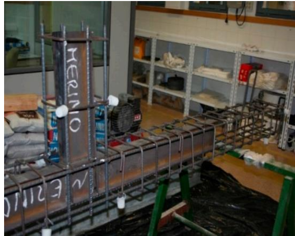
Figure 2.19 Strengthening scheme of the specimens (Montava et al., 2019)
