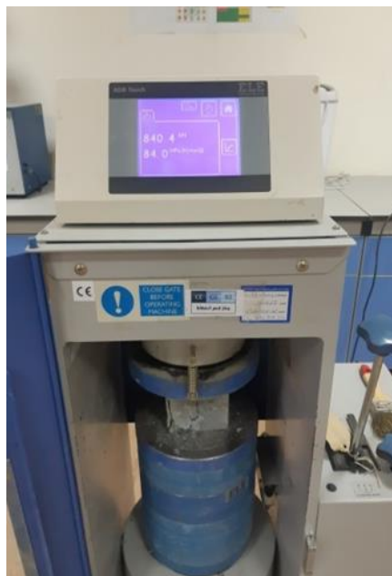
Figure 3.16 Compressive strength test
