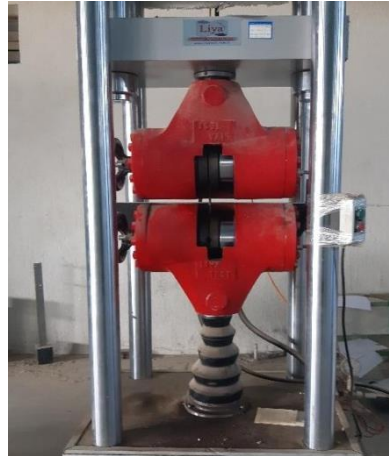
Figure 3.4 Testing machine of steel bars
