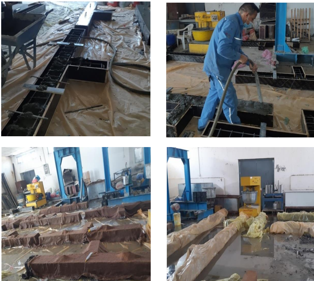
Figure 3.11 Casting and curing the specimens
