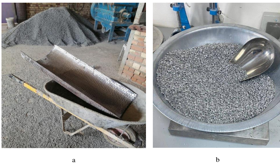
Figure 3.4 a-Filter With 6 mm Openings b- Graded PVC Particles.
