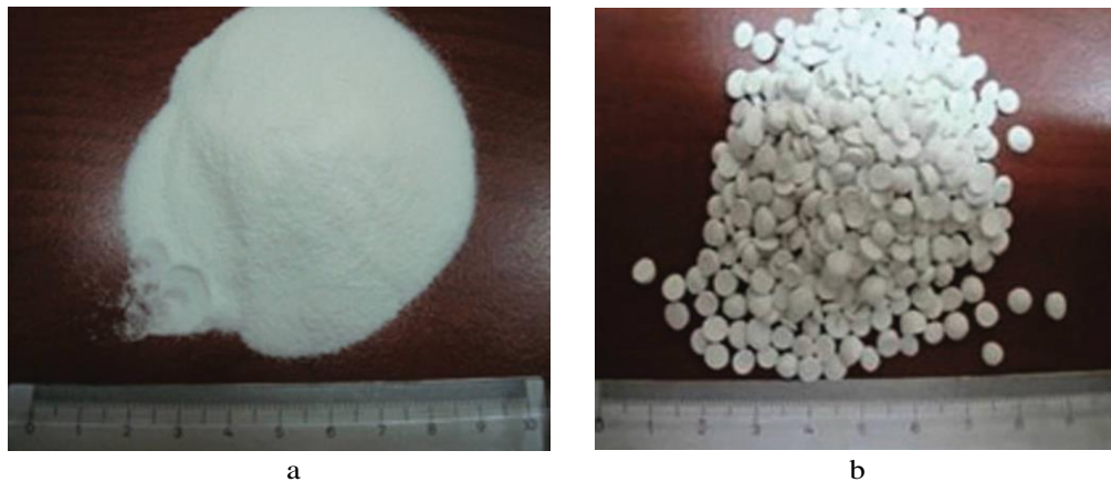
Figure 2.18 PVC Particles a-Powder, b-Granules [39].
