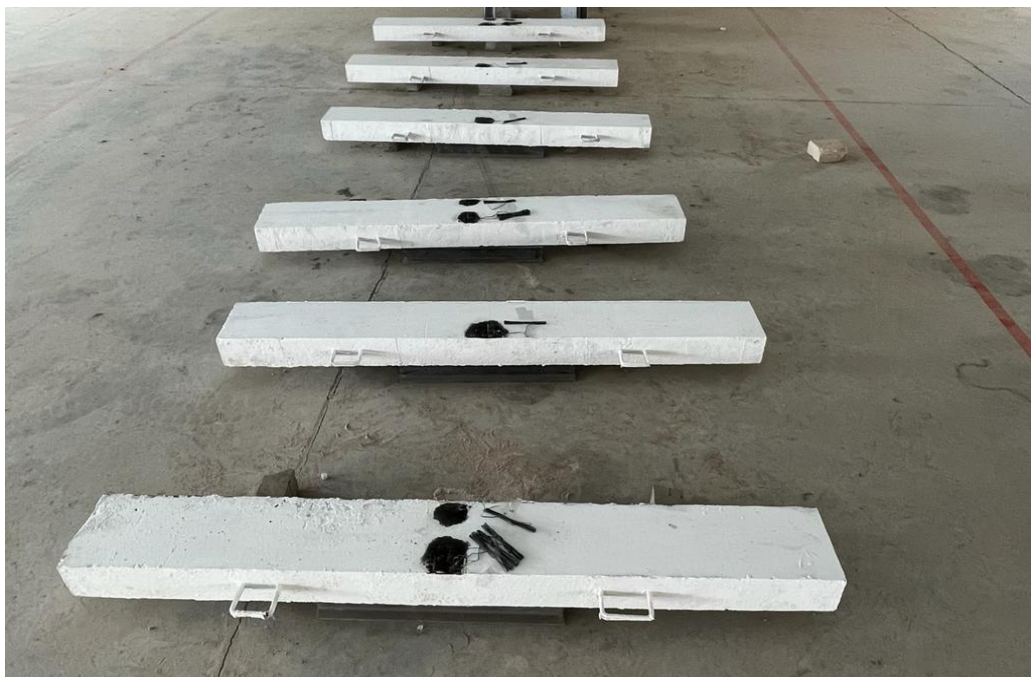
Figure 4.16 Reinforced Concrete Beams Used for All PVC/SAND Percentages.
