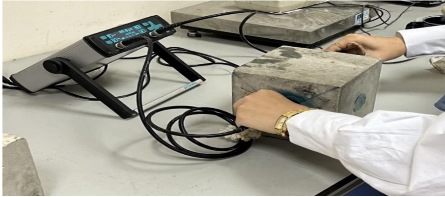
Figure 3.15 The Ultrasonic Pulse Velocity Test.
