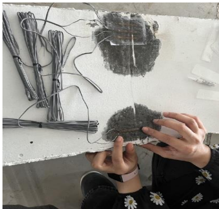
b. strain gages attaching for 0%, 10% and 30% ratios
