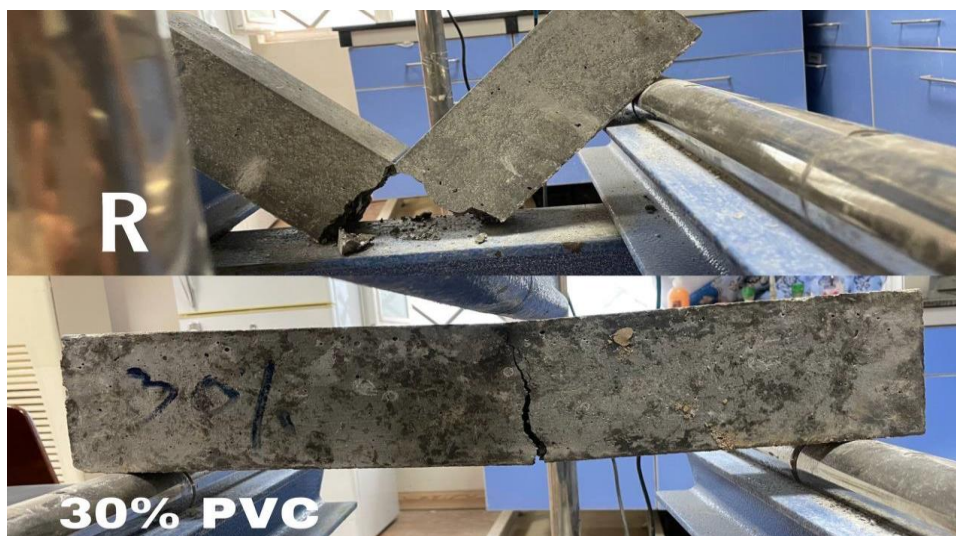
Figure 4.8 The Failure Mode of Concrete Prisms for Reference(R) And 30% PVC/Sand Percentages.
