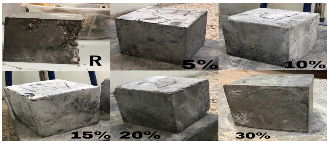
Figure 4.4 The Failure Mode of Concrete Cubes for Reference and All PVC/SAND Percentages.
