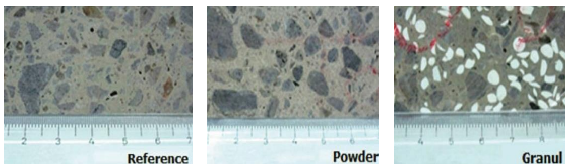
Figure 2.19 The Cross Section of Concrete with PVC Waste [39].
