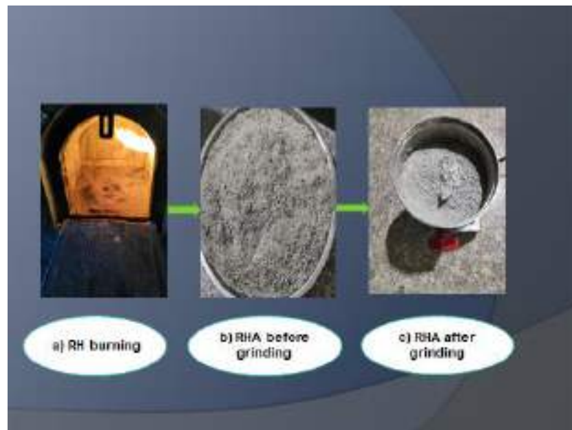
Fig. (3-11): Rice husk ash produced.
