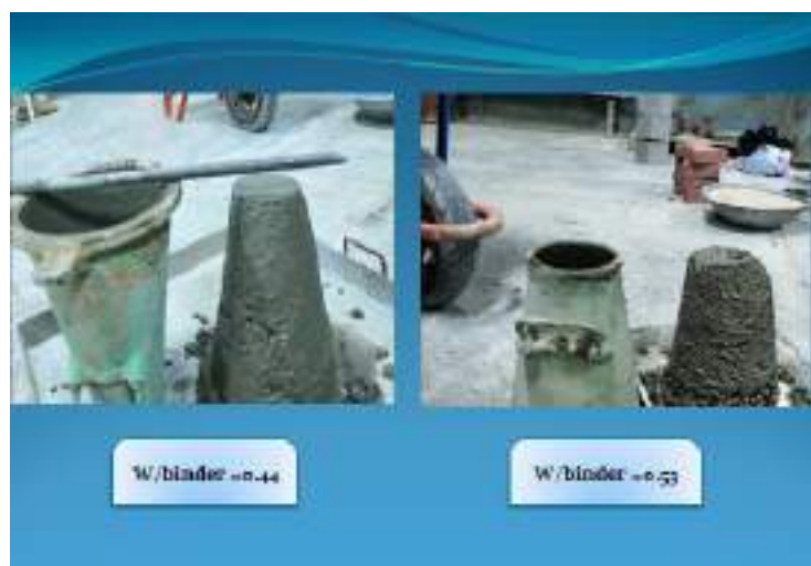
Fig. (3-13): The slump cone test.
