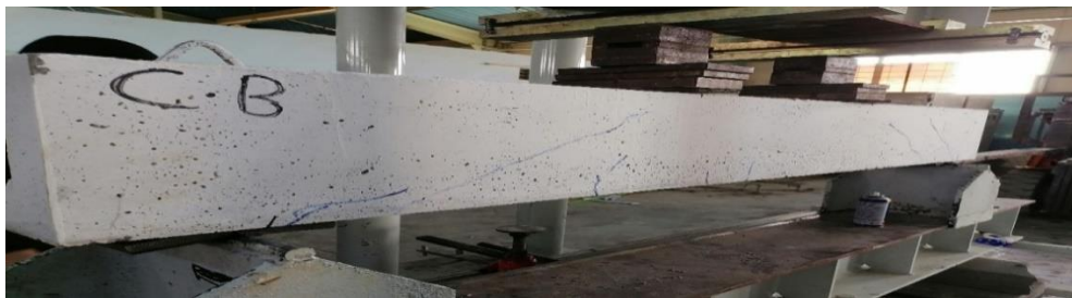
Figure 4.1 Load-deflection behavior and crack patterns for CB.
