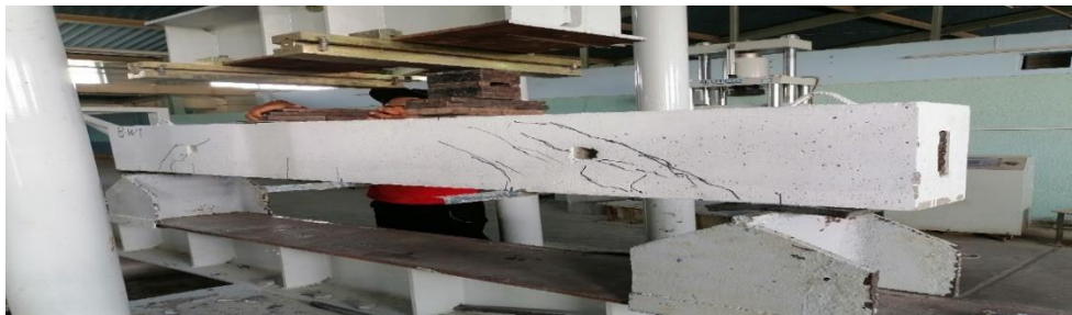
Figure 4.2 Load-deflection behavior and crack patterns for BW1.
