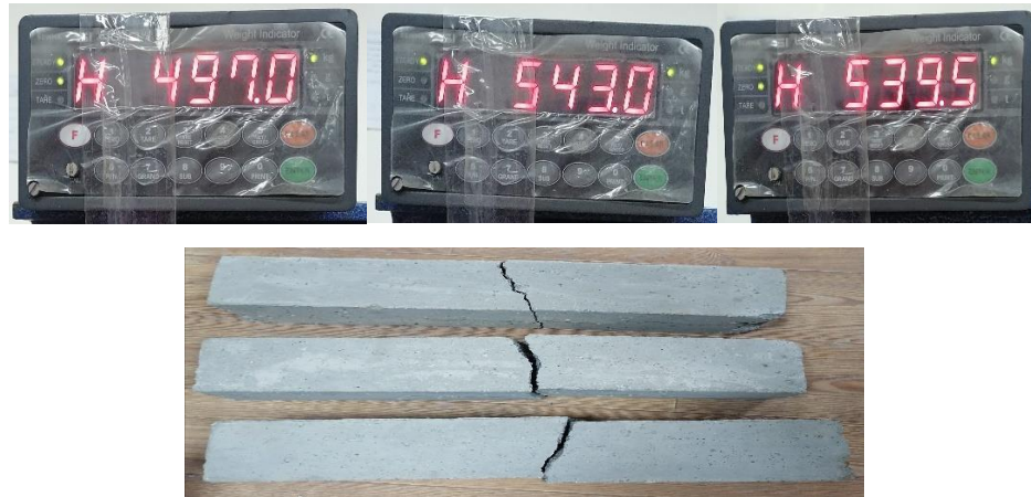
Figure 3.25 Test results and failure modes of modulus of rupture for prisms.
