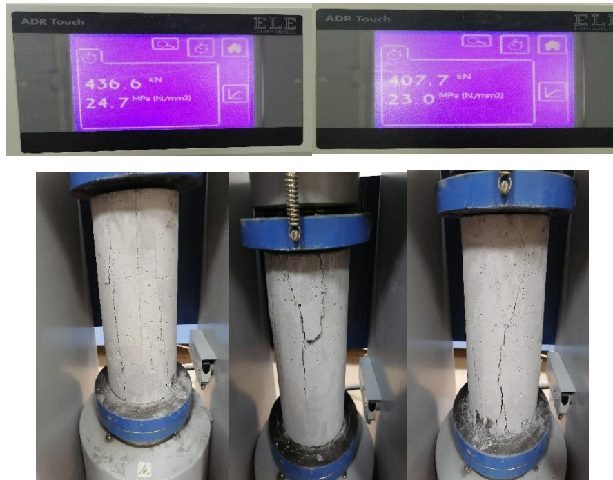
Figure 3.23 Compressive Strength Results and failure modes.
