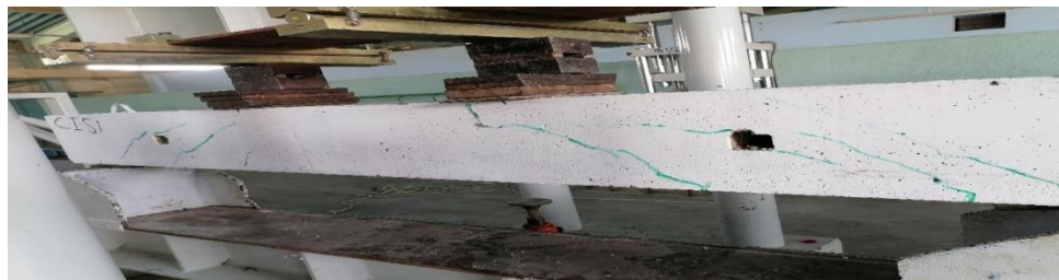
Figure 4.4 Load-deflection behavior and crack patterns for CIS1.
