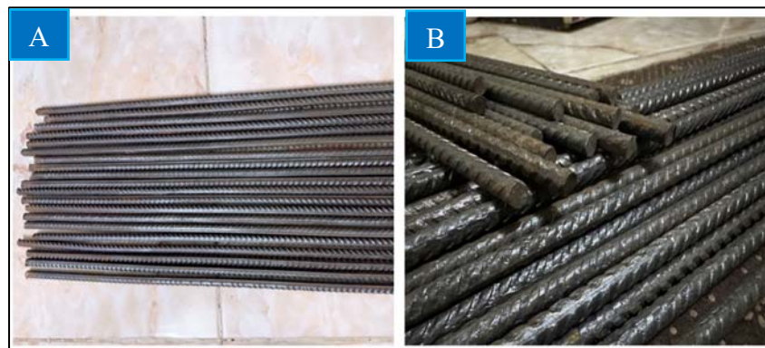
Figure 3.2 Steel bars used in the models (A) Ø 8mm, (B) Ø 6mm.
