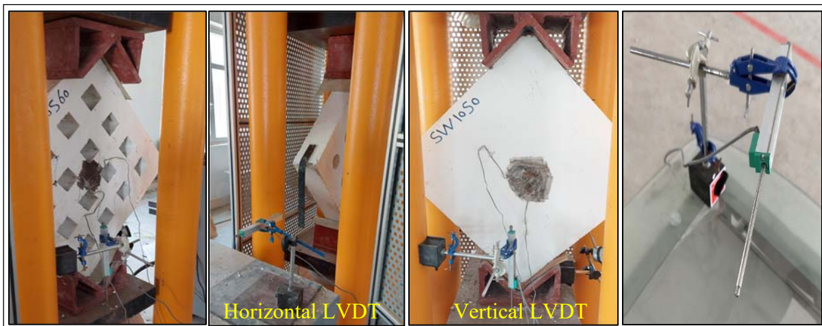
Figure 3.17 Setup of LVDT.
