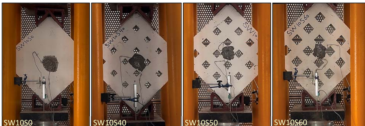
Figure 3.20 Testing setup for the tested shear wall specimens.
