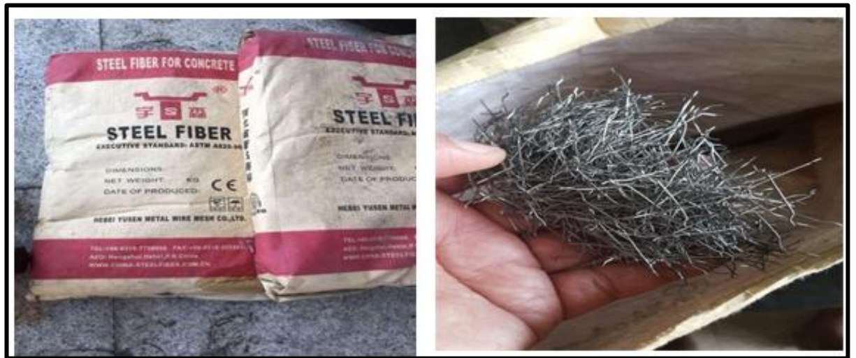
Figure 3.6 Shape of hooked steel fiber.
