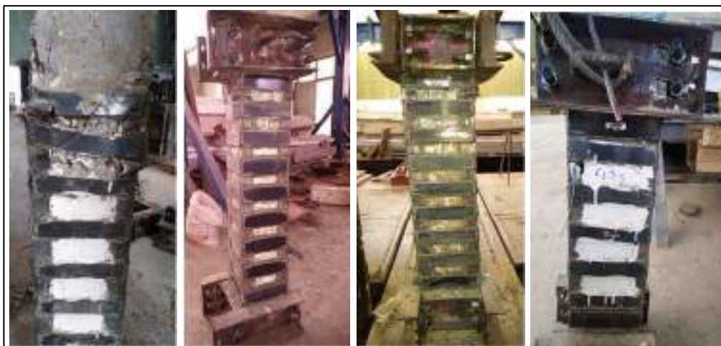
Figure 1.2 Details of Steel Jacketing Technique.[8]
