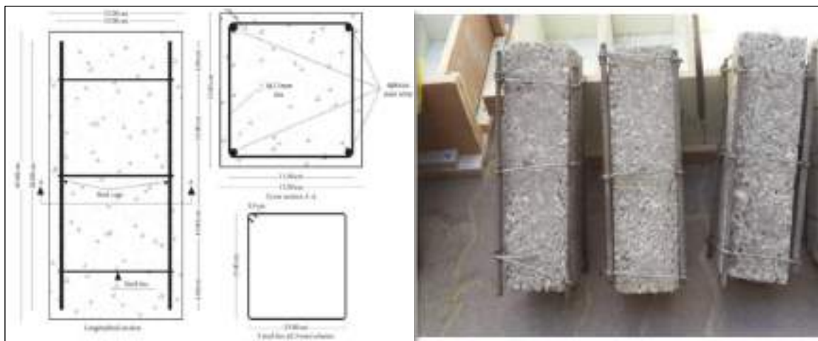
Figure 2.5 Geometry and Reinforcement Details of Columns.[38]
