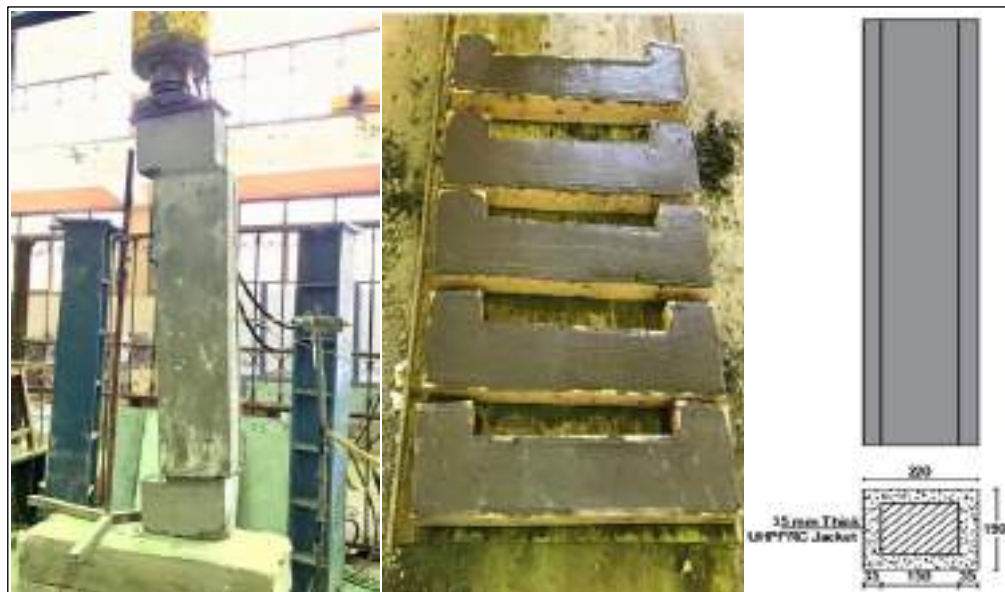
Figure 1.6 Details of HPFRC Jacketing technique.[13]
