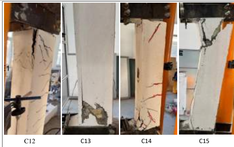
Figure 4.5 Mode Failure and Cracks Pattern for Group c 35% Defect Ratio Foam.
