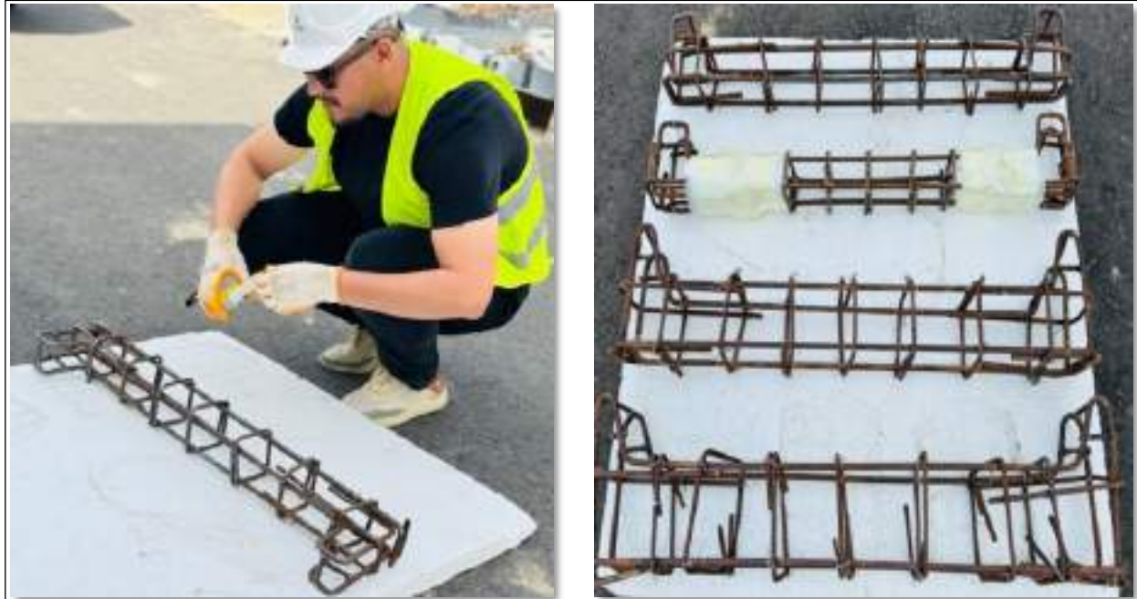
Figure 3.14 The Reinforcement Details of Specimens.
