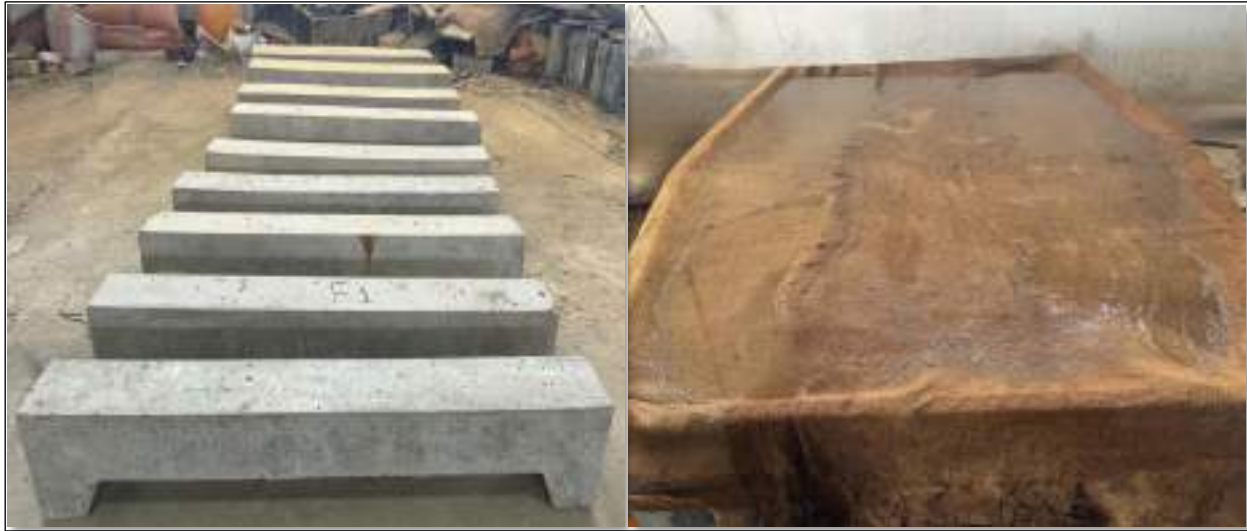
Figure 3.22 Demolding and Curing Process of Specimens and Samples in Water Tank.
