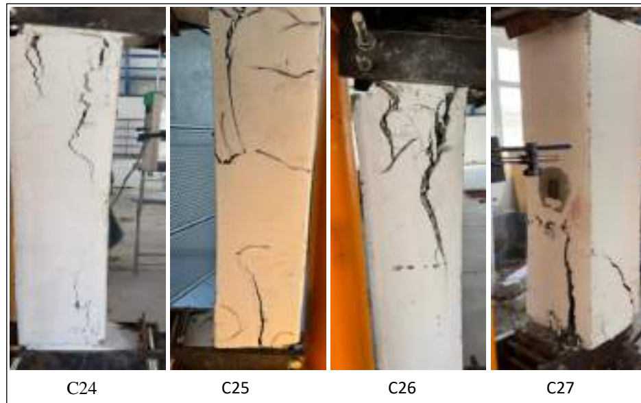
Figure 4.12 Mode Failure and Cracks Pattern for Group f 70% Defect Ratio WSC.
