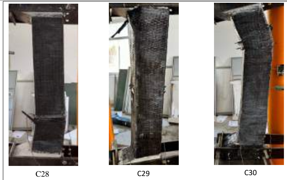
Figure 4.13 Mode Failure and Cracks Pattern for Group g 70% Defect Ratio.
