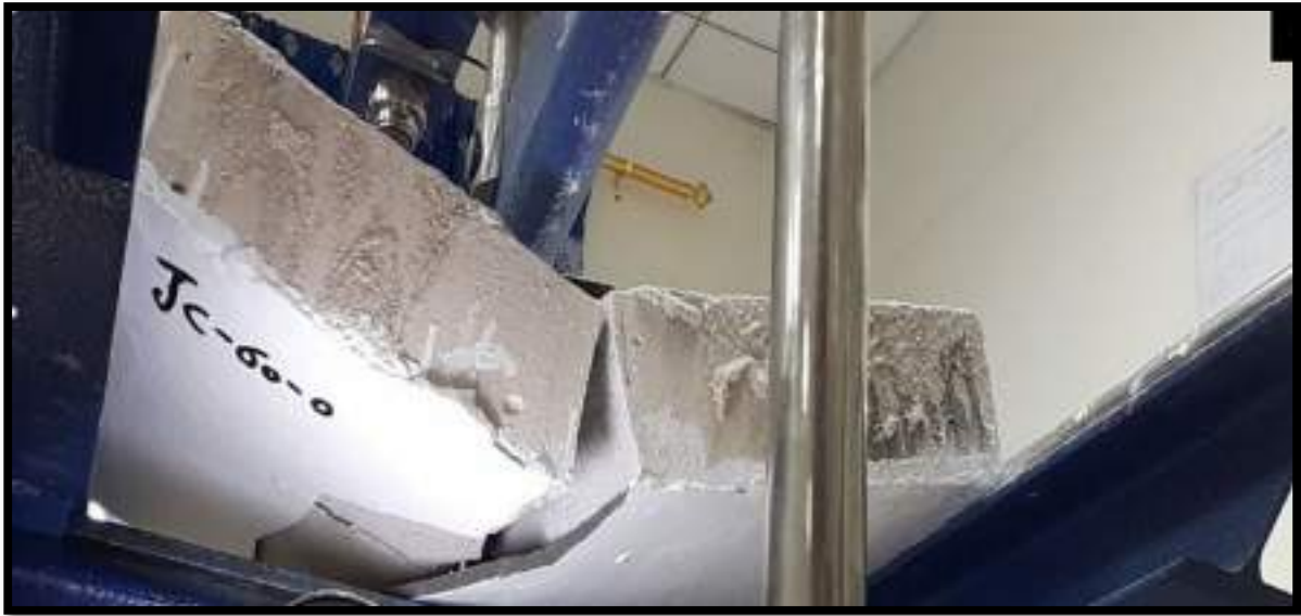
(e) Mode of failure for Jc-60-0 specimen.
