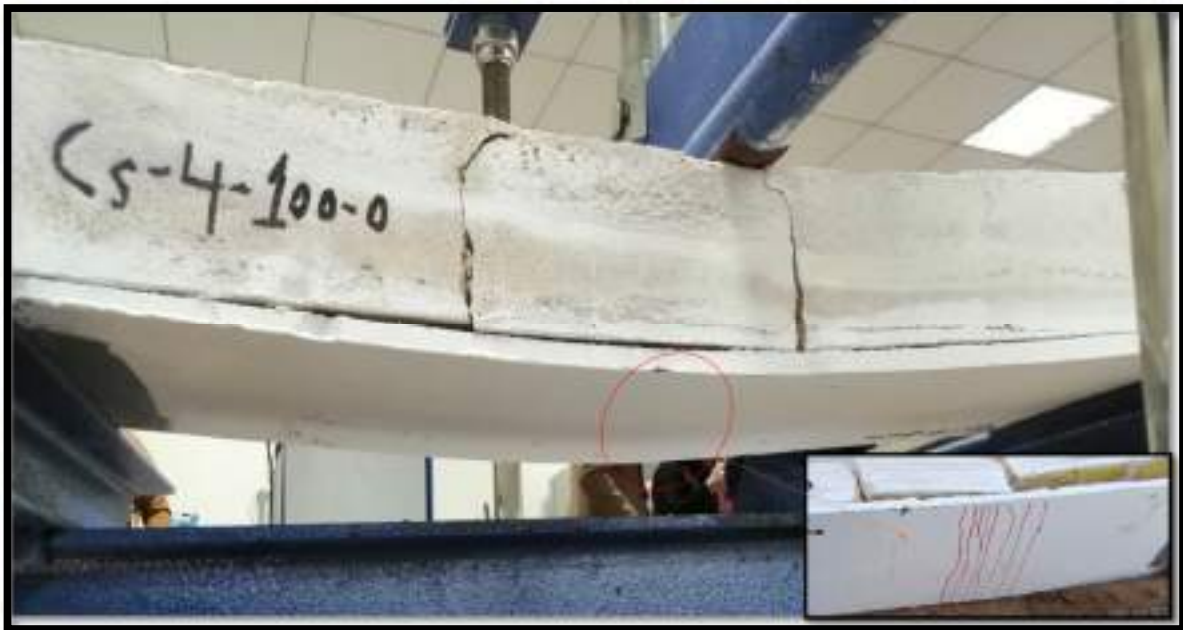
(e) Mode of failure for Cs-4-100-0 specimen.
