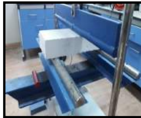
(e) Modulus of rupture test.
