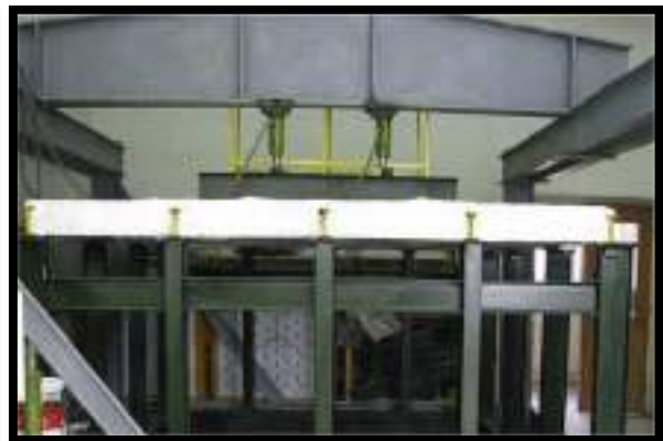
(d) test set-up for out-of-plane pushover loading of the slabs
