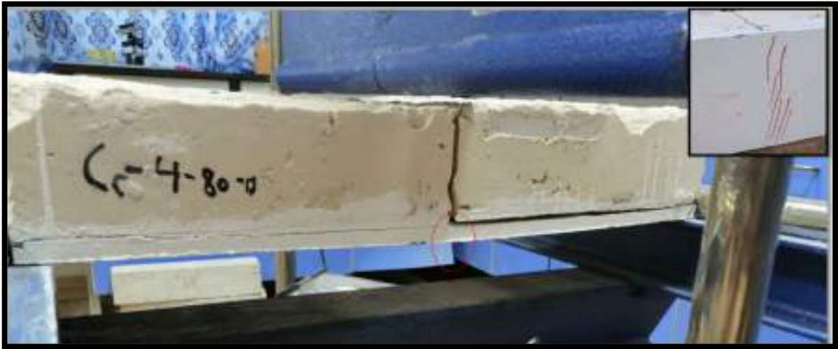
(k) Mode of failure for Cc-4-80-0 specimen.
