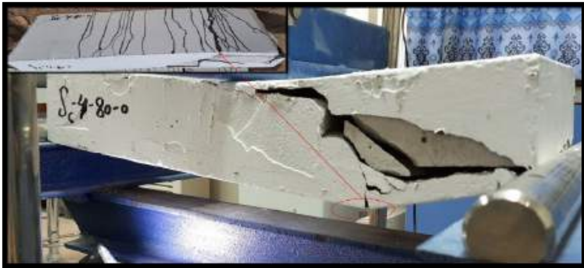
(a) Mode of failure for Sc-4-80-0 specimen.
