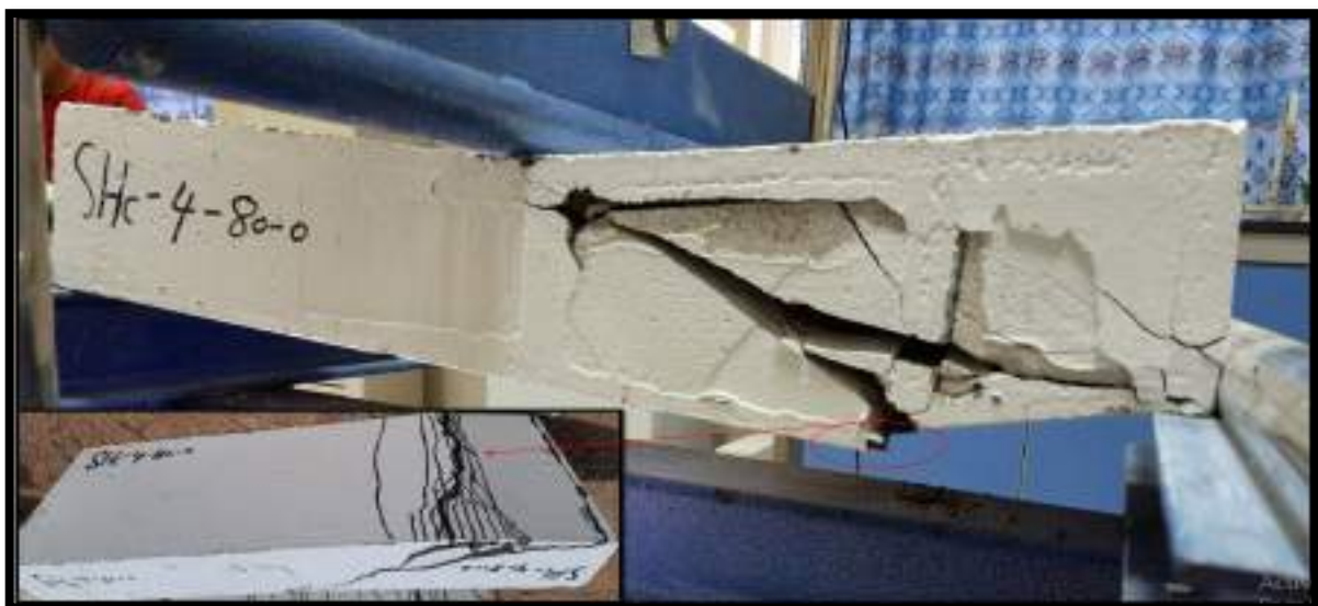
(b) Mode of failure for SHc-4-80-0 specimen.
