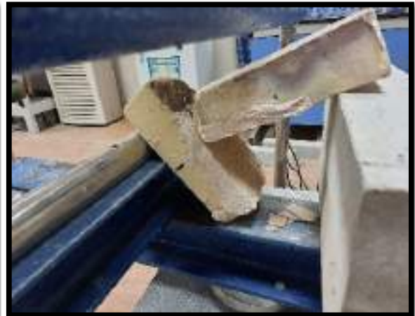
(b) Solid bricks after failure.
