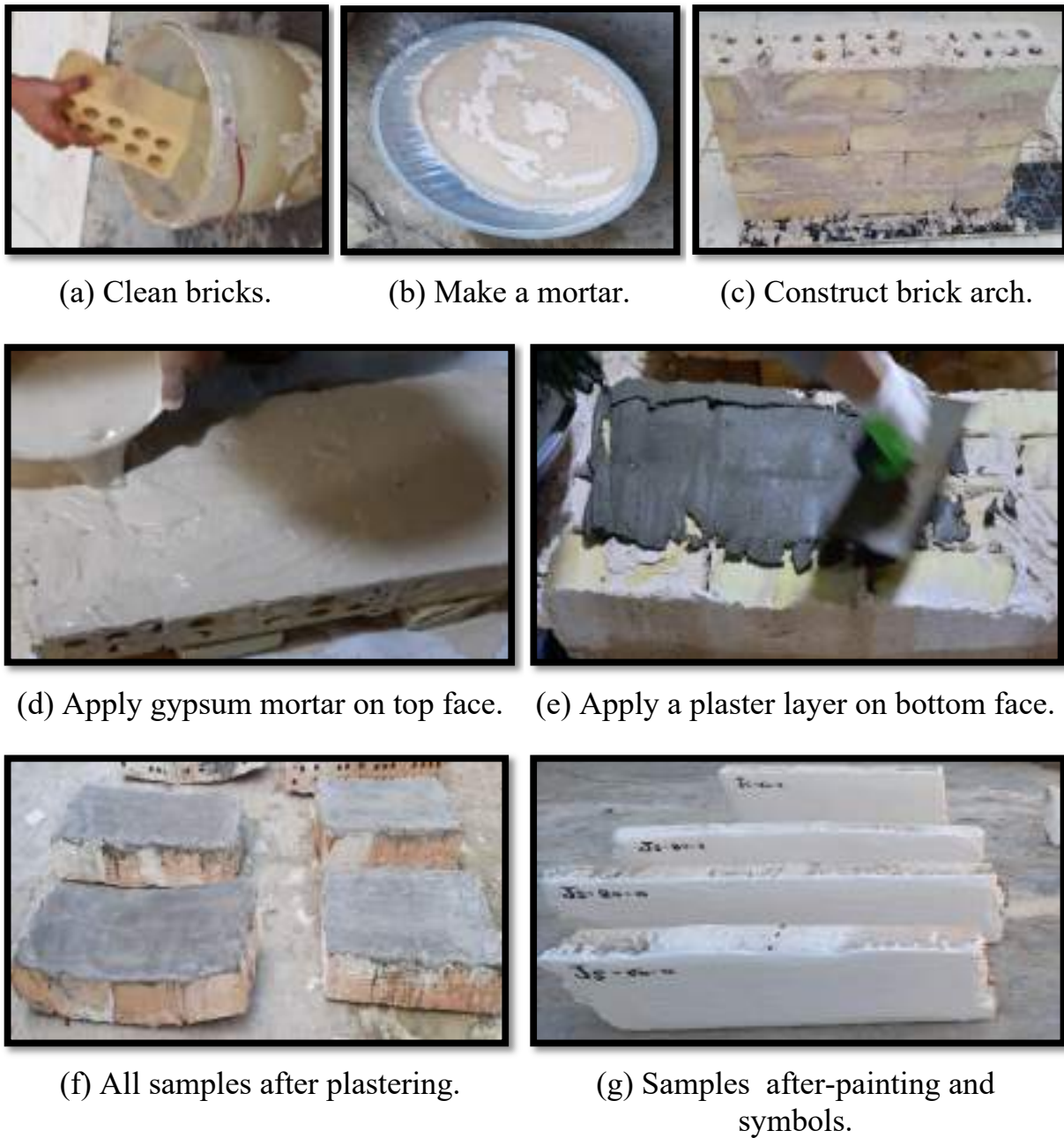
Figure. 3-12: Steps for preparing jack arch slab G_1 specimens.
