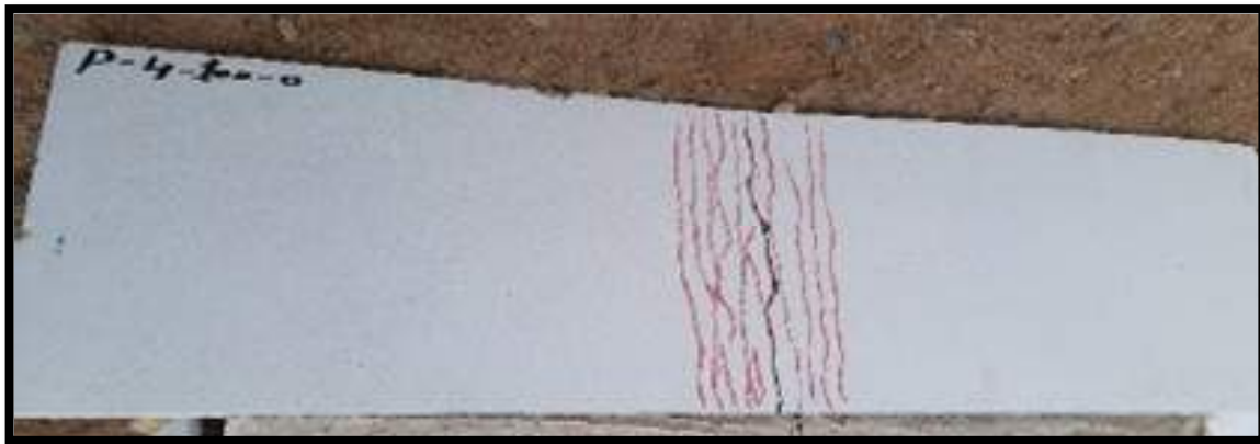
(e) Mode of failure for P-4-100-0 specimen.
