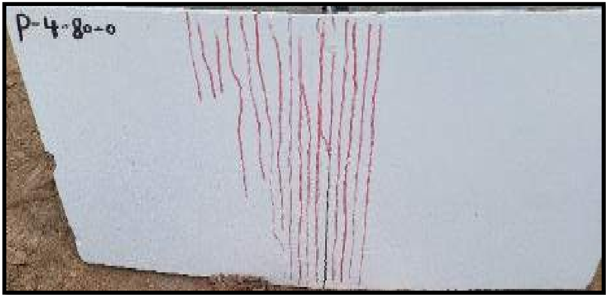
(c) Mode of failure for P-4-80-0 specimen.
