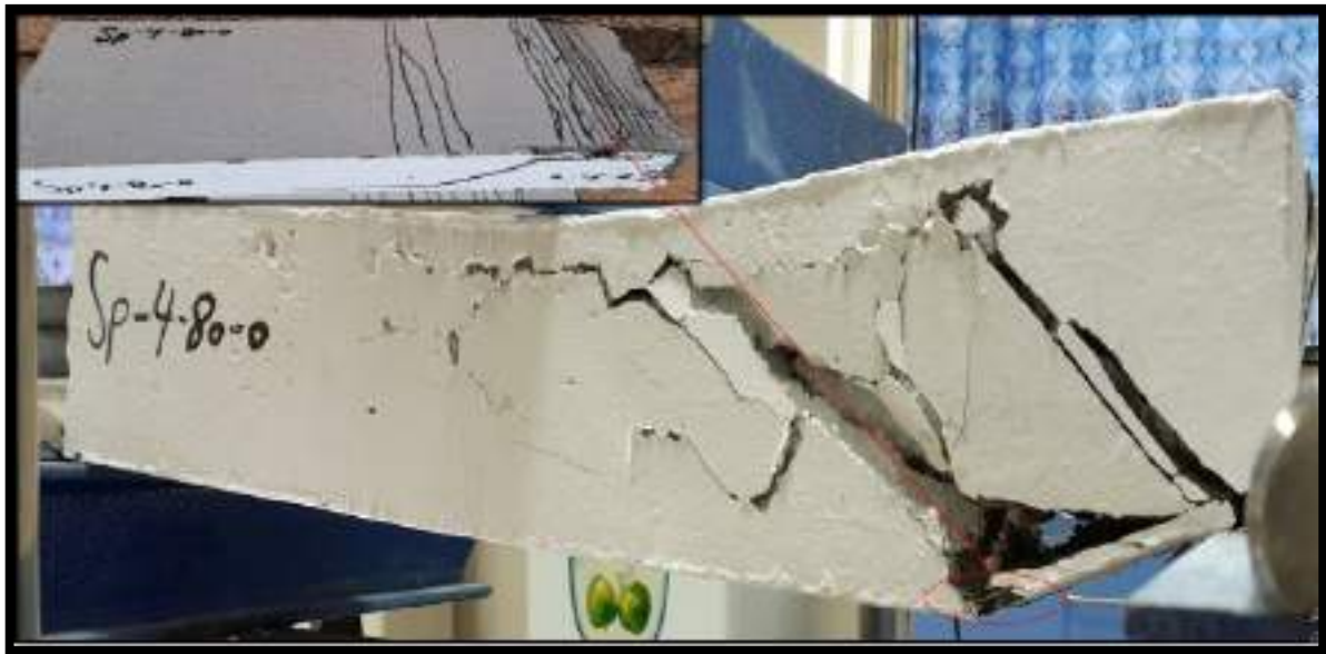
(c) Mode of failure for Sp-4-80-0 specimen.
