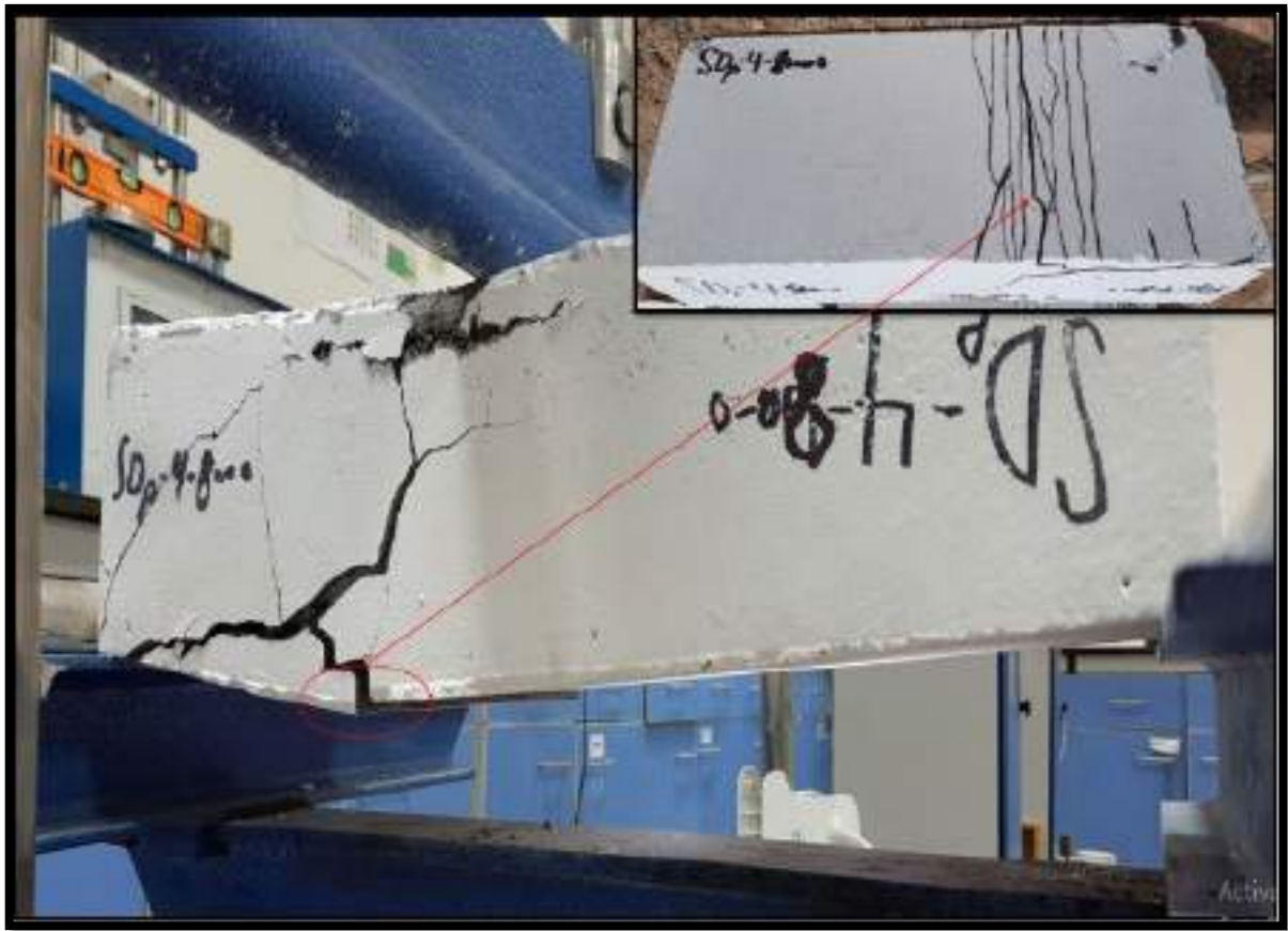
(g) Mode of failure for SDp-4-80-0 specimen.
