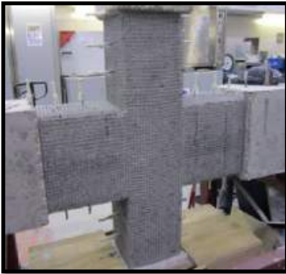
(a) Interior beam–column joints rehabilitated by ferrocement jackets [12].
