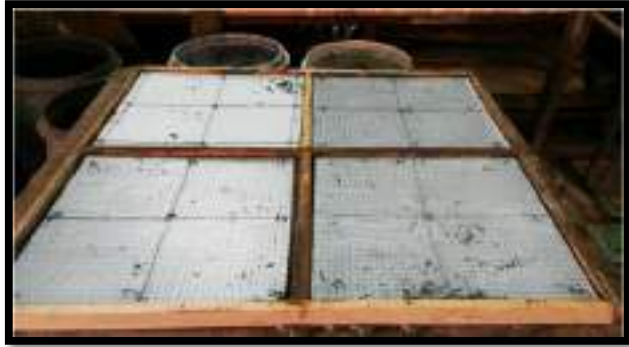
(b) fixing the reinforcement with core material.
