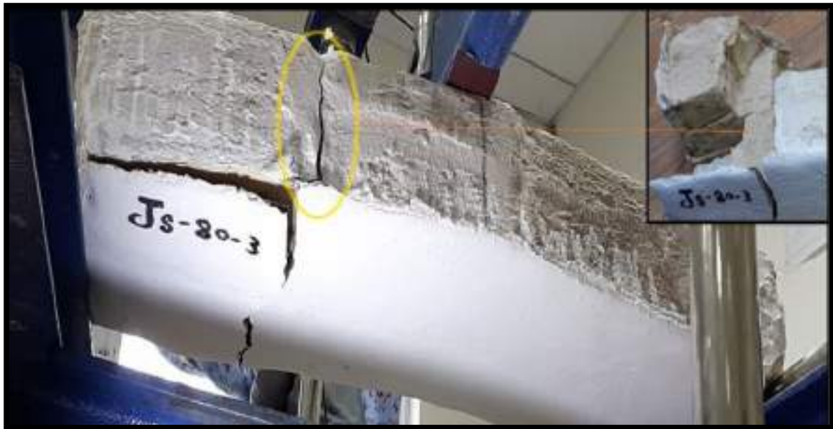
(c) Mode of failure for Js-80-3 specimen.
