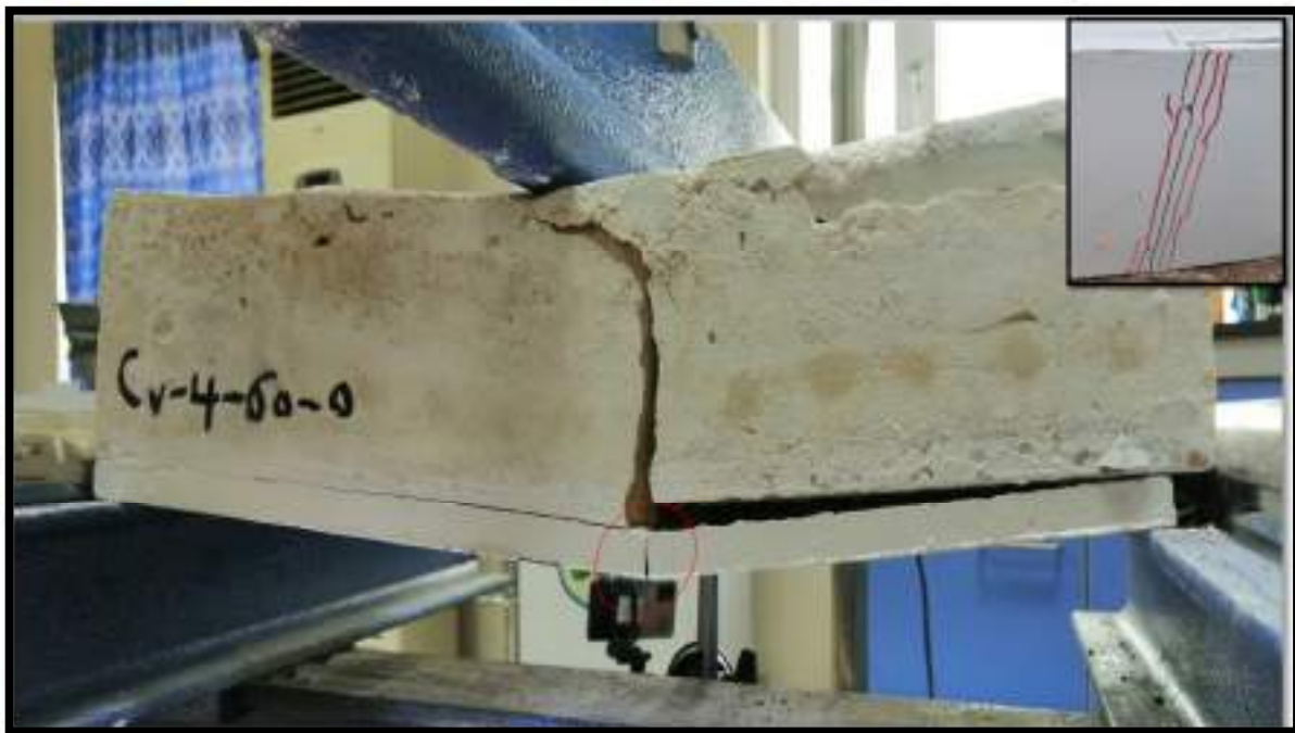
(h) Mode of failure for Cv-4-60-0 specimen.
