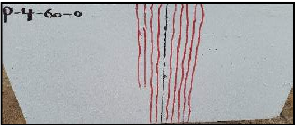
(b) Mode of failure for P-4-60-0 specimen.
