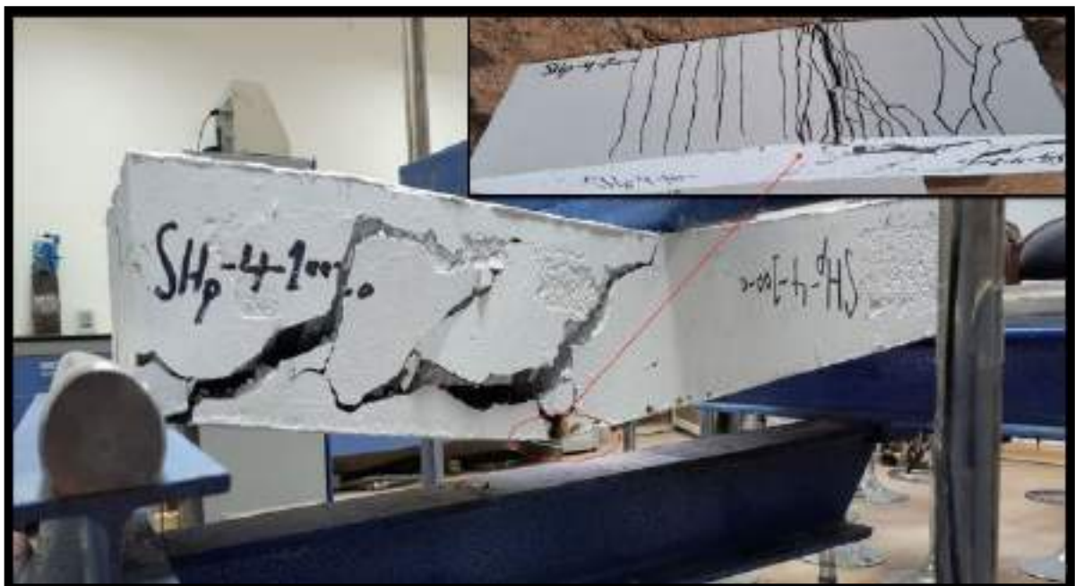
(f) Mode of failure for SHp-4-100-0 specimen.
