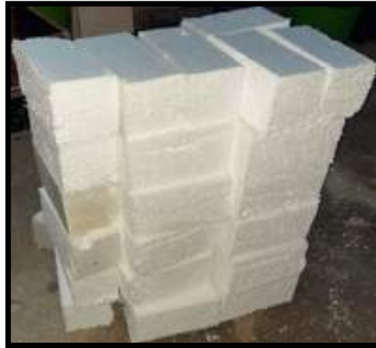
Figure. 3-6: Styropor prism of (200 ×100 ×100)mm.
