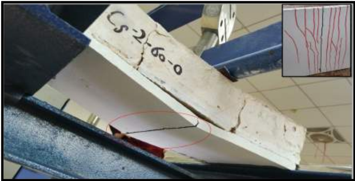
(a) Mode of failure for Cs-2-60-0 specimen.
