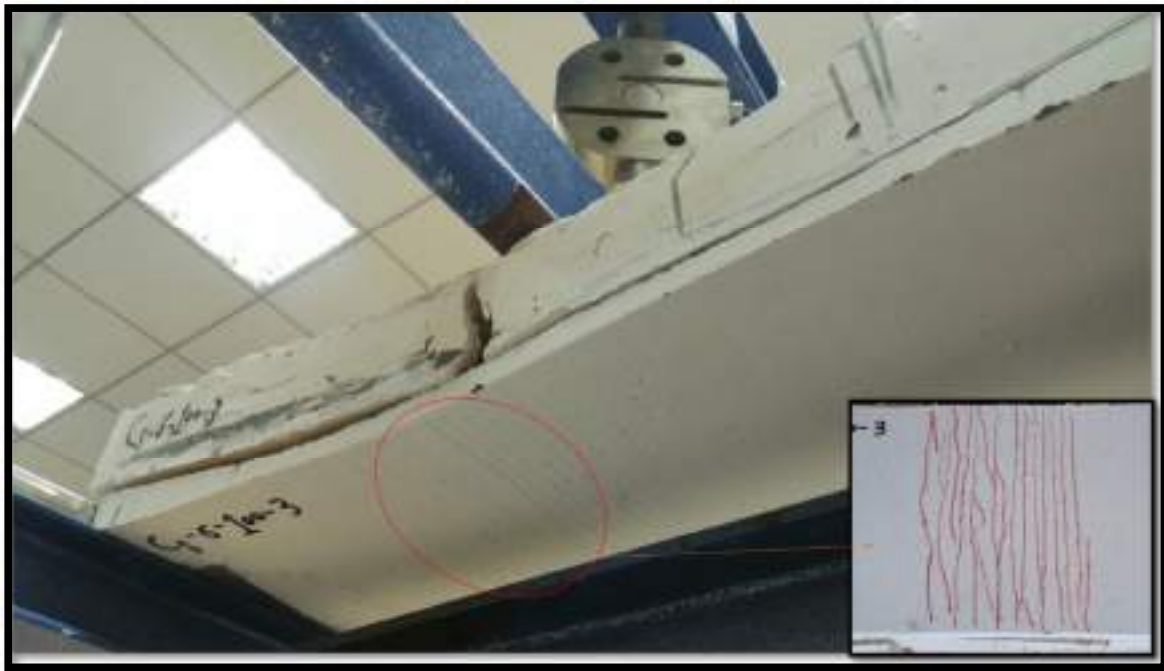
(g) Mode of failure for Cs-6-100-3 specimen.
