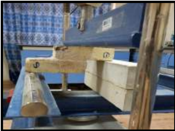
(a) Test set up of solid brick before failure.
