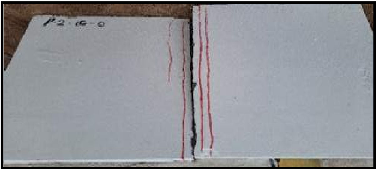
(a) Mode of failure for P-2-60-0 specimen.
