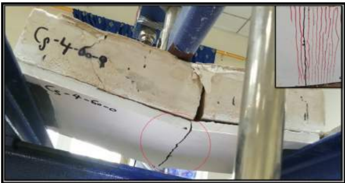
(b) Mode of failure for Cs-4-60-0 specimen.
