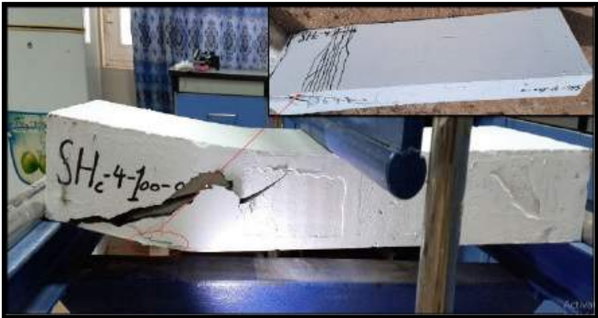
(e) Mode of failure for SHc-4-100-0 specimen.
