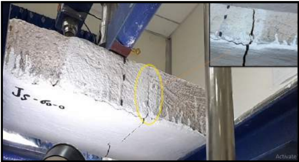
(a) Mode of failure for Js-60-0 specimen.
