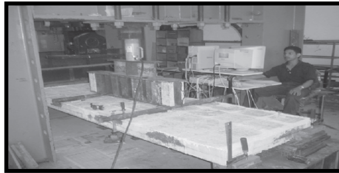
Figure. 2-21: Flexural two-line load Test setup of slabs [29].
