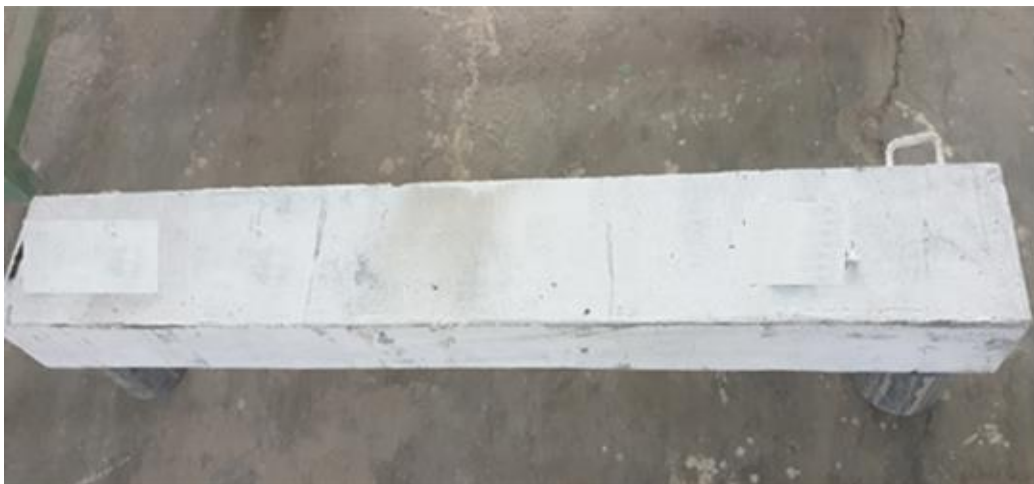
Figure 3.17 Painting the specimens by white color.
