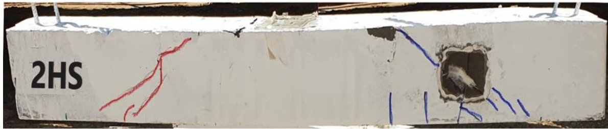
Figure 4.23 Diagonal shear failure for beam 2HS.
