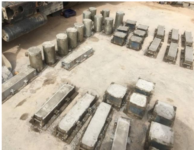
Figure 3.4 Specimens of hard concrete tests (cubes, cylinders and prism)
