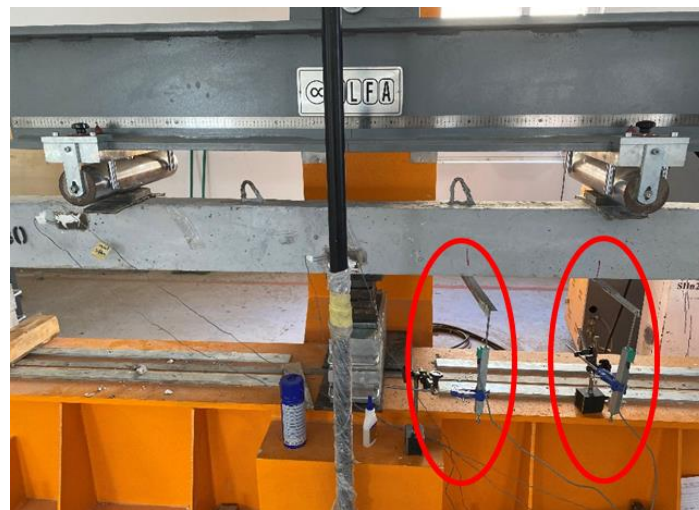
Figure 3.12 LVDT position on the beam
