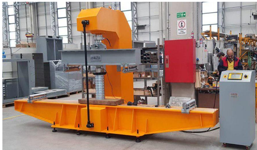
Figure 3.9 Flexural testing machine
