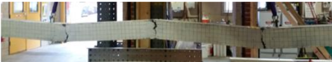
Figure 2.3 Typical beam after failure [23]
