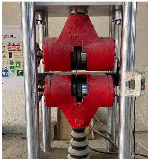
Figure 3.3 Tensile strength of reinforcement test bars
