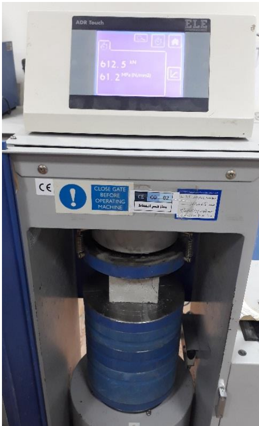
Figure 3.5 Compressive strength test
