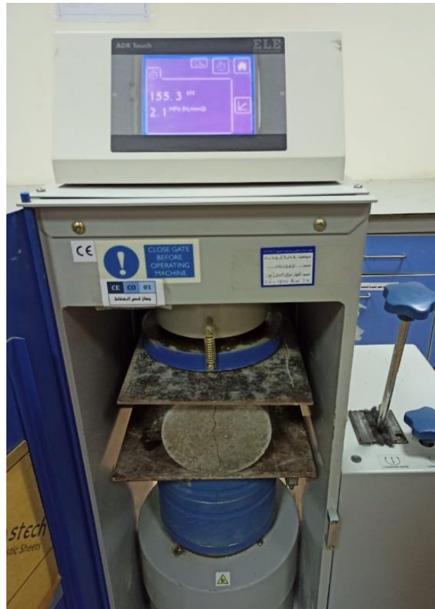
Figure 3.6 Split tensile strength test
