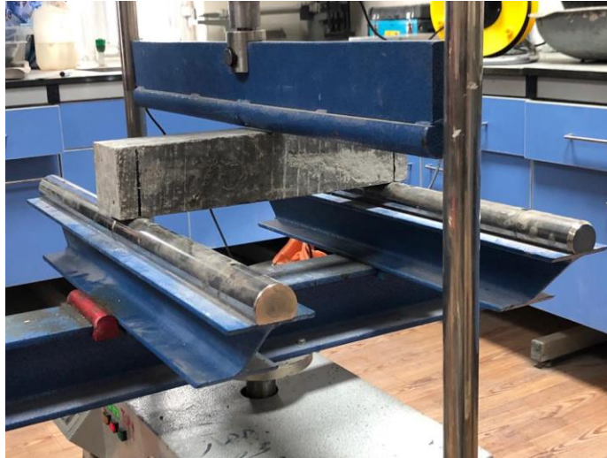
Figure 3.7 Flexural strength test
