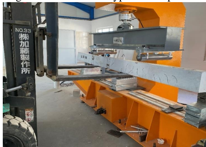
Figure 3.14 Flexural test of specimens
