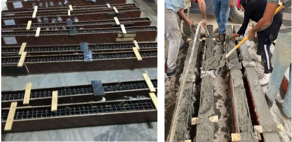
Figure 3.8 Preparing and casting procedure of the specimens
