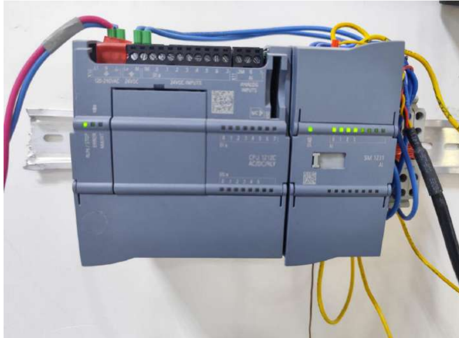
Figure 2-13 The Programmable Logic Controller (PLC) and the extension it provides
