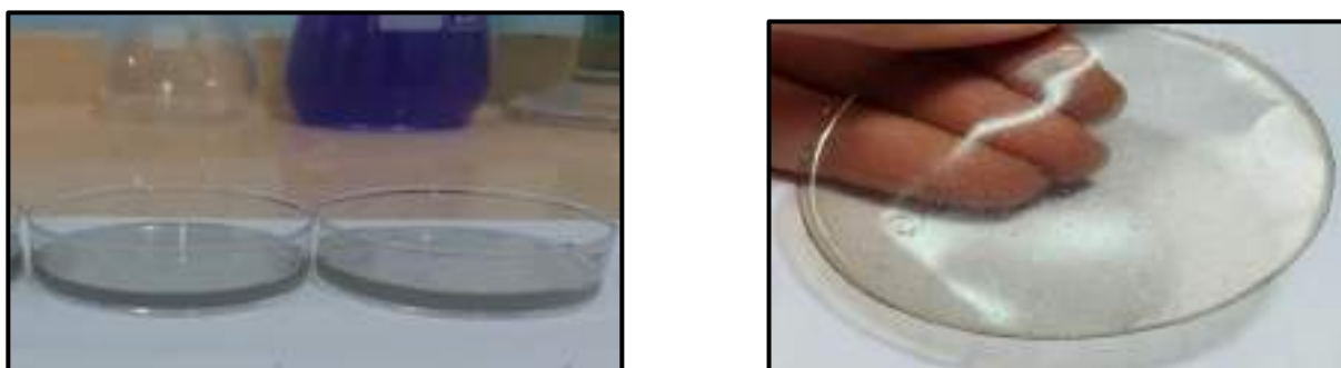
Fig. (2-6): (A) NGO-CS solution poured into a plastic Petri dish (B) the NGO-CS film after dry
