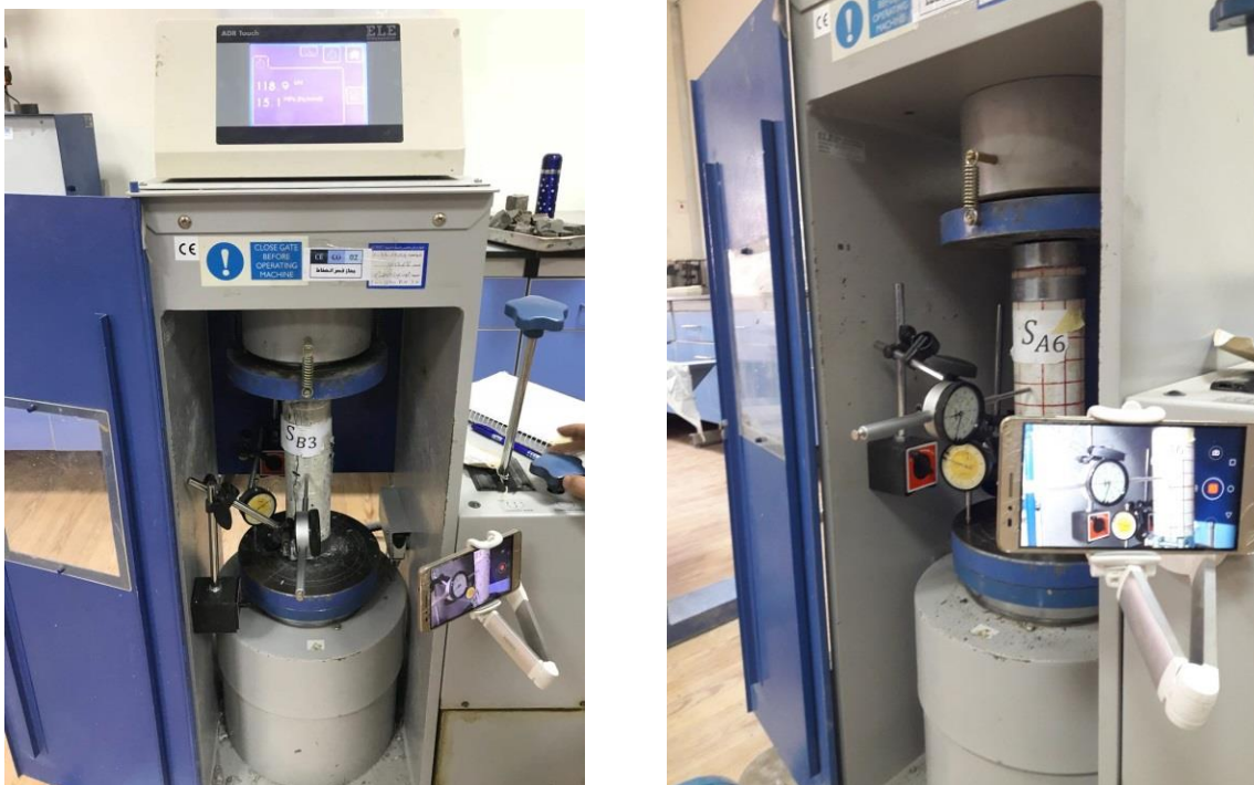
Plate (3.13). Short Column testing
