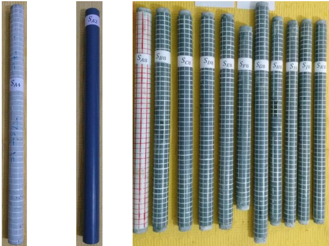
a-Concrete column b- PVC column c- Slender confined columns
