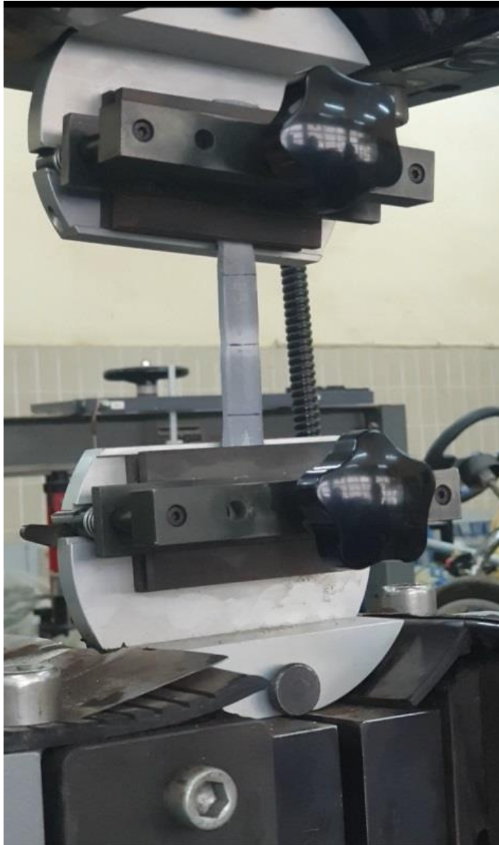
Plate (3.3) Coupon arrangement in testing machine.
