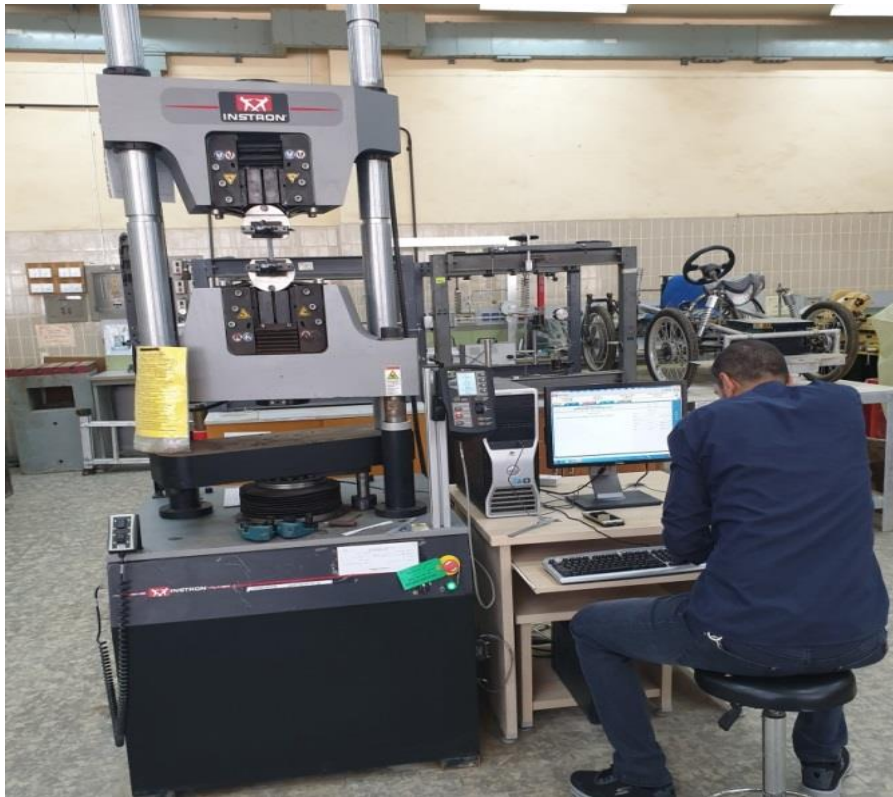
Plate (3.1) Tensile test machine for PVC coupons.
