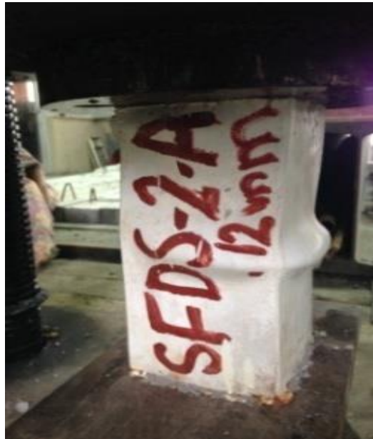
Plate (2.1) mode of failure
