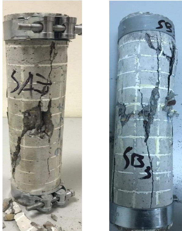
Plate (4.1) Typical failure modes of concrete short specimens SA3 and SB3
