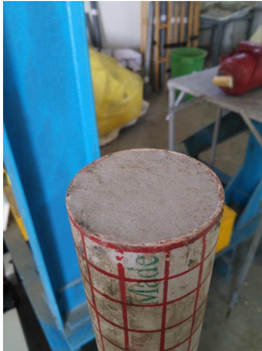
Plate (3.11). Column face after leveling.
