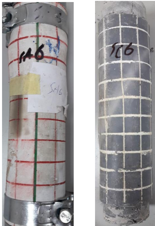
Plate (4.4) Typical failure modes of short confined specimens SA6 and SC6
