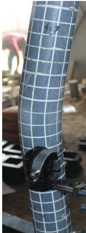
Plate (4.6) Typical failure mode of slender column SC7
