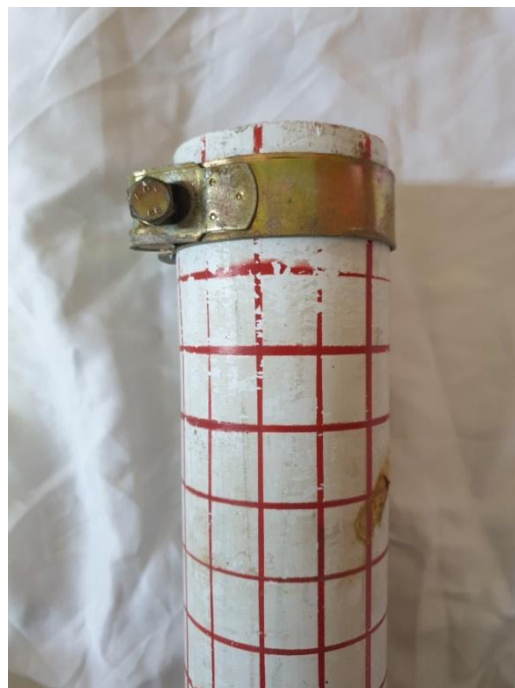
Plate (3.12) Column with steel ring strengthen
