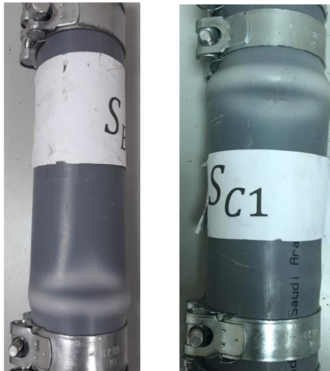
Plate (4.2) Typical failure modes of short plastic specimens SE1 and SC1
