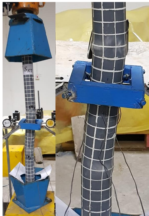
Plate (4.8) Typical failure modes of slender column SK7
